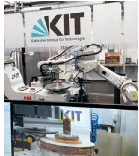
Fig. 5: Robotic winding of the MEESSST HTS-Magnets.
