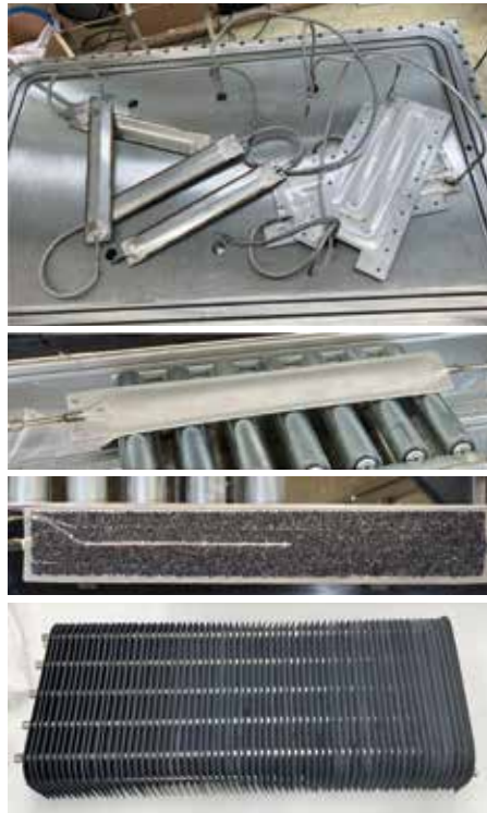
Fig. 1: Components of the JT-60SA Cryopumps.
