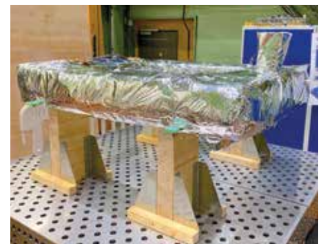
Fig. 3: Coil and current leads inserted into the cooling shield.
