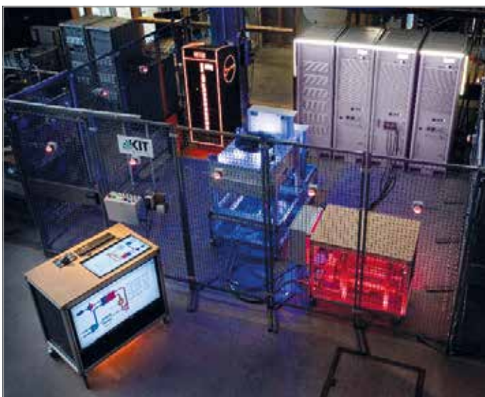
Fig. 10: Thermal-hardware-in-the-loop: (a) experimental setup, (b) mass flow control options.
