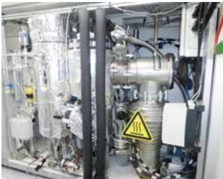
Fig. 8: NEMESIS experimental setup for characterising nozzle geometries for mercury diffusion pumps.
