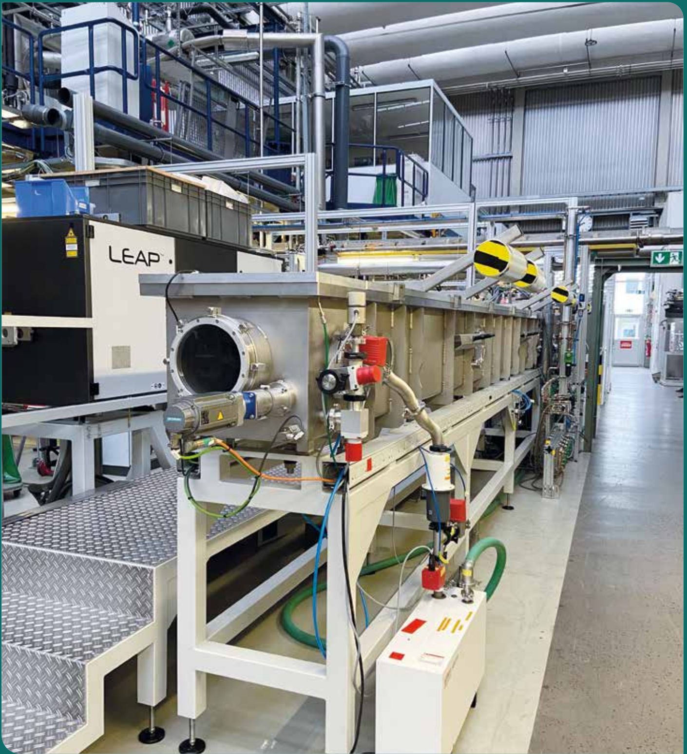
Set-up of the pulsed laser deposition cluster KC 4 – the KIT-CERN Cooperation on Coated Conductors
