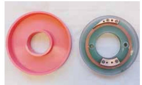
Fig. 1: Impregnated HTS Pancake-Winding (right) with impregnation mould.
