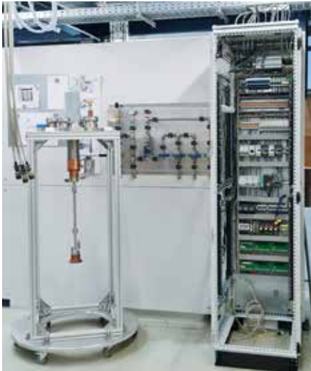
Fig. 2: Operation (left) and control cabinet (under construction, right) of the heat pipe test stand.
