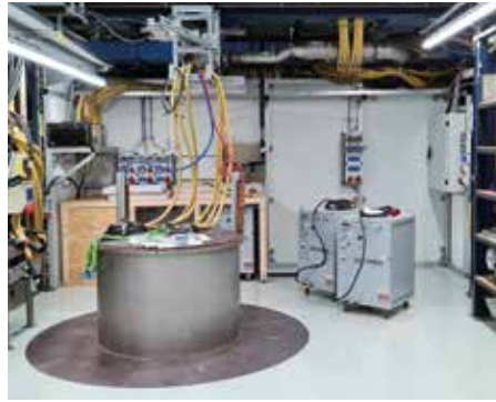
Fig. 3: State of construction of the 30 K test platform at the end of 2022.
