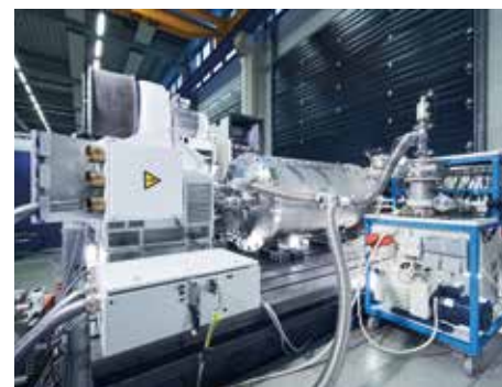
Fig. 2: Superconducting generator demonstrator on the engine test bench at Campus East.
