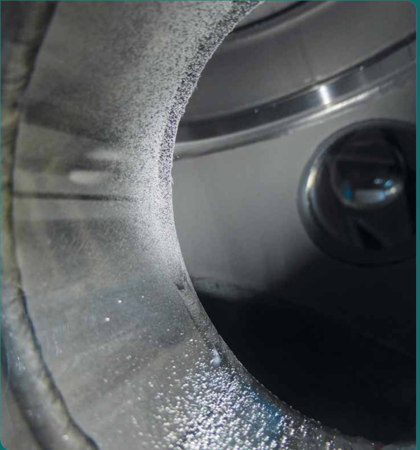
Retained mercury dew during active experimental operation with the NEMESIS setup in the HgLab Karlsruhe.
