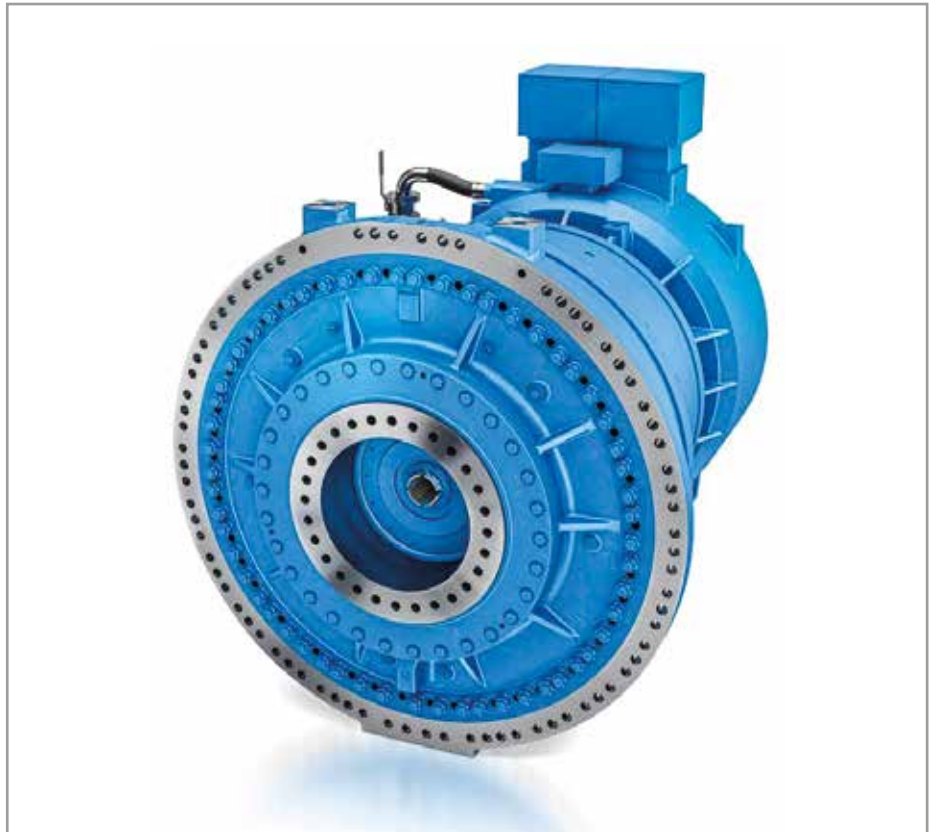
Illustration: Drive side (gearbox side) of a medium-speed wind power generator with central feed-through for the blade adjustment (“pitch tube”) of the wind turbine. In the final product, this pitch tube must also be able to be passed through an HTS rotor - the invention allows this. The picture shows the housing of the conventional machine (Flender/Winergy).
