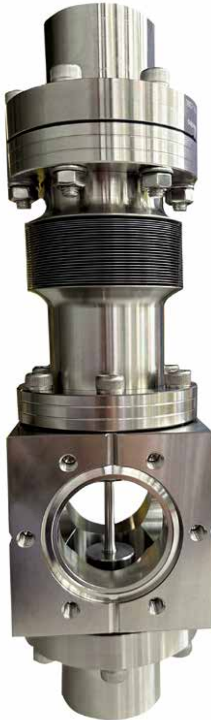
Test Chamber for mechanical tensile or fracture tests in cryogen hydrogen (gaseous or liquid)
