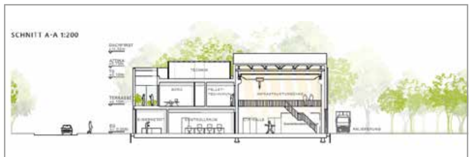
Fig. 9: Section through the DIPAK building; the workshop area is on the left, the test hall on the right.
