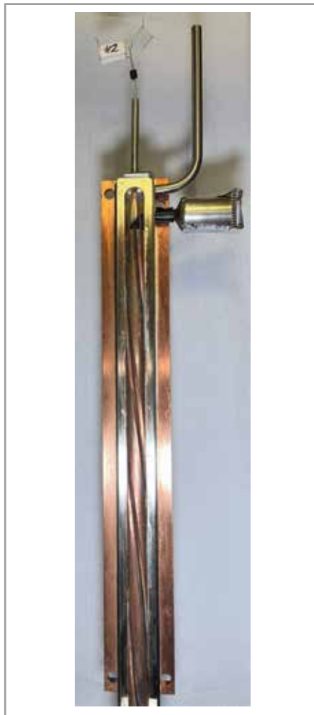
Fig. 9: Photo of the state of repair at the end of 2024. The wires (above) will have to be removed and replaced with glass fibers. The wires were used to prevent contamination of the capillaries.
