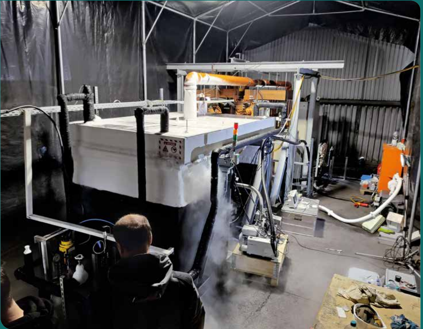
Installation of a technology demonstrator for a superconducting 200kA industrial busbar being at Trimet in Voerde
