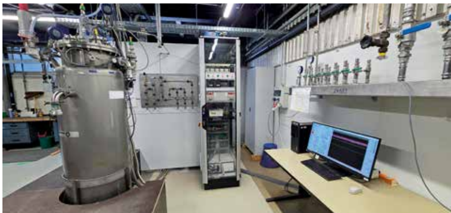
Fig. 2: Thermosiphon test stand with cryostat and cryocooler (left), measuring rack (center) and PC with LabView measuring program (right).
