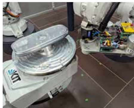
Fig. 1: Test winding of a coil with erected winding heads on a superellipse-shaped winding body.
