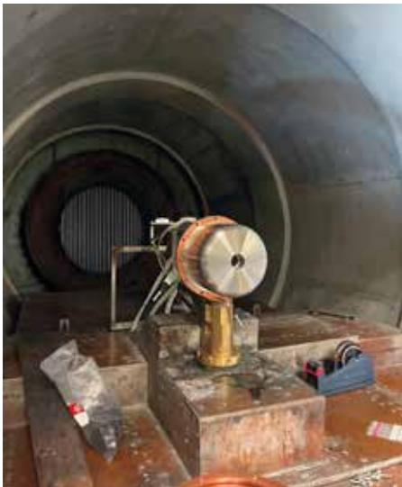
Fig.5: MEESSST magnet and cryostat during installation in the PWK1 plasma channel of the IRS.
