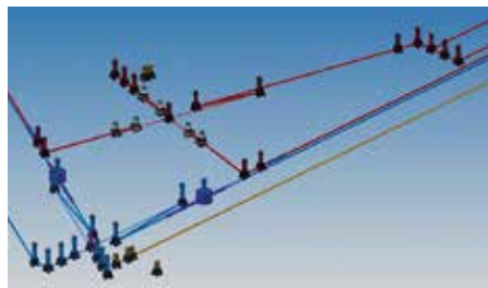
Fig. 5: Corner of the ET triangular interferometer with cryopumps already integrated in the detector layout (beam tubes with blue thickened sections).
