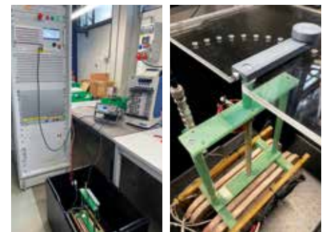
Fig. 16: Setup for angle-dependent AC magnetization measurement on DUDA coils.
