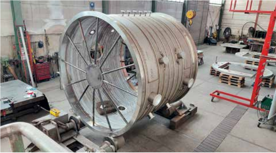
Fig. 10: Image from the production of the centre section of the central vacuum vessel.
