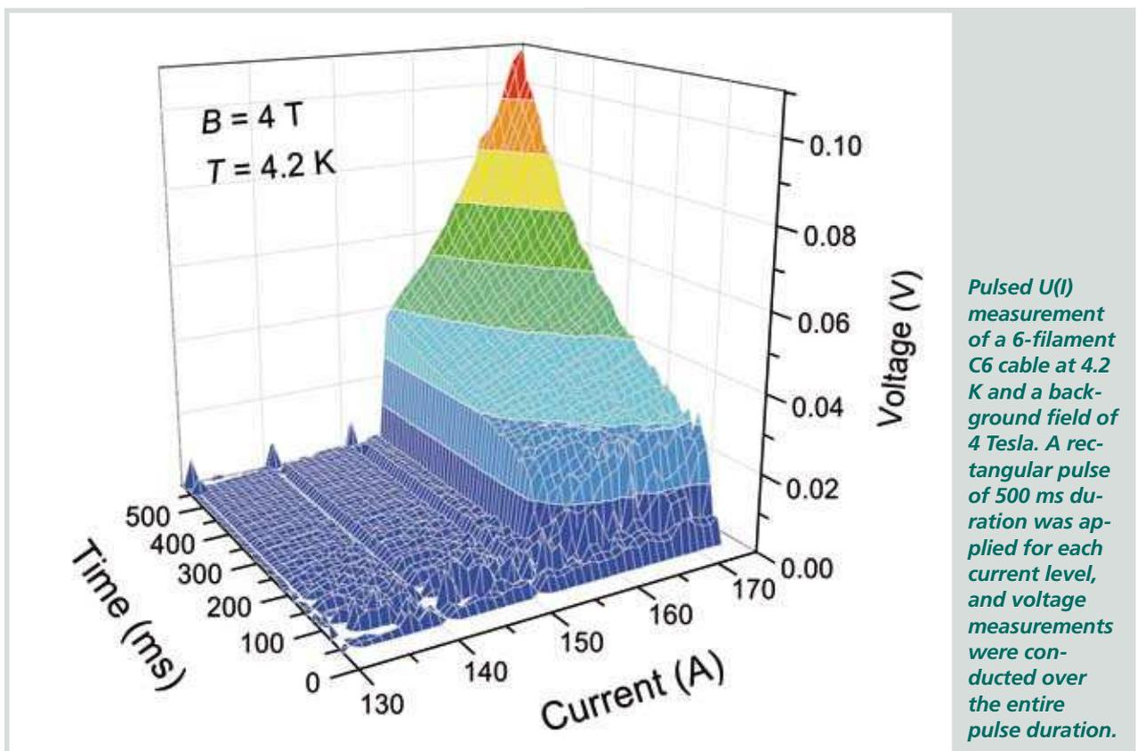
**Pulsed  $U(I)$  measurement of a 6-filament C6 cable at 4.2 K and a background field of 4 Tesla. A rectangular pulse of 500 ms duration was applied for each current level, and voltage measurements were conducted over the entire pulse duration.**
