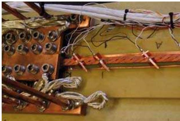
*Cable section and area of current application in the Roebel cable shown in Fig. 1.*
