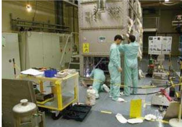
**Fig. 7: Installation of parts of the tritium loop into the ISS glovebox of the TLK.**
