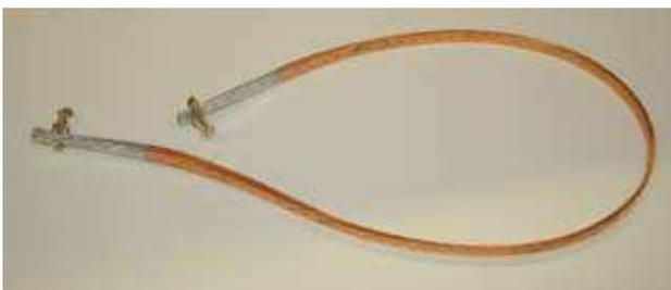
*Roebel cable 1.1 m long with a transport current of 2.6 kA at 77 K.*
