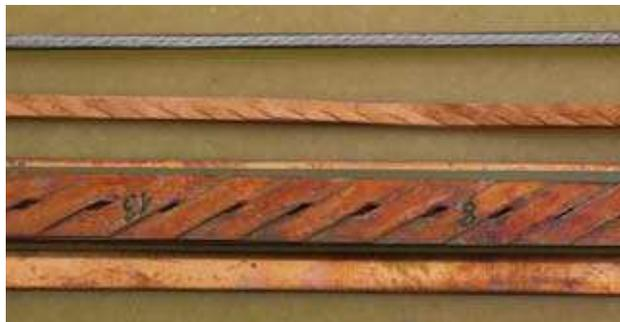
*Reduction of Roebel cable width from 12 mm (bottom) to 4 mm (center), and steel strip experiments for structures 2 mm wide (top).*
