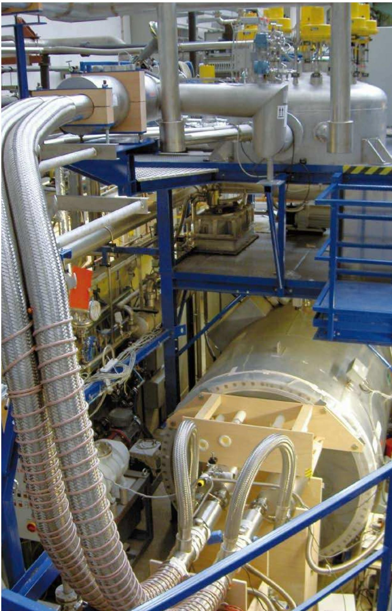
*Fig. 2: The new cryotransfer line of the ITER prototype is commissioned in TIMO-2.*
