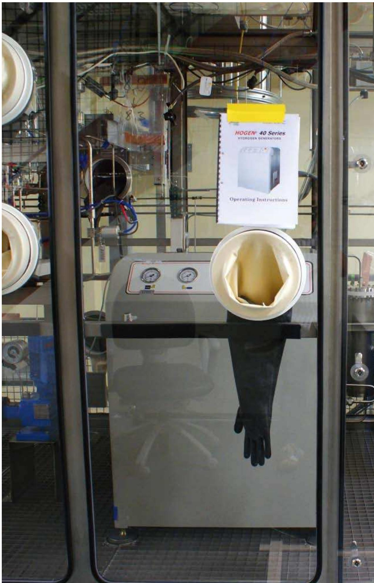
Fig. 3: Electrolysis units in the caisson.
