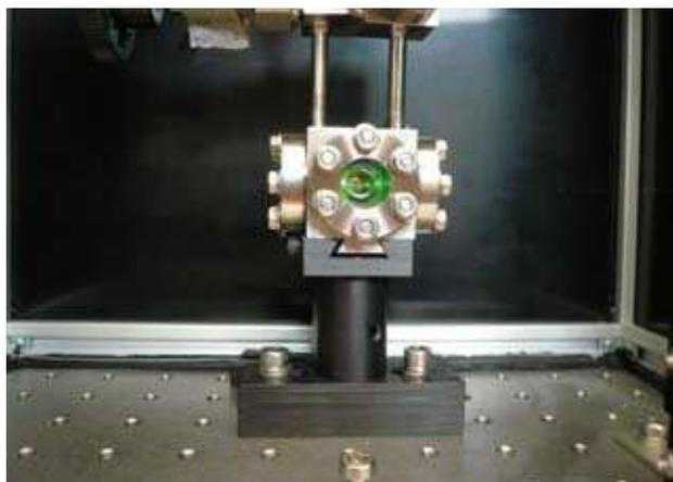
**Fig. 8: Laser Raman cell. The laser beam (green) is visible when passing through the gas-filled cell.**
