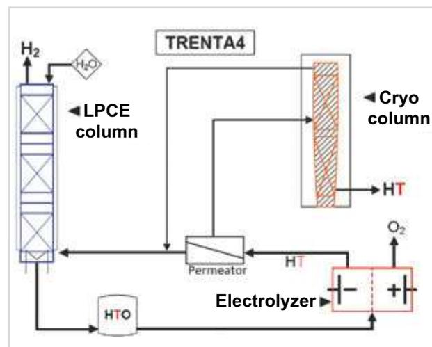
Fig. 5: TRENTA4: WDS + Cryo distillation.
