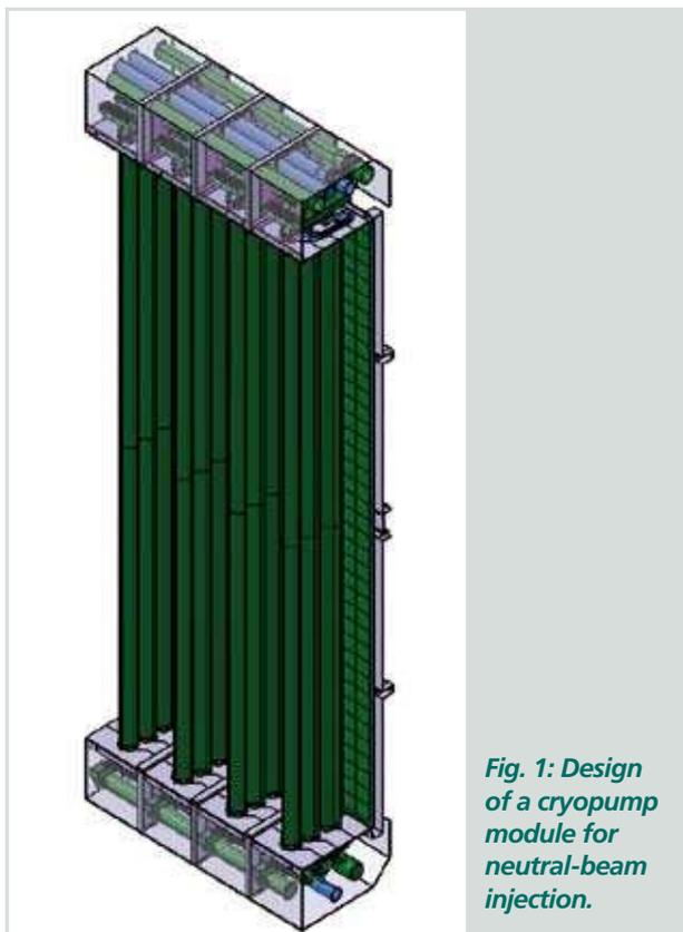
*Fig. 1: Design of a cryopump module for neutral-beam injection.*
