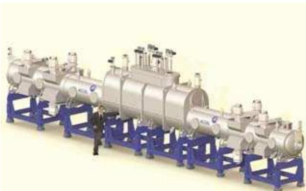
**Fig. 2: WGTS magnet cryostat. The technical requirements to be met by the 16 m long cryostat are challenging, and its technical design is extremely complex. The system has twelve cryogenic loops and uses six different fluids (He, Ne, N<sub>2</sub>, Ar, T<sub>2</sub>, and Kr).**
