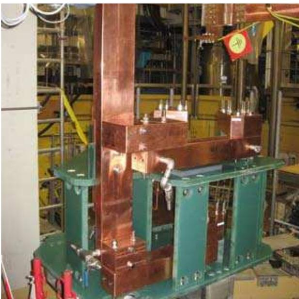
*High-current current leads allowing three coils to be fed current individually up to 18.2 kA.*
