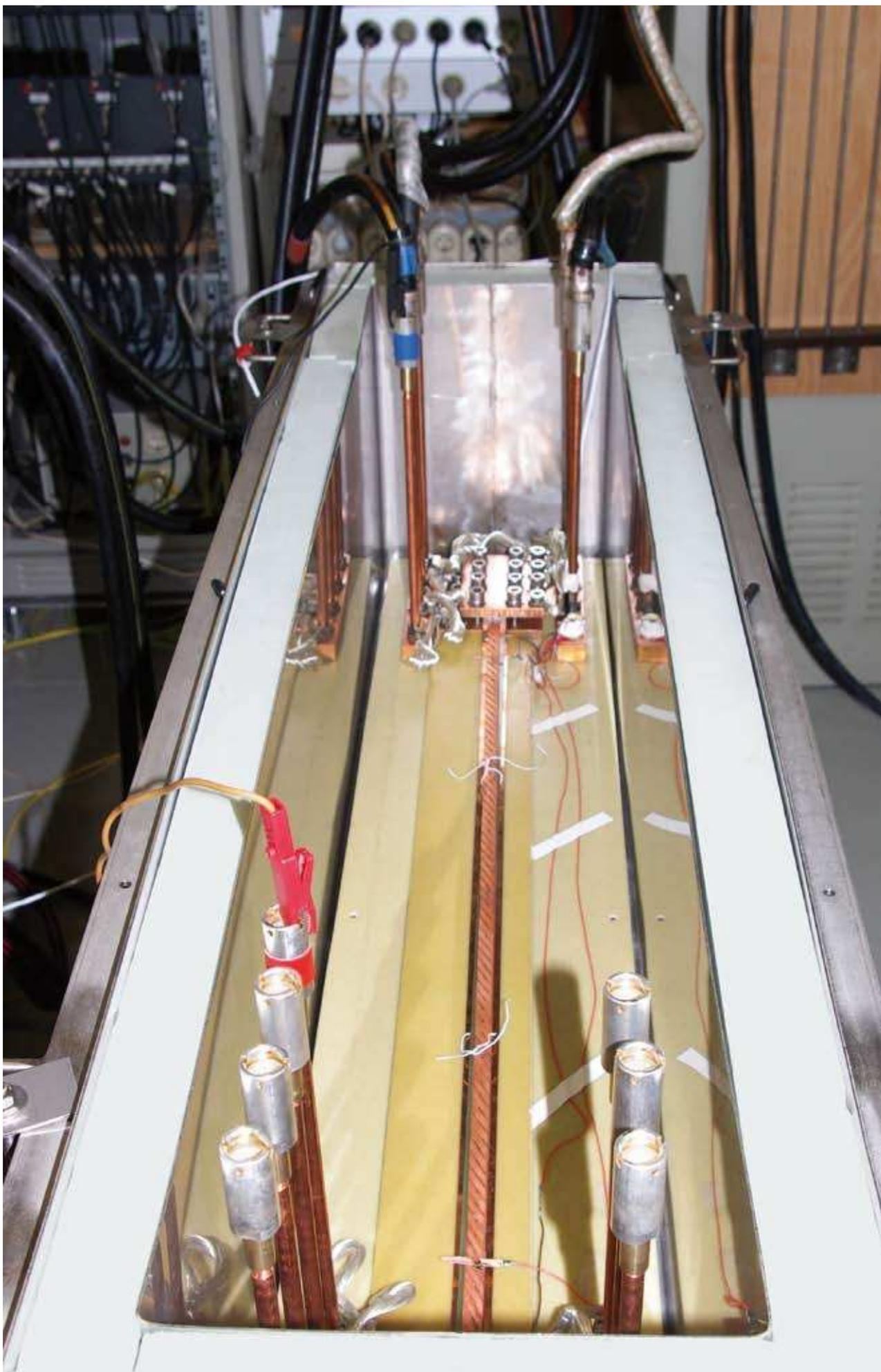
*A 2.6 kA Roebel cable in the LN<sub>2</sub> test cryostat with a transport current feed system split sevenfold.*
