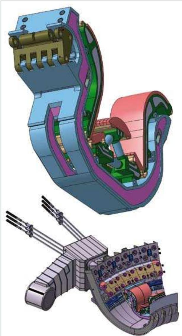
*Fig. 4: 3D design of a divertor cassette and its position in the vacuum vessel of ITER.*
