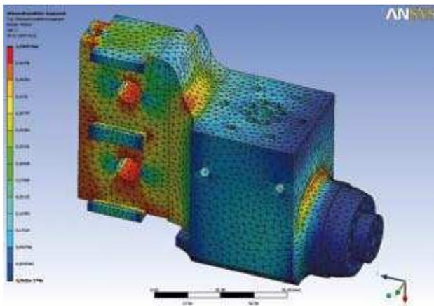
**Fig. 2: FEM analysis of the RT current lead head.**
