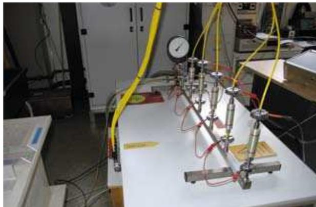
**Fig. 3: High voltage test station for insulation breaks.**
