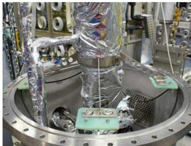
Fig. 4: Top of the cryo column in the cold box.
