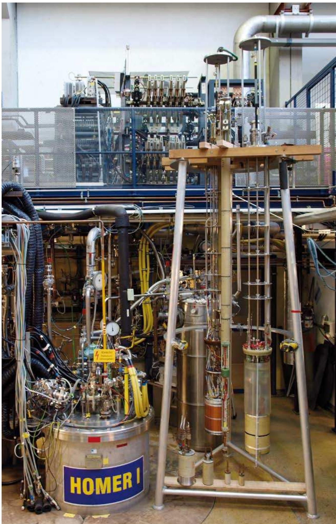
*HOMER I 25 years: background magnet system plus variable high field insert coils.*
