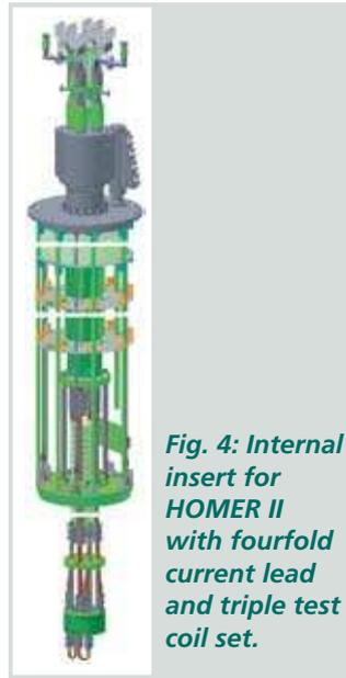
*Fig. 4: Internal insert for HOMER II with fourfold current lead and triple test coil set.*
