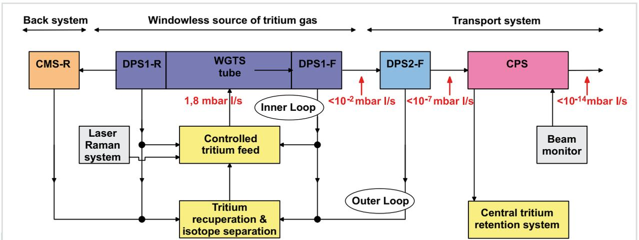
Fig. 3: Block diagram of the KATRIN tritium source and its interfaces with the infrastructure of the Karlsruhe Tritium Laboratory.
