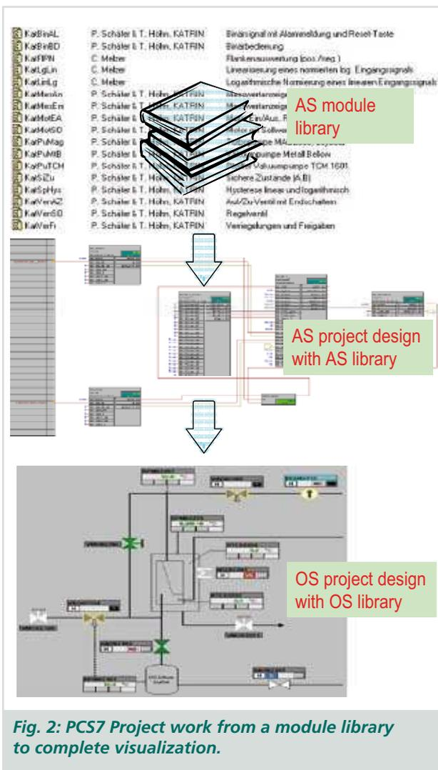
Fig. 2: PCS7 Project work from a module library to complete visualization.
