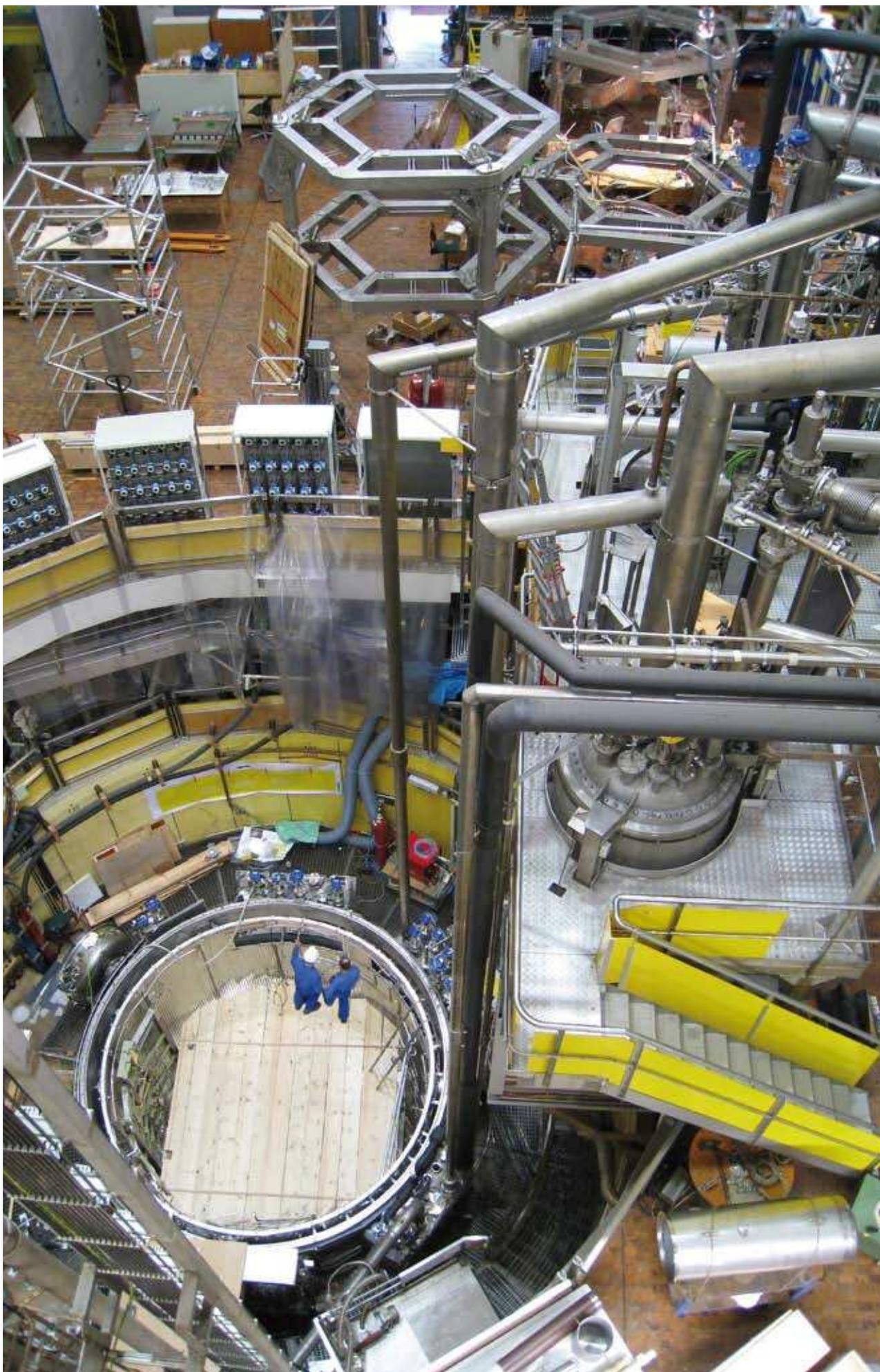
*TOSKA: preparation for the W7-X coil tests.*
