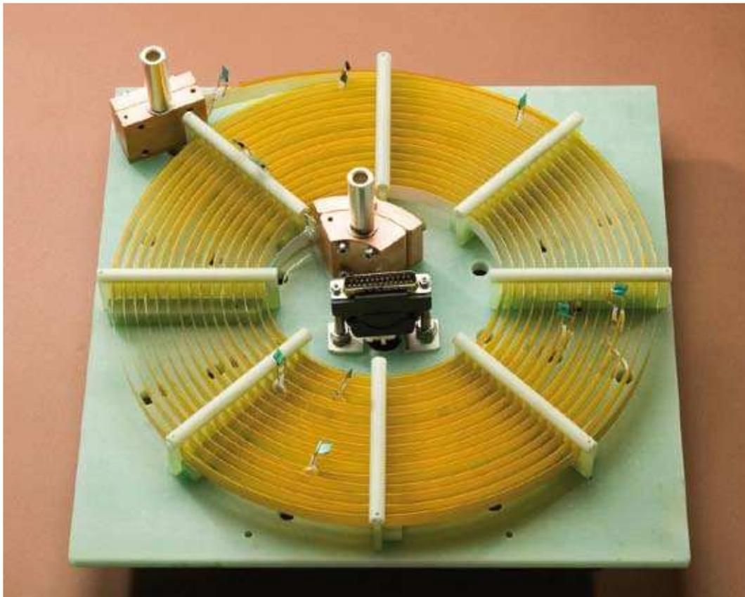
*Superconducting current-limiting module made out of an YBCO strip conductor.*
