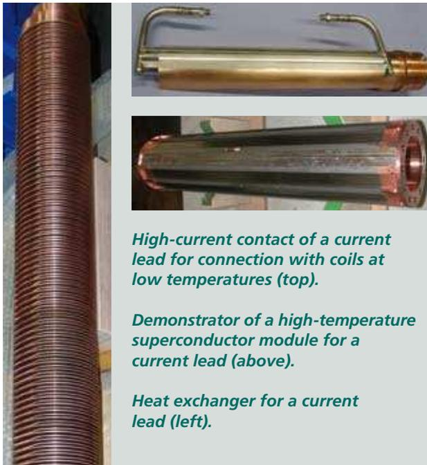
*High-current contact of a current lead for connection with coils at low temperatures (top).*
