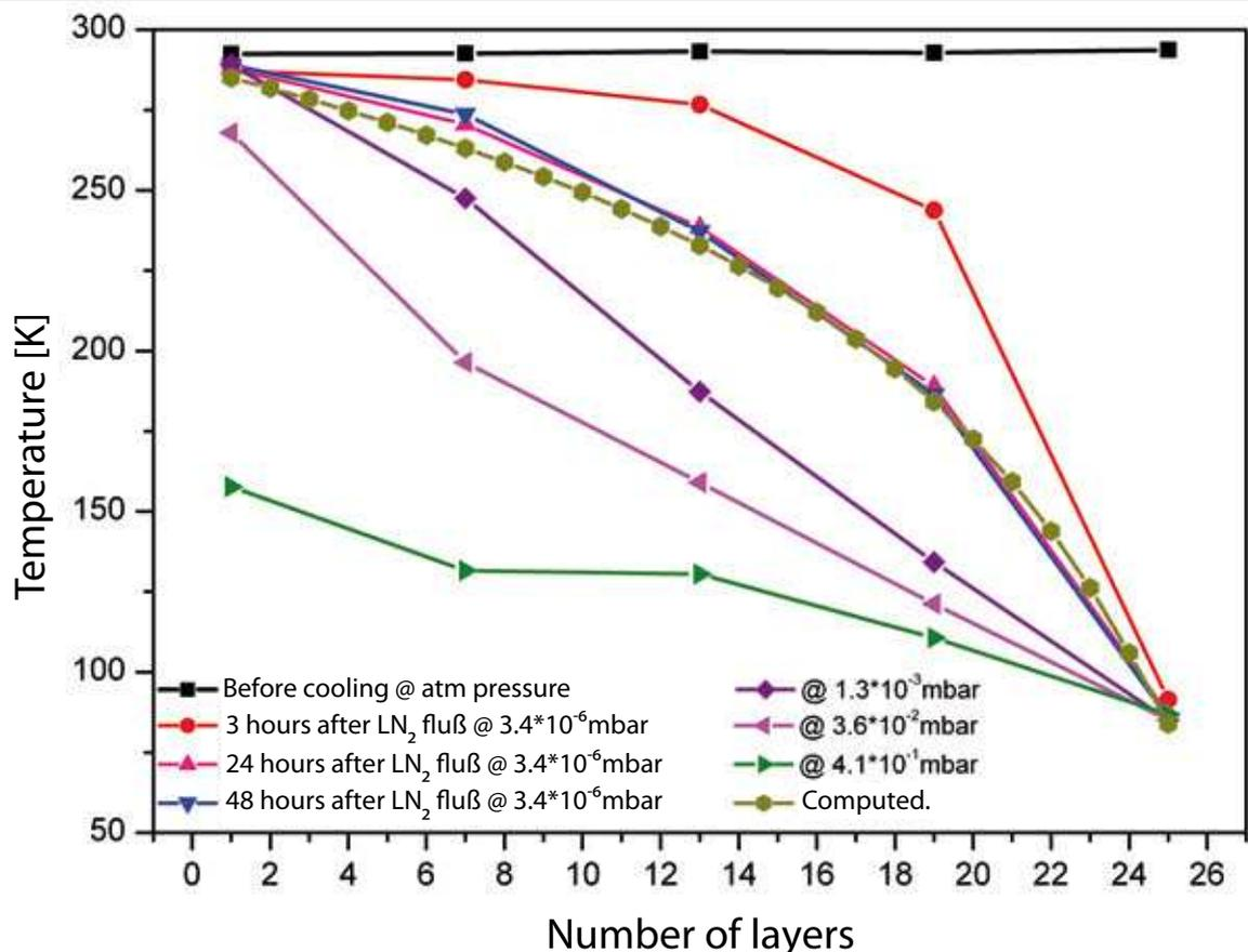
Measured and computed layer temperatures in a superinsulation stack.
