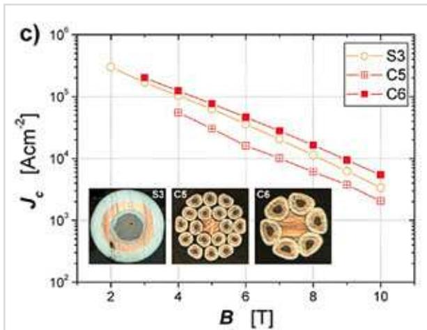
**Field dependence of current densities of a single  $MgB_2$  strand (S3) with a composite sheath of Nb/Cu/stainless steel, and of cables prepared from 6 and 18 of these strands.**
