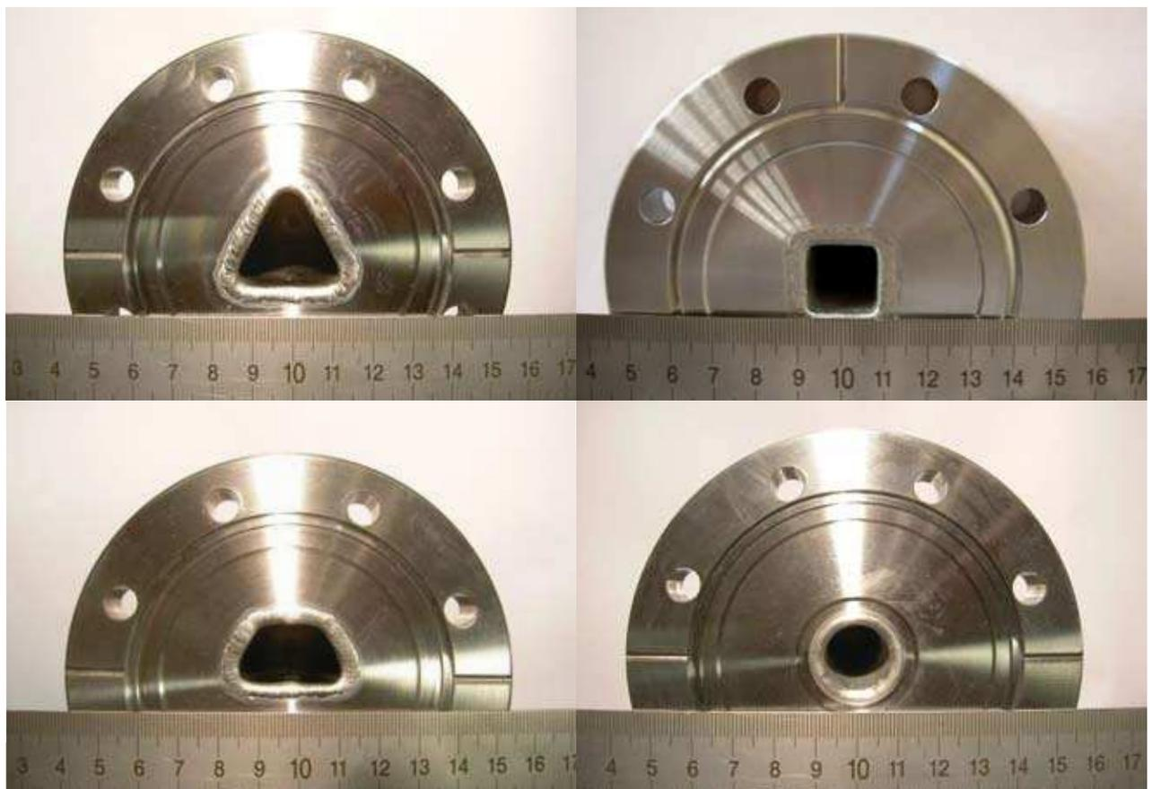
Fig. 3: Channel profiles measured in TRANSFLOW.
