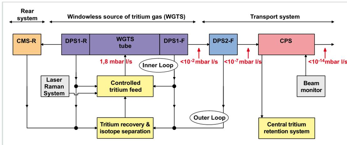
Fig. 4: Block diagram of the KATRIN tritium source and its interfaces with the TLK infrastructure.
