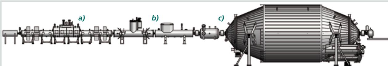
**Fig. 2:** Schematic diagram of the KATRIN international large-scale experiment. The electrons produced in  $\beta$ -decays in a high-intensity windowless molecular tritium source (WGTS, (a)) are passed through a tritium pumping section containing DPS2-F and CPS as active and passive elements (b) to a system (c) made up of two electrostatic spectrometers (pre-spectrometer and main spectrometer). The electrons analyzed are detected in a solid-state detector (d).
