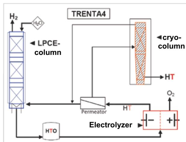
**Fig. 5: TRENTA4 - WDS and cryo distillation.**
