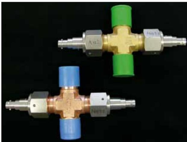
*Fig. 6: Cross-shaped I-clamps electroplated with gold and aluminium, respectively.*
