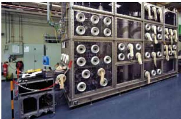
*Fig. 7: ISS glove box with the LARA system connected. The newly erected part of the tritium loop is contained in the left section of the box.*
