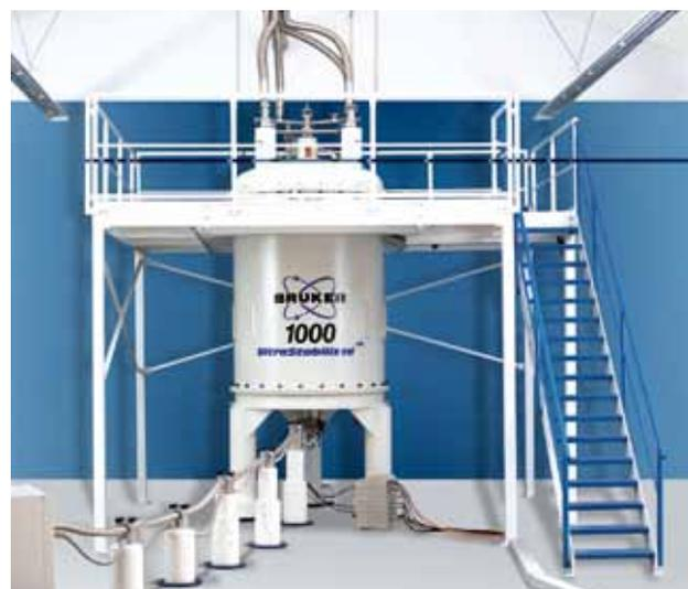
Fig. 6: The world's first 1000-MHz NMR spectrometer with a field strength of 23.5 T (see [www.bruker.biospin.com/pr090601.html](http://www.bruker.biospin.com/pr090601.html)).
