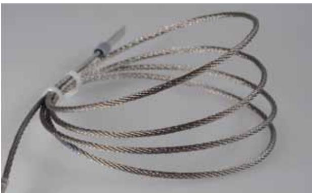
**Fig. 5:**  $\text{MgB}_2$  cable with thin strands.
