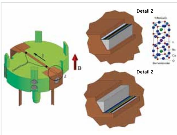
Fig. 1: Test set-up to determine the anisotropic physics properties of high-temperature superconductors with the magnet field positioned normal to the broad side of the strip conductor.
