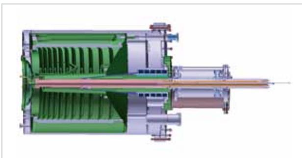
**Fig. 1:** 3D CAD model of the prototype torus cryopump. The inlet valve (left) has a diameter of 800 mm.
