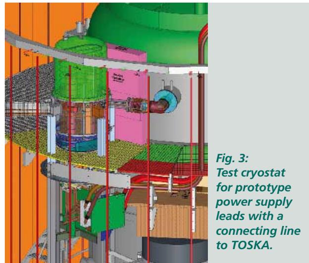
*Fig. 3: Test cryostat for prototype power supply leads with a connecting line to TOSKA.*
