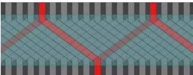
Fig. 2: CAD drawing of the superimposed laser structure of two superconducting YBCO layers and the transport current path produced.
