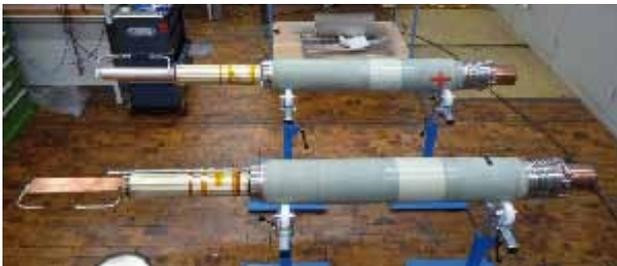
*Fig. 2: Prototype power supply leads after soft soldering of the heat exchanger, HTS module, and cold contact.*
