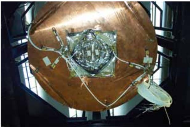
**Fig. 5:** THISTA lower cooling shield with connections for test objects and sensors.
