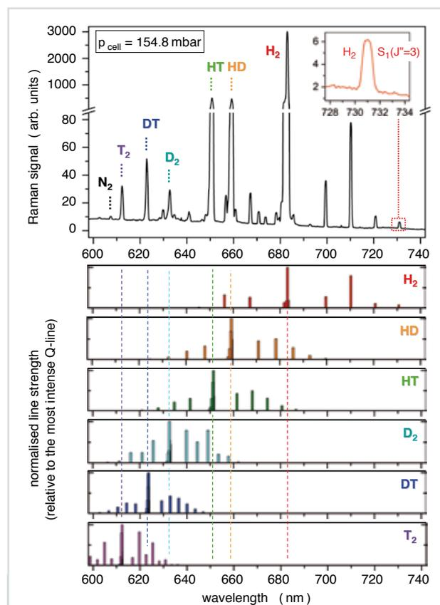
**Fig. 9: Raman spectra of an equilibrated mixture of hydrogen isotopologs (measurement time 1000 s). The Q1-lines of all isotopologs are marked. Bottom: model spectra, Q1-line suppressed by a factor of 20 (Sturm et al., Laser Physics 20 (2), 2010).**
