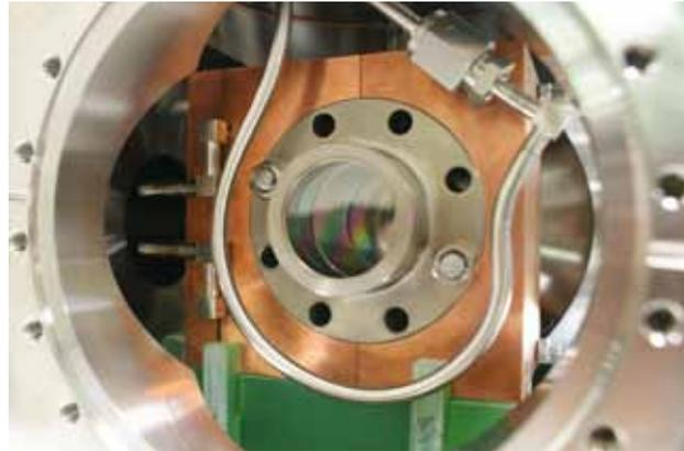
Fig. 8: IR measurement cell in the cooling structure.
