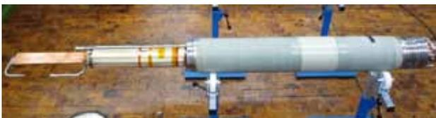
*Fig. 1: Prototype current lead showing assembly of the bus bar power connection (left), HTS module (center), and heat exchanger (right, with insulated vacuum space) components.*
