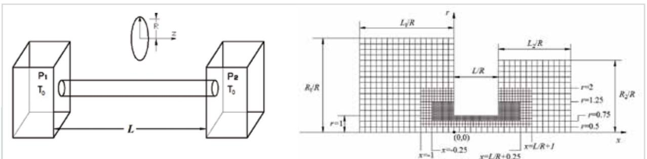
**Fig. 4: Modeling and meshing for numerical simulation of the vacuum flow through short pipes in the transition range.**
