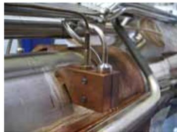
Fig. 5: Temperature sensors at beam tube (vapor pressure thermometer/Pt500).
