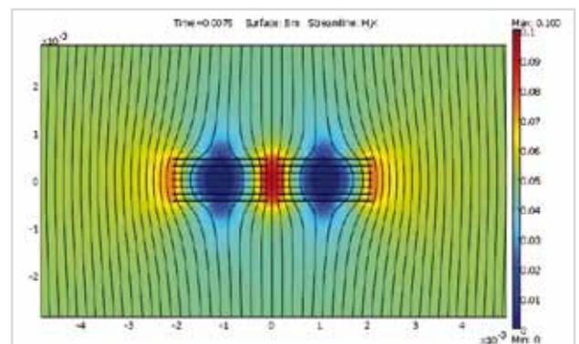
**Fig. 6:** Distribution of magnetic flux density in a Roebel cable with 14 conductors. The field amplitude is 50 mT, conductors are assumed to be isolated.
