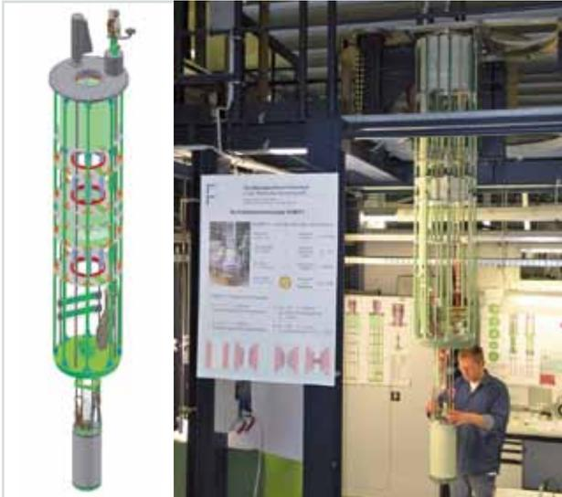
**Fig. 3: Magnet flange accepting a 24-T  $(\text{NbX})_3\text{Sn}$  insert coil.**
