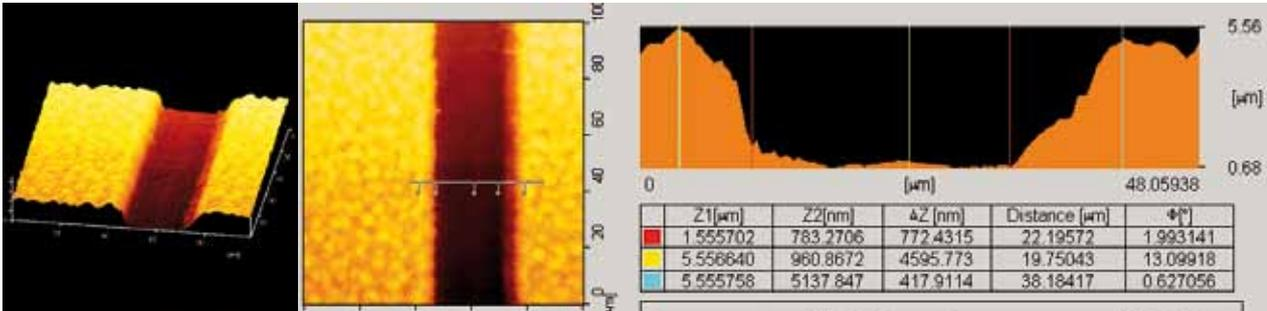
Fig. 1: AFM profilometer image of a laser-structured slit, and line scan for determining width (22.2 μm) and depth (4.6 μm).
