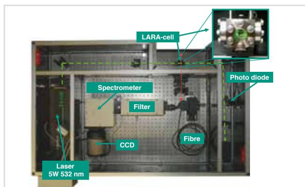
**Fig. 8: LARA system for KATRIN. This system was developed over several years in a joint effort with the University of Swansea, Wales.**
