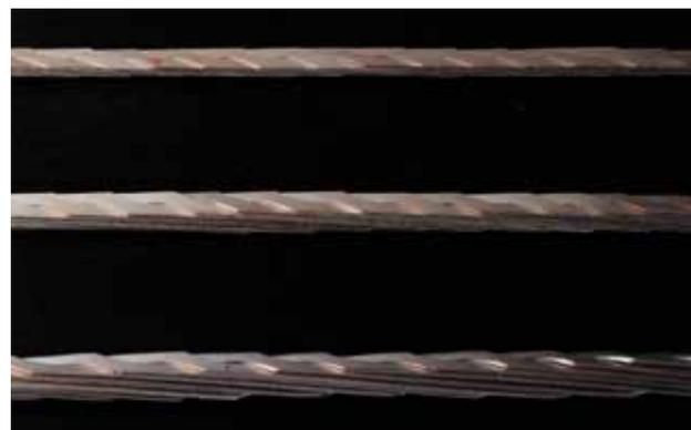
Fig. 3: Roebel cables with 14, 39, and 50 conductors (top down) and width of 4 mm.
