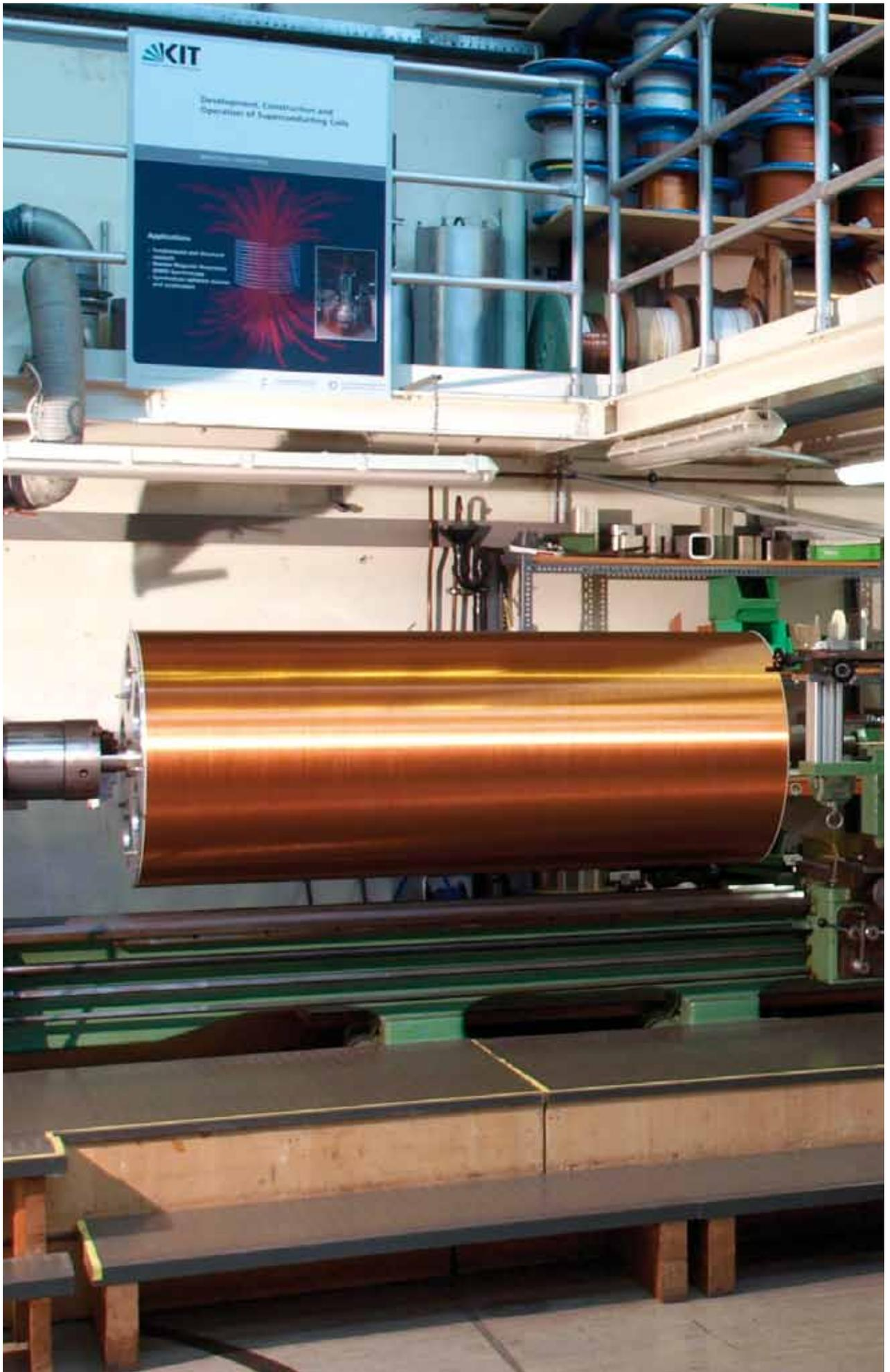
*Solenoid coil manufactured for the helium-3 polarizer of the university of Mainz.*
