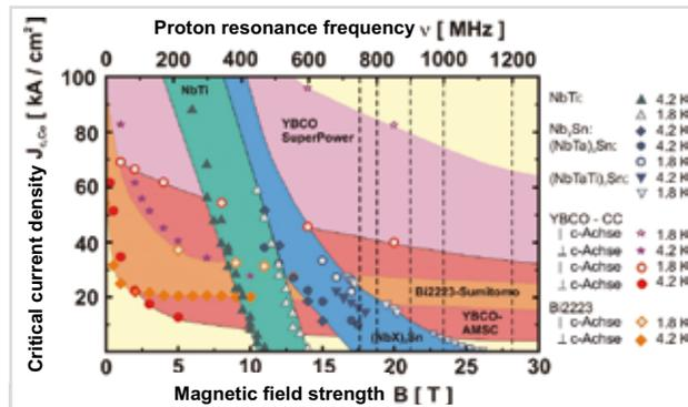
Fig. 2: The critical current density,  $J$ , plotted as a function of the external magnetic field,  $B$ , for commercial composite superconductors.
