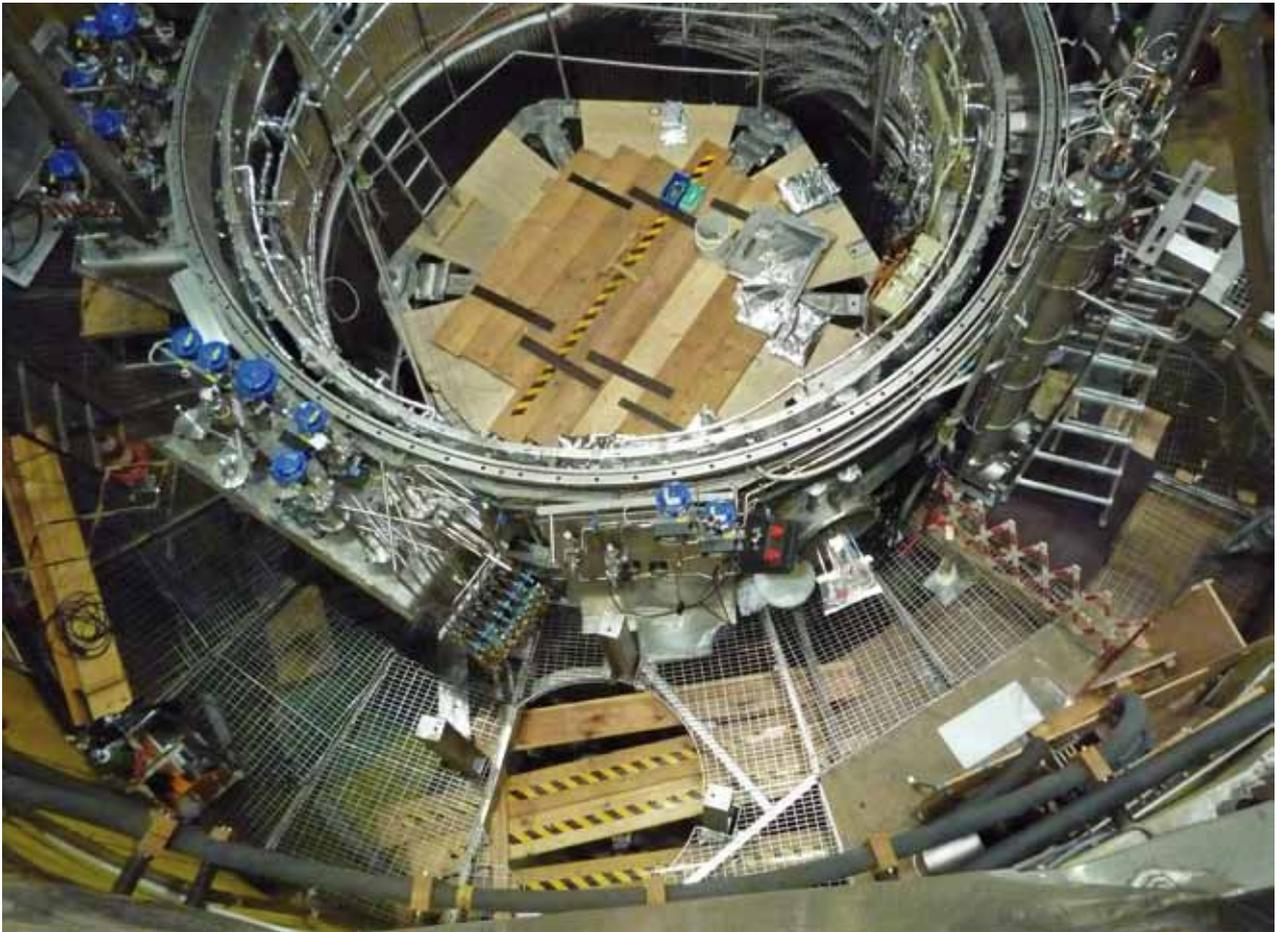
*Fig. 2: TOSKA during adaptation for the prototype test of the W7-X current lead.*
