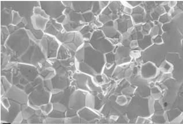
**Fig. 4:** Electron micrograph of the grain structure of a solid  $\text{Nb}_3\text{Sn}$  specimen. Grain sizes are around 0.01 mm in diameter.
