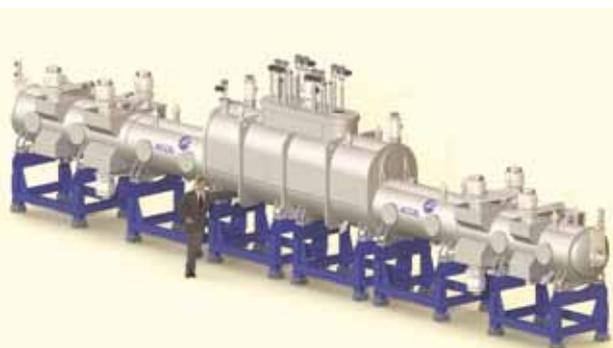
**Fig. 3:** WGTS magnet cryostat. The technical requirements to be met by the  $16 \text{ m}$  long cryostat are ambitious, and its technical structure is extremely complex. The system has twelve cryogenic loops; six different fluids (He, Ne,  $N_2$ , Ar,  $T_2$  and Kr) are used.
