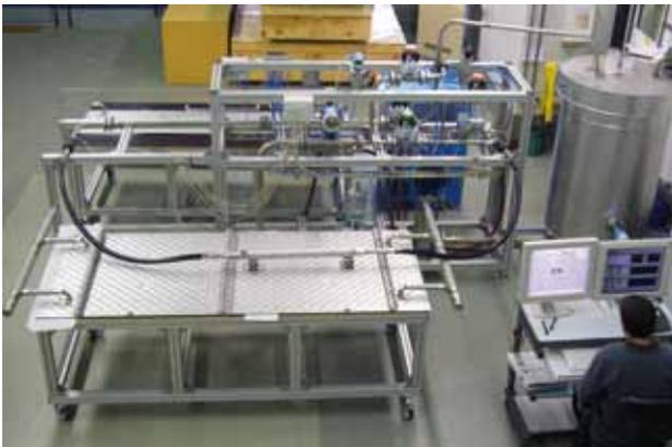
**Fig. 3: Measuring pressure losses in complex components over a broad range of Reynolds numbers in the THEA facility.**
