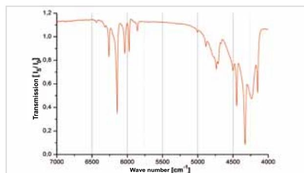
Fig. 9: Transmission spectrum of  $H_2$  in  $D_2$ .
