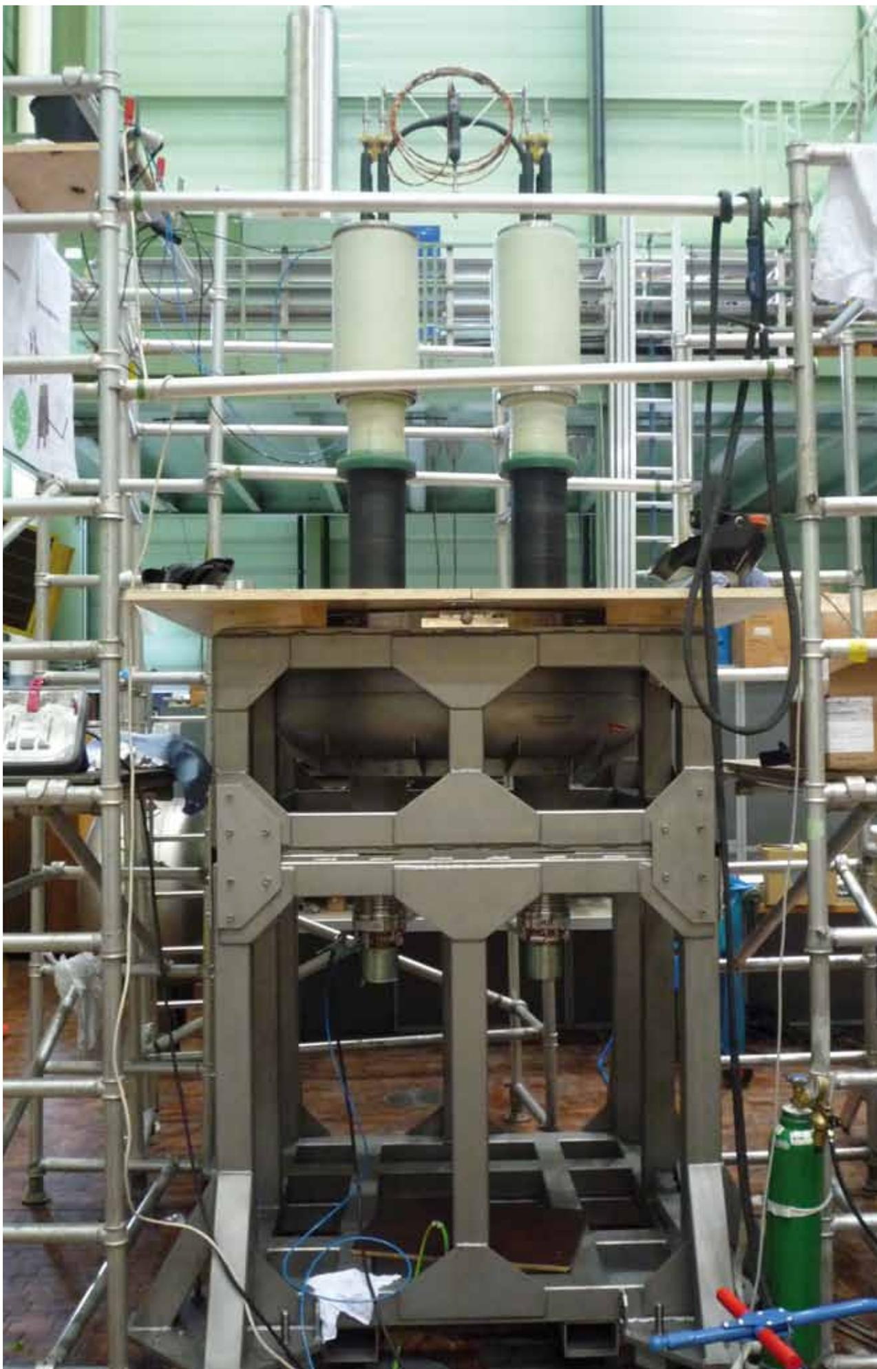
*Two high-current supply leads under preparation for the power test.*
