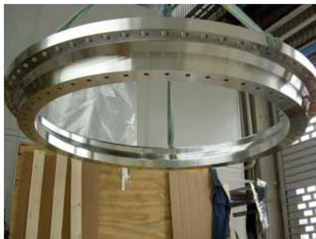
**Fig. 2:** The adapter flange (diameter 2 m), the first component for the new tests in TIMO-2.
