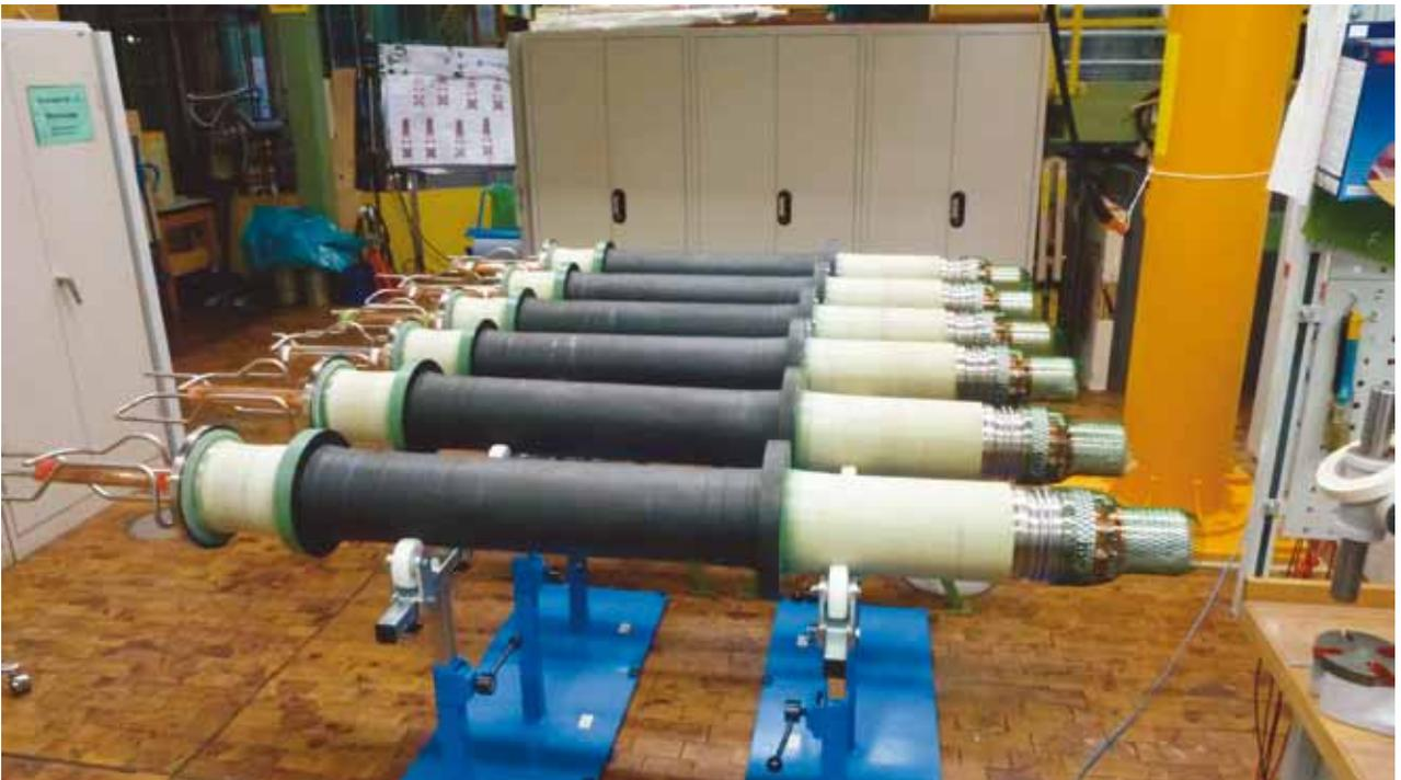
*Fig. 7: Series production of the current leads for W7-X.*
