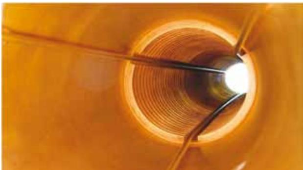
**Fig. 5:** Gold coating of beam tube section #3. The three capillaries for argon injection are mounted inside the beam tube.
