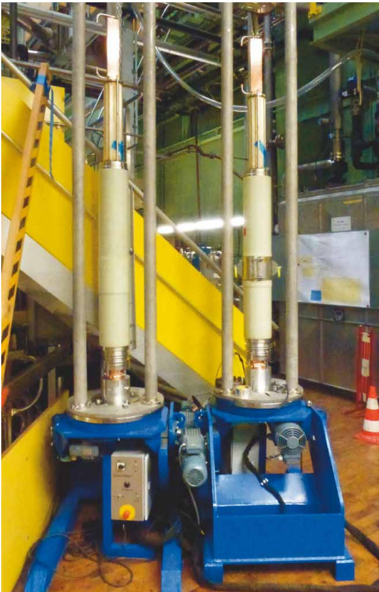
*Current leads for W7-X, prepared for soft soldering of the cold contact.*
