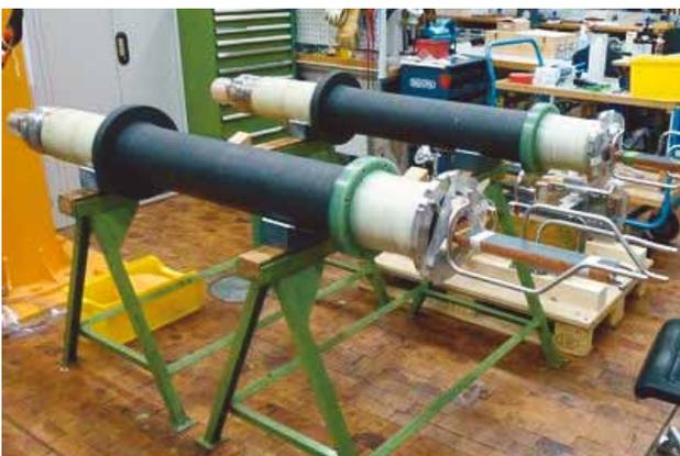
*Fig. 1: W7-X series current leads after assembly.*
