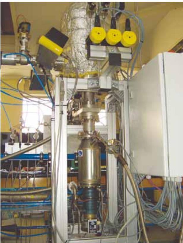
**Fig. 6: The THESEUS facility testing a mercury diffusion pump.**
