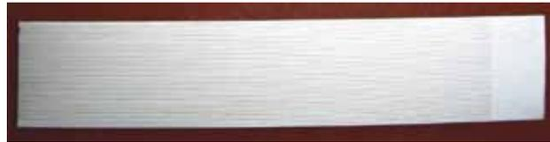
*Fig. 2: Coated conductor with 40 burned filaments.*
