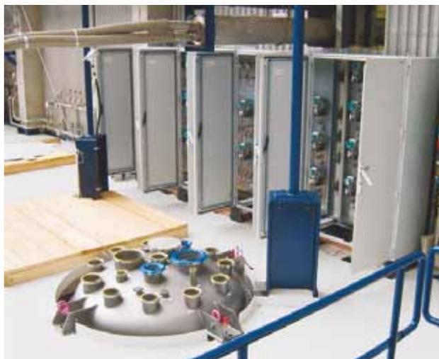
*Fig. 2: Test facility CuLTka under construction for the series test of the JT-60SA current leads.*
