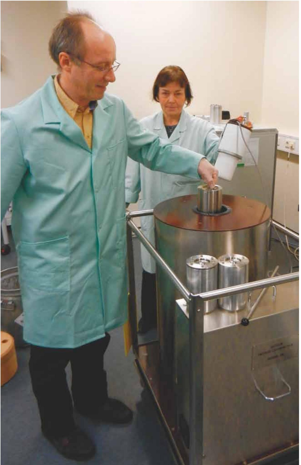
*2\*2. 5 grams of tritium were delivered in November 2011. Activity is measured with a TLK calorimeter for incoming components inspection and mass balance study. Displayed is the insertion of the second tritium container into the calorimeter.*
