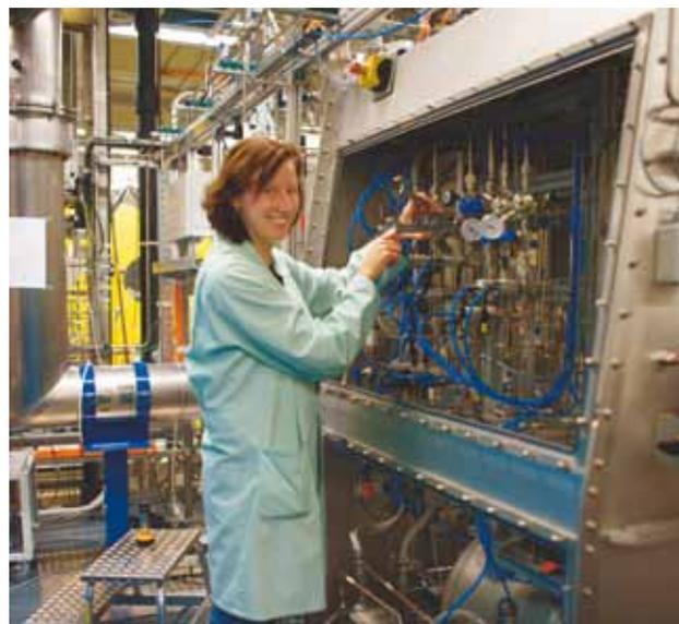
Fig. 2: A view on a part of the Trenta System. The glove box is a connection between WDS and ISS.
