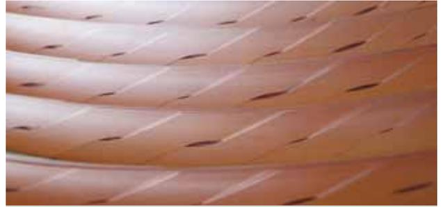
*Fig. 14: Stranded HTS Roebel conductor wire with ten strands, 2 m length and 12 mm width for research at CERN.*
