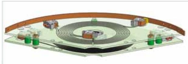
Fig. 11: CAD design of components of the fault current limiter in the project ENSYSTROB.
