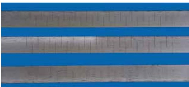
**Fig. 5: Structured coated conductor for use as micro-undulator.**
