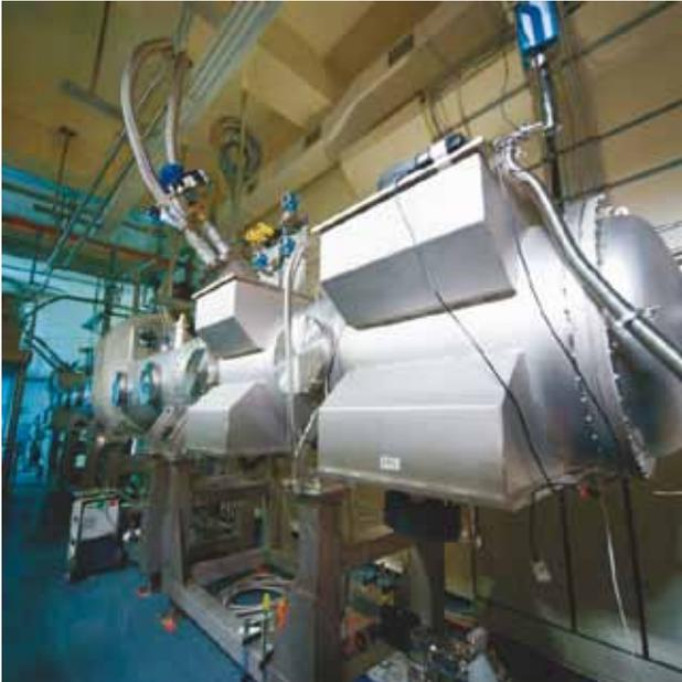
Fig. 8: Shown is the Demonstrator inside TLK for testing the WGTS beam tube cooling.
