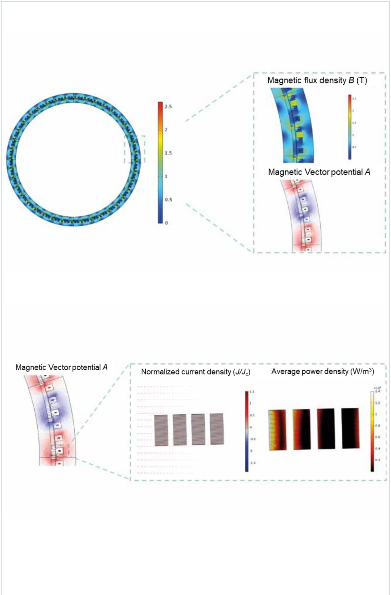
Simulation of the electromagnetic field of a fully superconducting wind turbine generator (top) with simultaneous calculation of the AC losses in the individual conductors (bottom).
