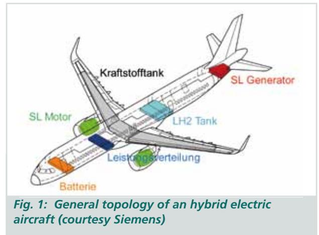
Fig. 1: General topology of an hybrid electric aircraft (courtesy Siemens)
