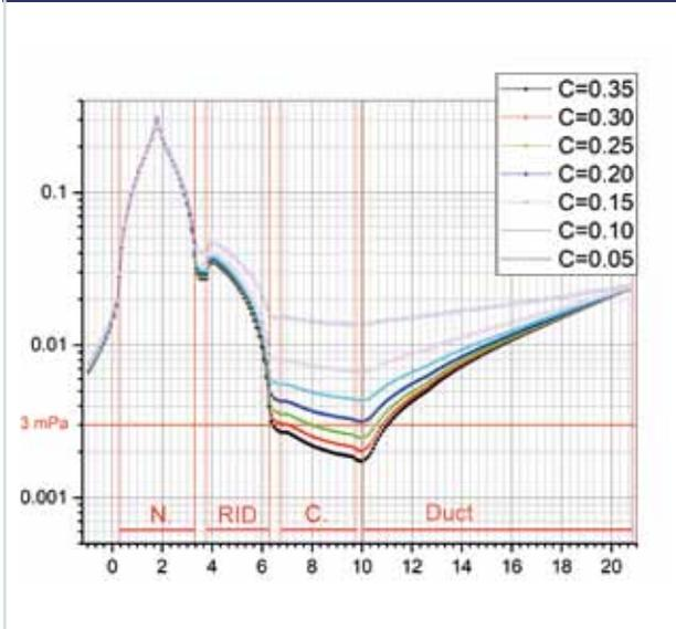
*Fig. 9: Calculated pressure profiles along the DEMO neutral particle injector for different assumed pump efficiencies.*
