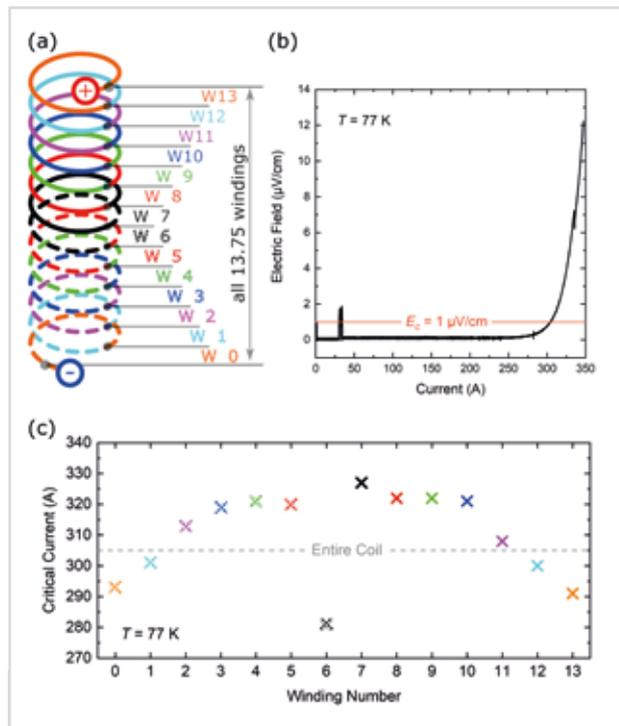
**Fig. 17:** Measurement results of the single-layer HTS CroCo coil in the liquid nitrogen bath ( $T = 77$  K). (a) Schematic of the coil and its instrumentation. The top 7 turns are shown by solid symbols, the bottom 6.75 turns by broken symbols in (c). Equal colors correspond to equal distance of the winding from the coil center. (b) Electric field along the whole coil as a function of coil current. (c) Critical current of the individual windings.
