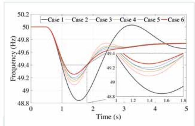
Fig. 8: Flywheel frequency support in microgrids under different controllers' actions.
