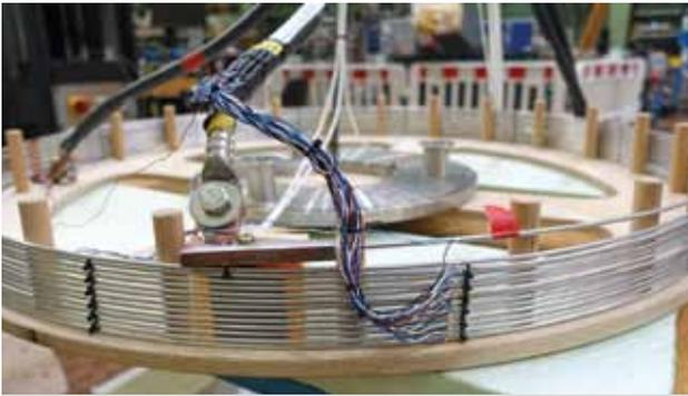
**Fig. 15:** Single-layer, insulated coil of 42 meters HTS CroCo before installation in the test equipment for measurement at  $T = 77$  K. In the foreground a power connection and the instrumentation can be seen. The voltage along each individual winding was measured separately.
