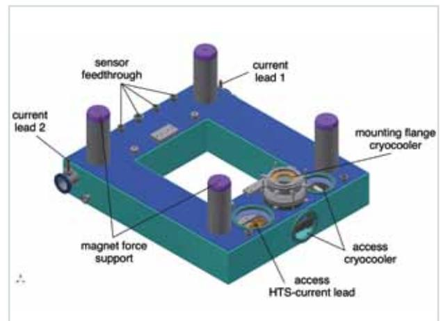
**Fig. 3: Top view of the cryostats of the superconducting magnetic heater**
