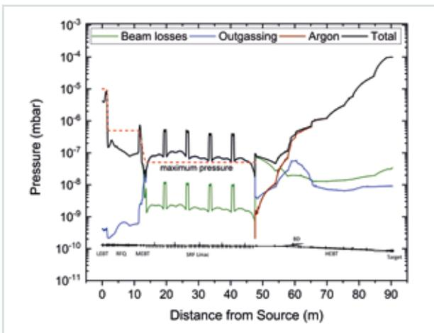
Fig. 3: Pressure profile at the IFMIF-DONES accelerator.
