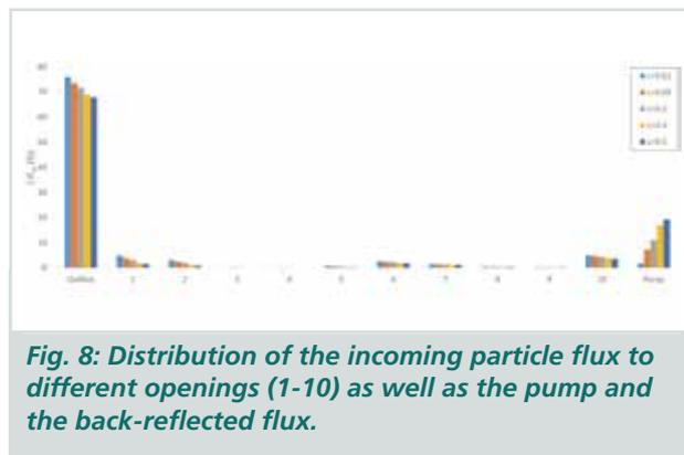
**Fig. 8: Distribution of the incoming particle flux to different openings (1-10) as well as the pump and the back-reflected flux.**
