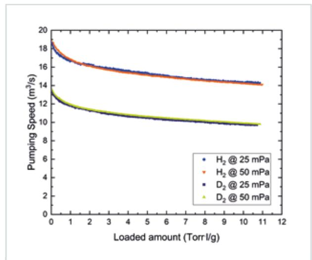
Fig. 5: Isotope dependence of the pumping speed for hydrogen, in comparison at two pressures in each case.
