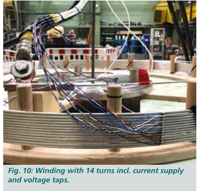
**Fig. 10:** Winding with 14 turns incl. current supply and voltage taps.
