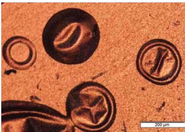
**Fig. 1:** Microscopic image of hydrogen blisters on a copper-coated iron membrane.
