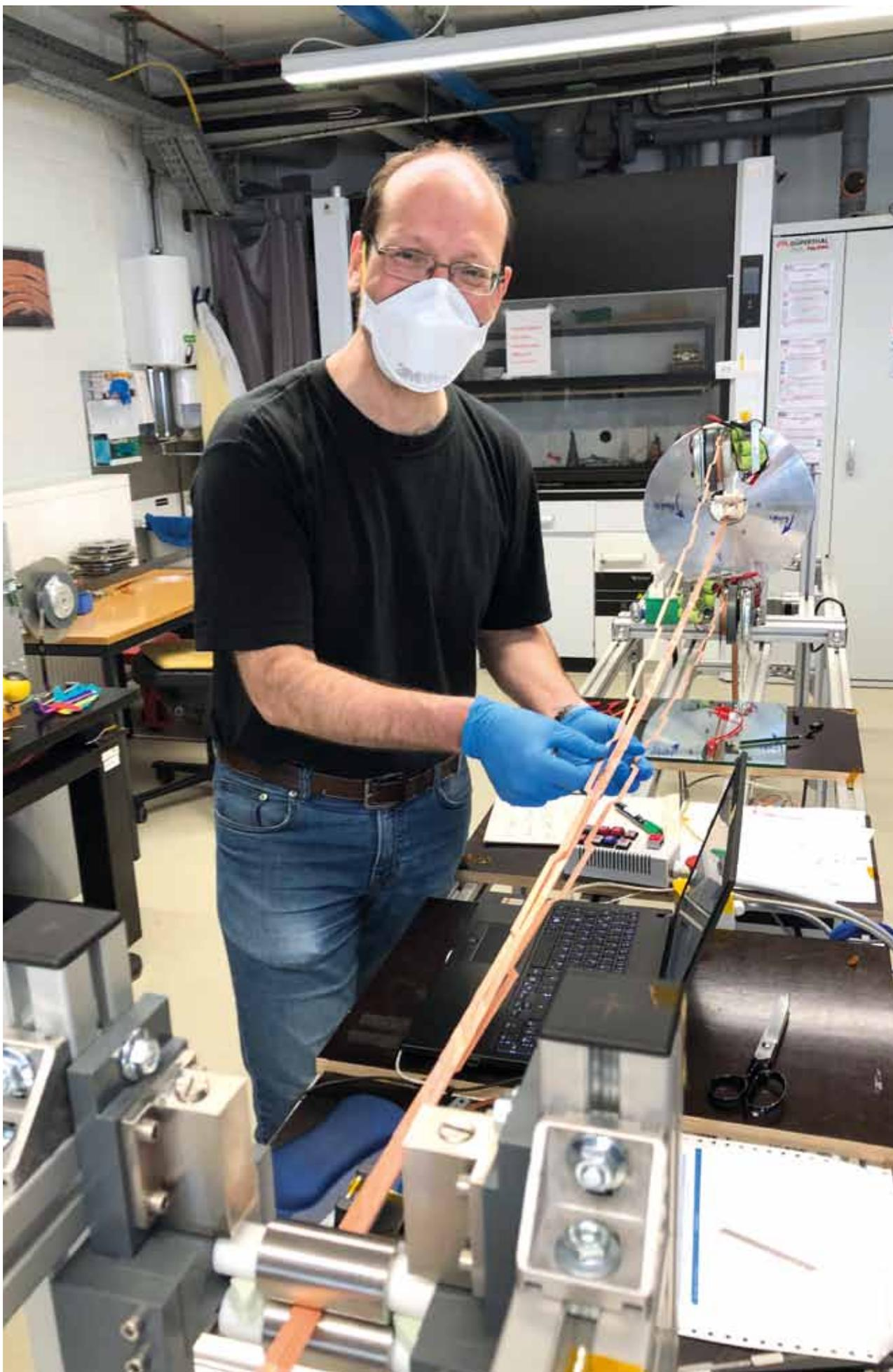
*Cabling of low-loss, high current HTSC ROEBEL cables within a joint KIT-CERN research collaboration to develop HTSC dipole magnets for accelerator storage rings*
