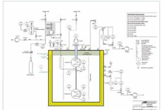
**Fig. 4: Flow diagram of the planned test stand for the investigation of the thermosiphon cooling concept**
