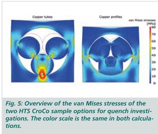
**Fig. 5:** Overview of the von Mises stresses of the two HTS CroCo sample options for quench investigations. The color scale is the same in both calculations.
