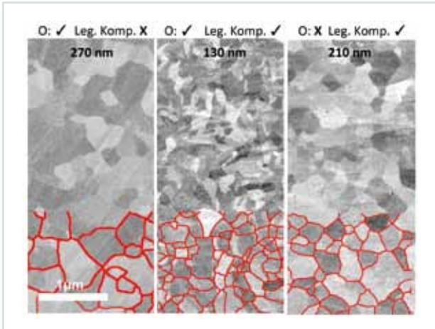
**Fig. 7: Comparison of the grain size of remaining Nb alloy after 300 h at 640 °C. If either O or Zr is present, a reduction of grain growth is visible, indicating a successful oxygen transport into the Nb alloy. The recrystallization is fully suppressed only if both Zr and O are present in a filament.**
