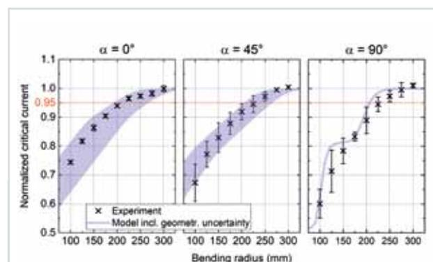
**Fig. 7:** Dependence of the critical current of HTS CroCos as a function of the bending radius for different orientations of the HTS strips to the bending plane.
