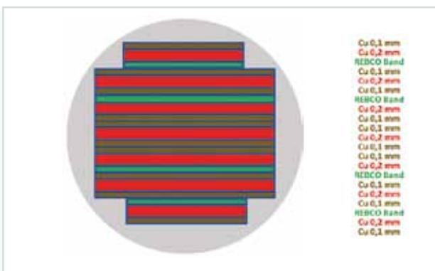
**Fig. 8:** Structure of the HTS CroCo, which was partially equipped with HTS REBCO tapes.
