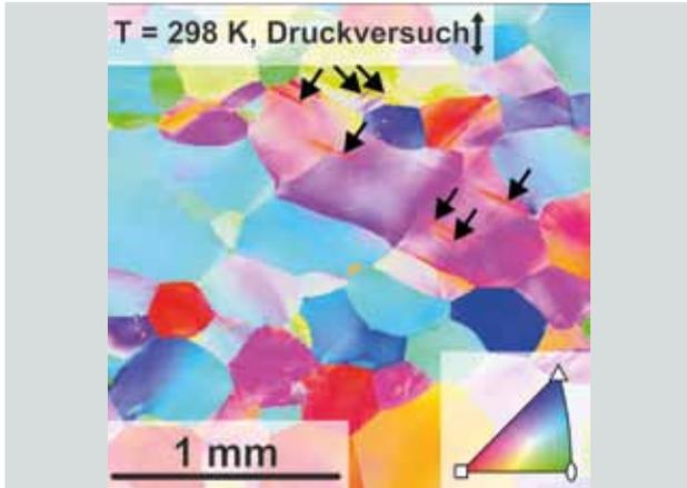
**Fig. 9: Orientation map determined of a longitudinal section of a HfNbTaTiZr sample deformed at 298 K. Double-arrow in top of picture indicates pressure direction, arrows mark kink bands, inset shows orientation.**
