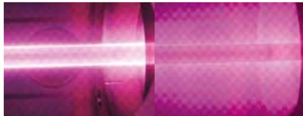
**Fig. 12: Dependence of the plasma shaping at different external magnetic fields.**
