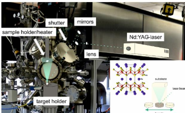
**Fig. 1: Schematic view of the experimental setup, the structure of the Ba122 and the schematic principle of the multi-target PLD**
