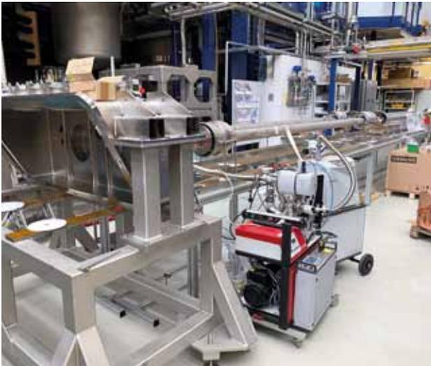
**Fig. 2: Design of the valve box and cryodemonstrator for a 20 K high current line with high temperature superconductors**
