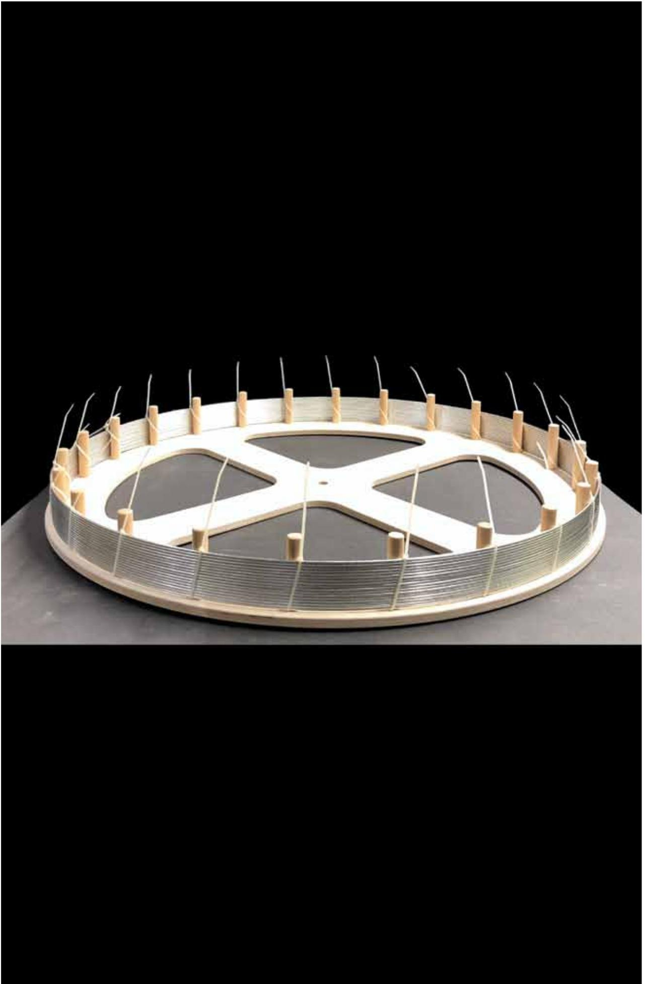
*53 m winding of a HTS CroCo, made of 3mm/2mm REBCO tapes in a continuous manufacturing process*
