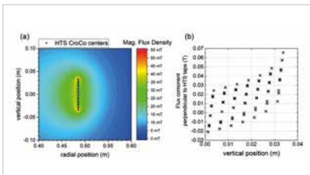
**Fig. 16:** (a) Calculated field geometry and flux density distribution near the HTS CroCo conductors. (b) Normal component of the flux density relative to the orientation of the HTS tapes.
