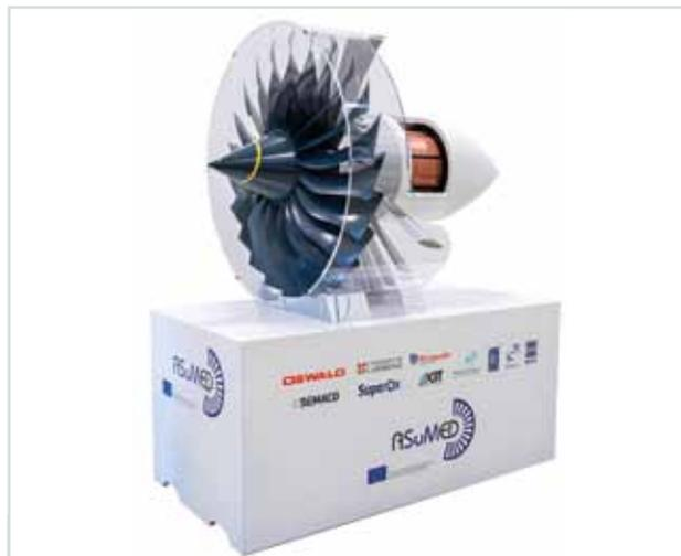
*Fig. 14: Motor with pod and fan for electric aircrafts having a distributed propulsion concept (1 MW, 6000 rpm, 1:1 Mockup).*
