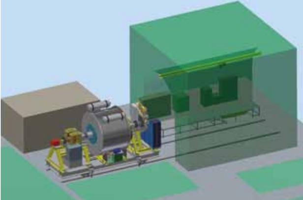
**Fig. 11: CAD-picture of the testrig for cold rotor components based on superconductor technology. The cylindrical vacuum vessel has a diameter of about 2 m.**
