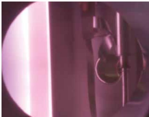
**Fig. 2:** View into the vacuum chamber of HERMESplus during operation. On the left side the shining hydrogen plasma around the plasma source can be seen, on the right-side further installations are visible, among others a membrane, which was wound into a cylinder.
