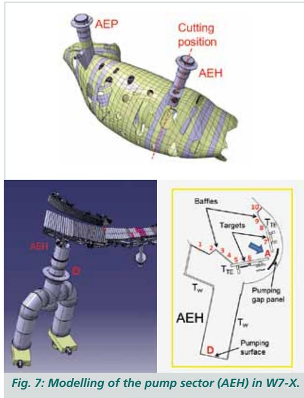
**Fig. 7: Modelling of the pump sector (AEH) in W7-X.**
