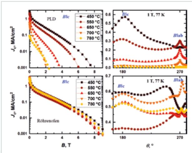
**Figure 4:** Field ( $B||c$ ) and angular dependence (at 1 T) at 77 K for different oxygen annealing temperatures.
