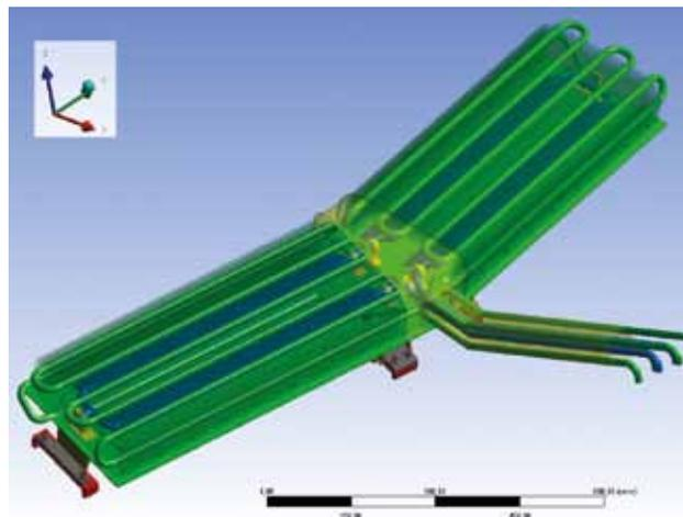
**Fig. 1: Design of the cryopump for JT-60SA.**
