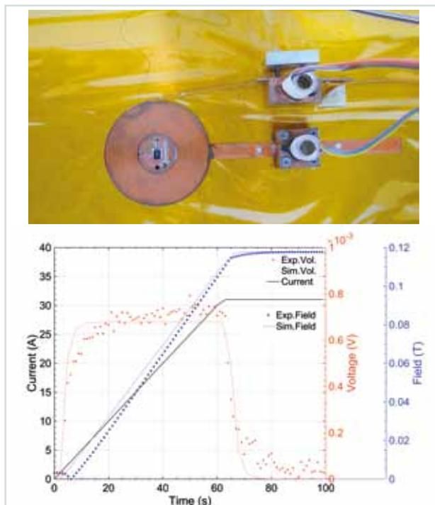
**Fig. 6:** Photo of a HTS-NI coil with 157 turns. The supply lines for the power supply are also visible. Below: Total voltage and central magnetic field with a ramp rate of 0.5 A/s and a specific contact resistance of  $90 \mu\Omega \cdot \text{cm}^2$ .
