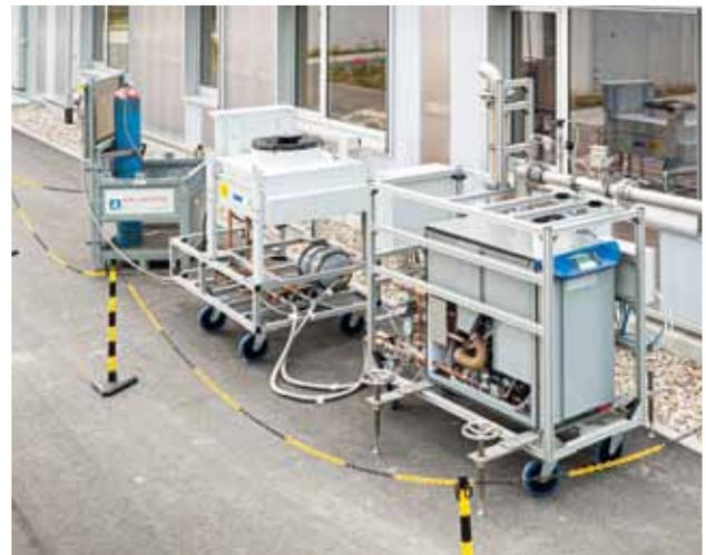
Fig. 9: Micro-gas turbine experimental setup.
