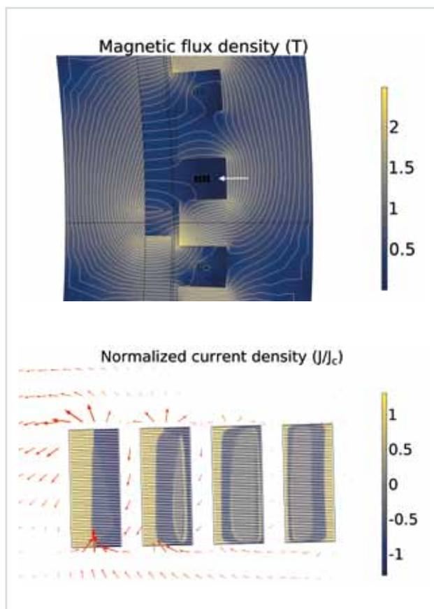
**Fig. 5:** Top: Distribution of magnetic flux density in one of the designs of the superconducting generator of a wind turbine. Below: Distribution of the normalised current density in four half coils (see white arrow). The red arrows indicate the direction and strength of the magnetic field. The left half of the coil, which is saturated with current and exposed to a high magnetic field, is the one with the highest losses.
