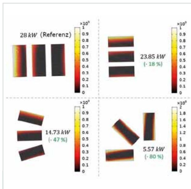
**Fig. 13: Variations of a HTS stator winding. Compared to the reference configuration the ac loss can be reduced by 18%, 47% or 80% by specific orientations in the slot.**
