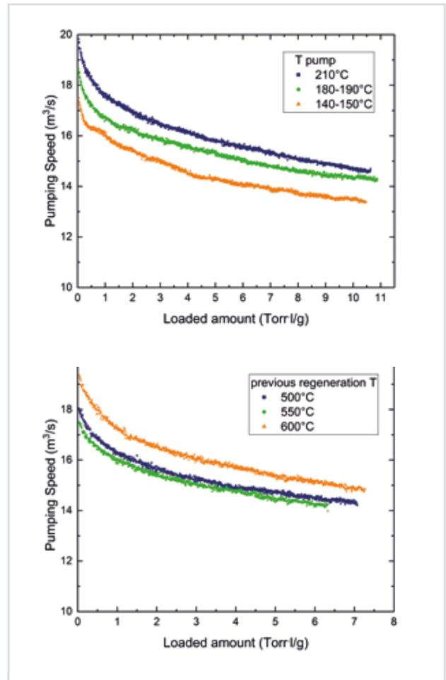
Fig. 4: Influence of getter temperature on the pumping speed for H<sub>2</sub>; during pumping (top) and in the regeneration step before pumping (bottom).
