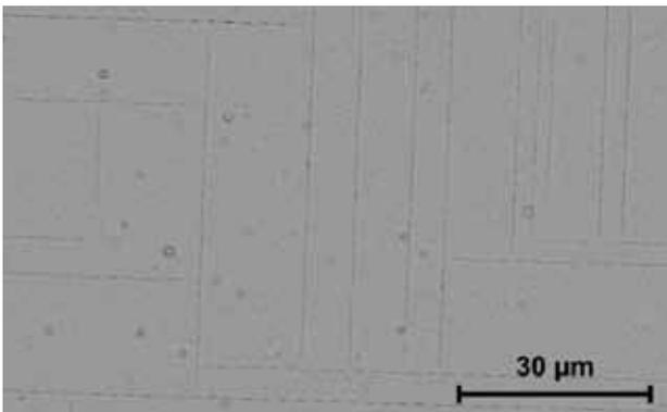
**Fig. 5:** Crack formation in  $YBa_2Cu_3O_7$  on LSAT single crystal substrates during too fast a cooling process. The cracks are parallel to the  $a$ - and  $b$ -axis of  $YBa_2Cu_3O_7$ .
