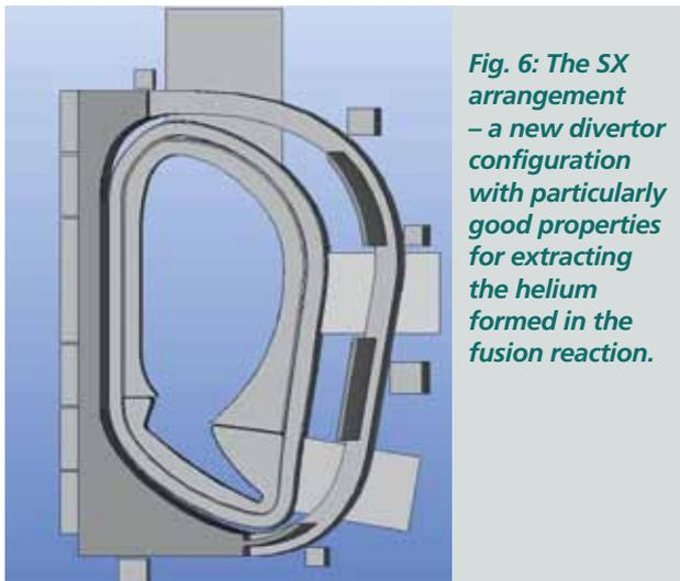
**Fig. 6: The SX arrangement – a new divertor configuration with particularly good properties for extracting the helium formed in the fusion reaction.**
