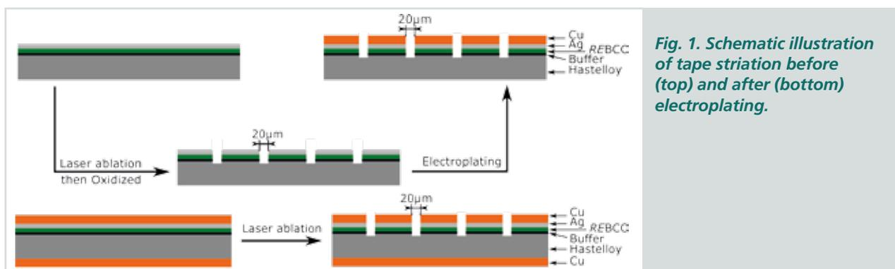
**Fig. 1. Schematic illustration of tape striation before (top) and after (bottom) electroplating.**
