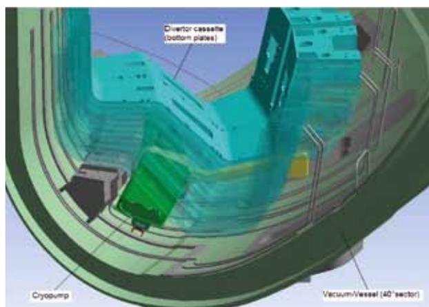
**Fig. 2: View of the installation of one of the nine cryopumps in the JT-60SA plasma vessel.**
