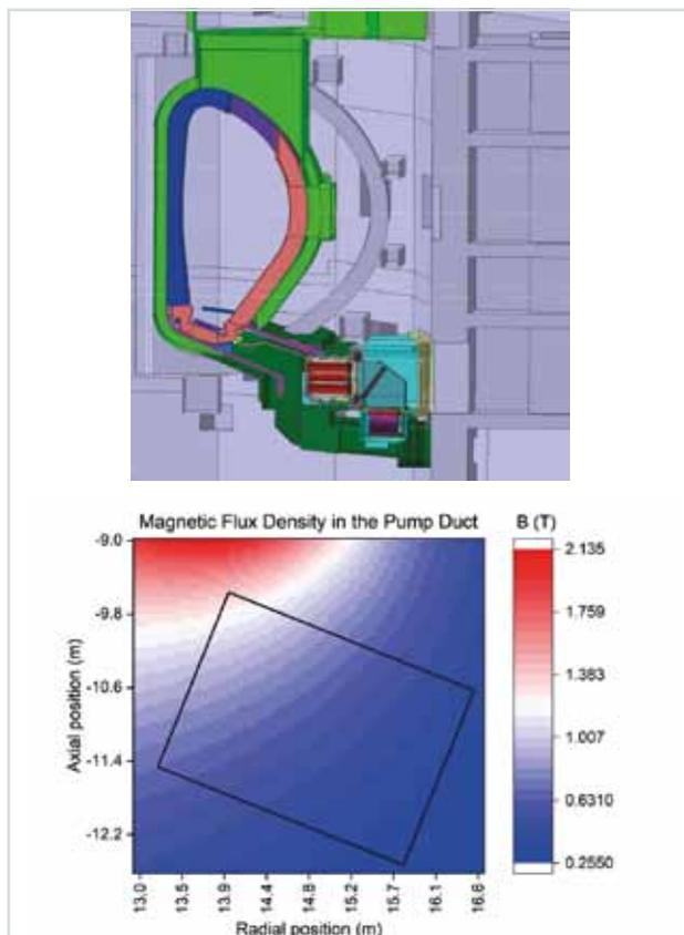
**Fig. 11: Indication of the field strength conditions at the potential installation site of the metal foil pumps at DEMO.**
