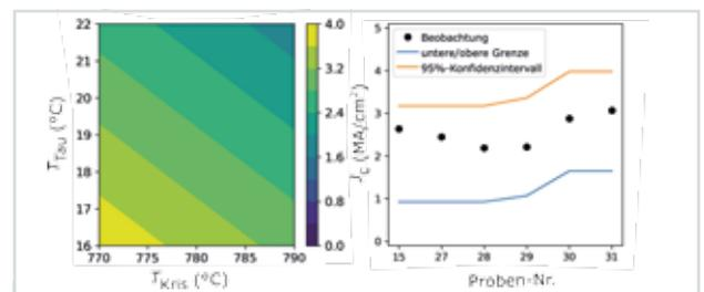
**Fig. 3: Dependence of  $J_{\text{c}77}^{\text{sf}}$  on humidity and  $T_{\text{crys}}$  at fixed  $p_{\text{O}_2}$  (left) and model confirmation for  $J_{\text{c}77}^{\text{sf}}$  (right).**
