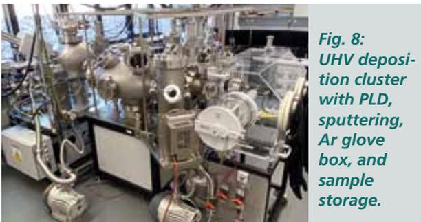
**Fig. 8: UHV deposition cluster with PLD, sputtering, Ar glove box, and sample storage.**
