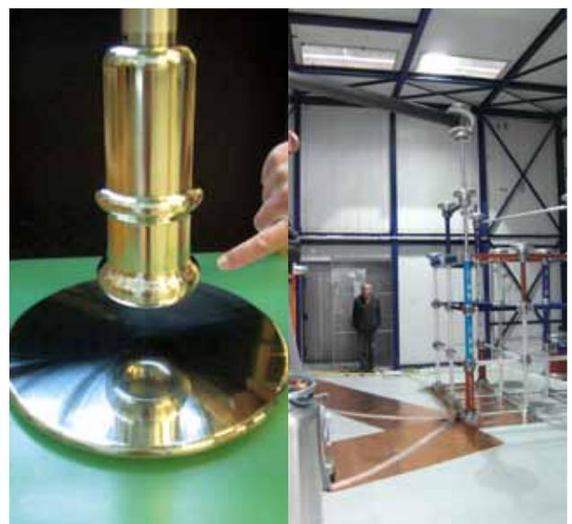
**Fig. 4: On the left: Bell-plate arrangement to study the breakdown behaviour in liquid nitrogen. Right: Setup of the test cryostat in the cryogenic high voltage laboratory of the ITEP**
