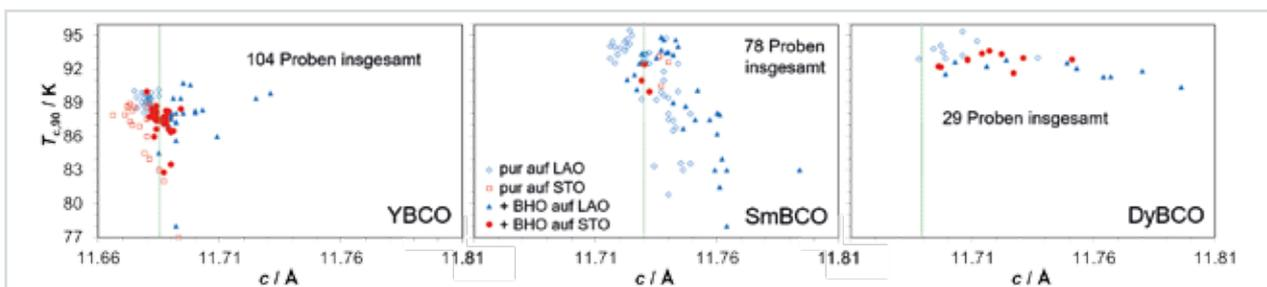
Fig. 1. Dependence of the critical temperature  $T_c$  on the  $c$ -axis lattice parameter for YBCO, SmBCO, and DyBCO.
