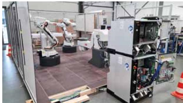
**Fig. 1: Advanced stage of the robot chamber with two robots, positioning table and partially constructed protective screen. In the foreground the electronic controls for the robots can be seen.**
