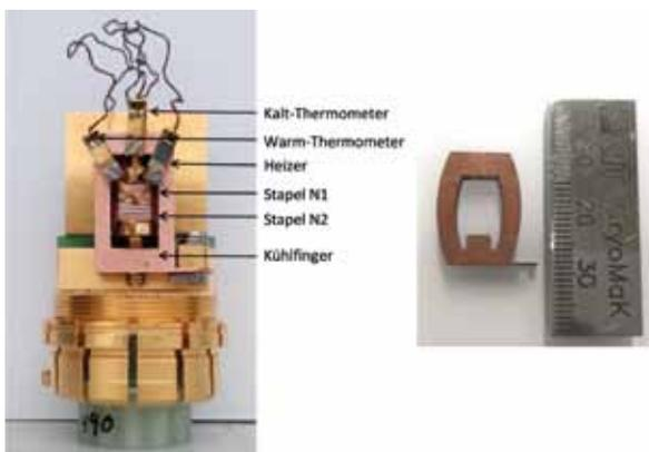
**Fig. 10: Left: Copper frame mounted on probe platform with installed stack N1 and N2. Right: adapted frame to measure contact pressure simultaneously.**
