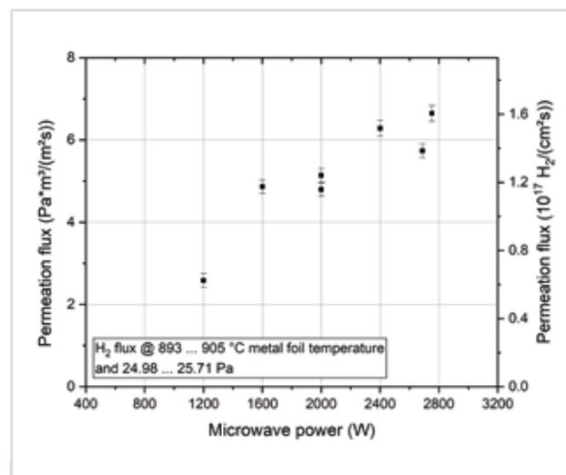
**Fig. 13: Performance data of hydrogen through a niobium foil at about 900°C at a pressure of about 25 Pa.**
