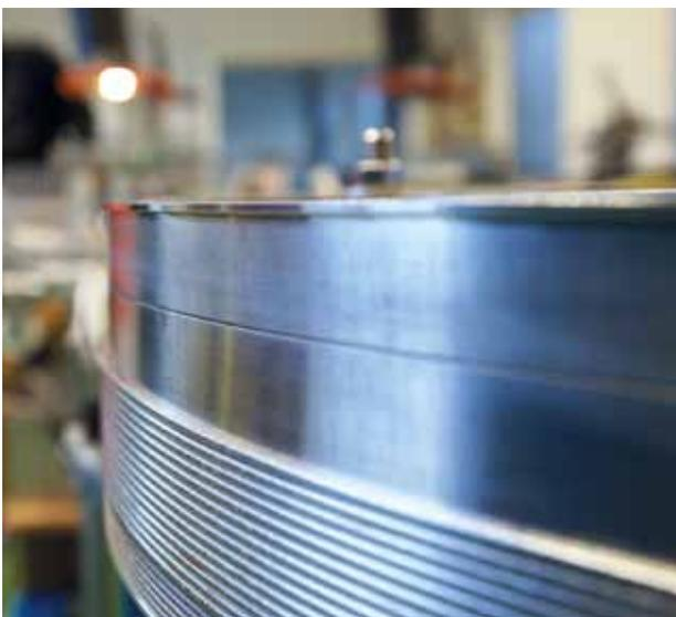
**Fig. 9:** Receiver reel with the first 14 turns of the HTS CroCos during the production of the winding.
