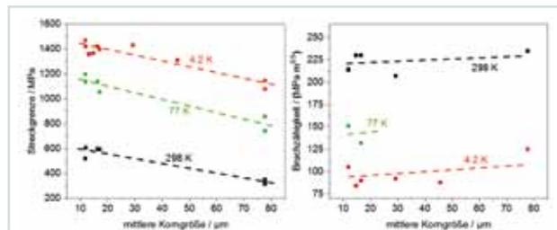
**Fig. 11: Increasing yield strength with decreasing grain size on the left, constant fracture toughness at different temperatures on the right.**
