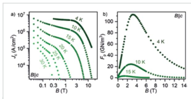
**Fig. 6:** Magnetic field dependence of  $J_c$  (a) and corresponding  $F_p$  (b) of a (Li,Fe)OHFeSe film for several temperatures.
