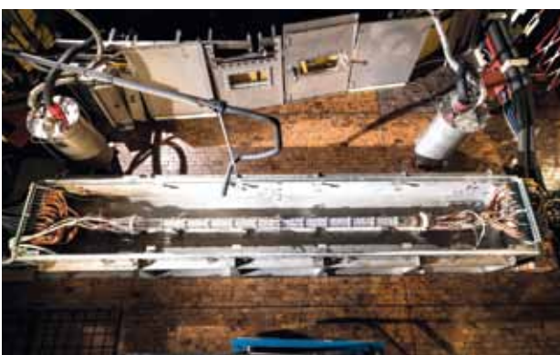
Fig. 3: Setup of a 35 kA DC cable demonstrator with 12 Croco conductors
