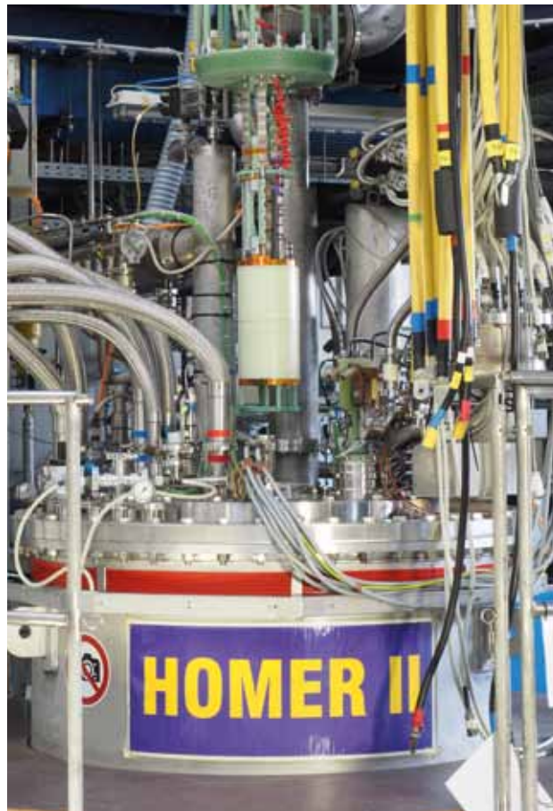
Fig. 18: Insertion of the HTS insert coil into the HOMER II cryostat in which the base NbTi and NbSn magnet system is already situated.
