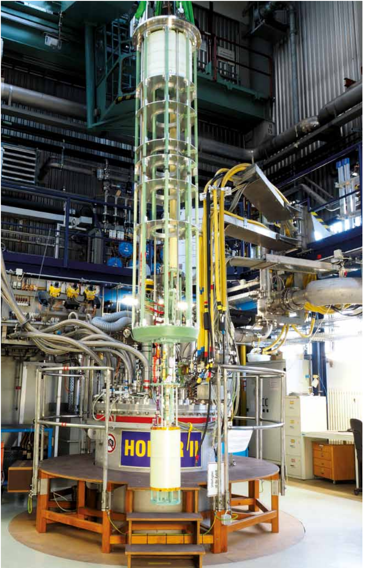
HTS insert coil in front of HOMER II during installation
