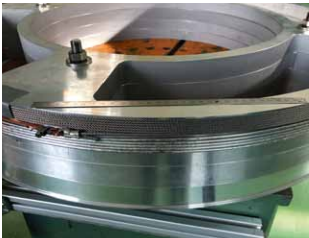
Fig. 8: Several HTS CroCo windings (made from Cu and HTS tapes of 2 mm and 3 mm width) spooled on a drum of 100 cm diameter
