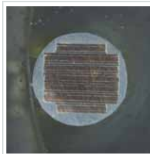
Figure 8: Polished cross-sectional image of a HTS CroCo conductor made of 2 mm and 3 mm wide tapes. The cross-shaped tape stack and the round solder shell is very well formed.
