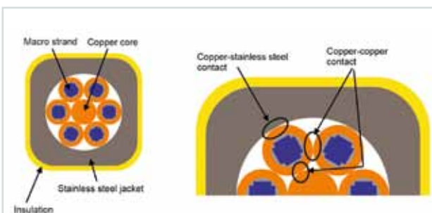
Fig. 6: Schematic representation of the contacts present in an HTS-CICC
