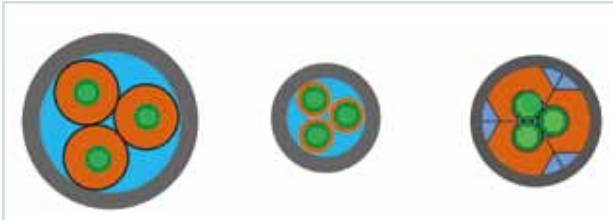
Fig. 4: Schematic representation of three CroCo conductor concepts for a quench experiment in SULTAN: reference design (left), design with low copper content (middle) and design with copper profiles (right)
