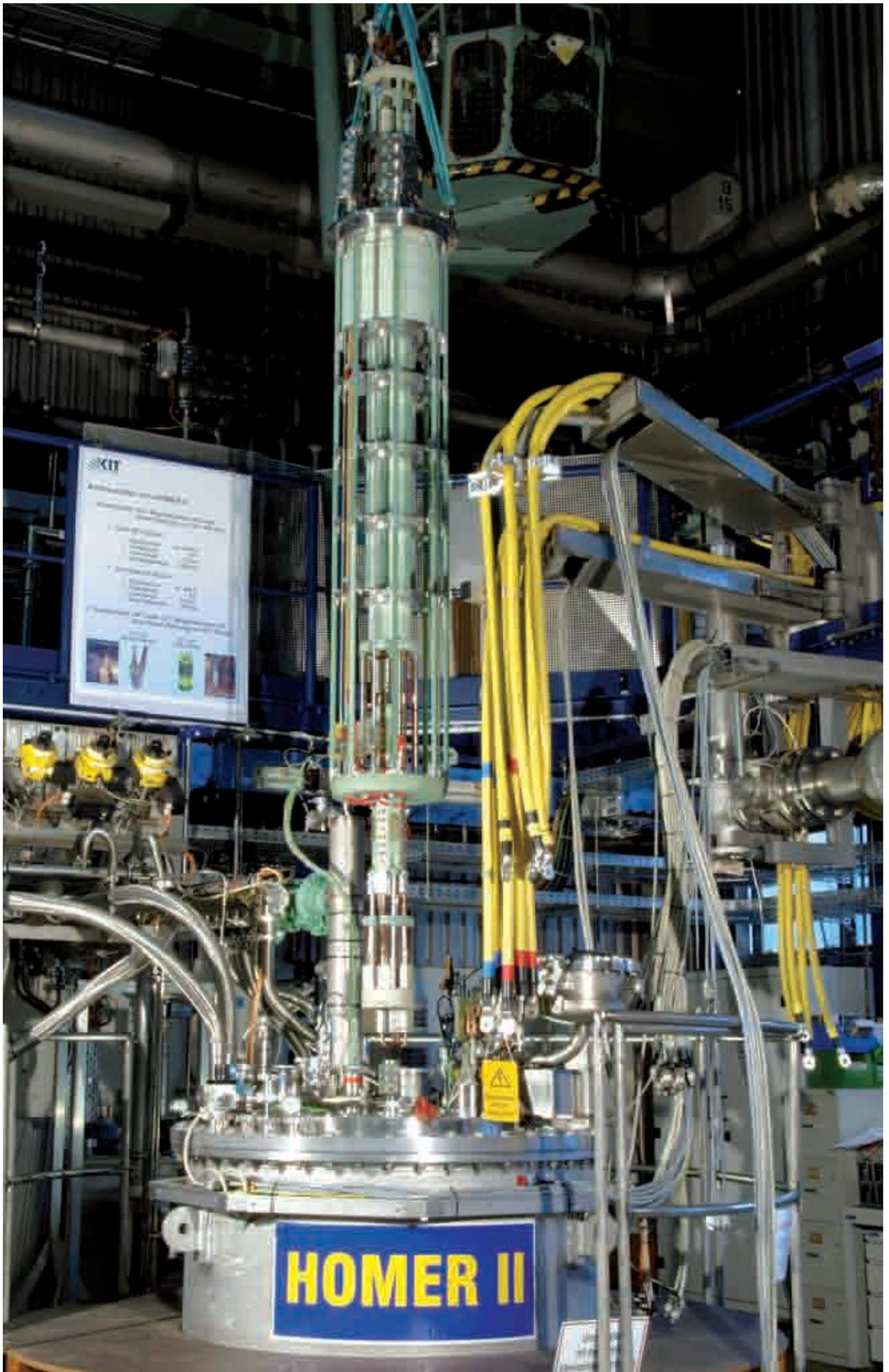
*HOMER II – Superconducting High Field Magnet facility with magnet flange and triple insert coil.*
