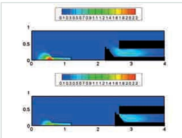
Fig. 11: Representation of the Mach number contours for helium and two valve positions (100 % open and 25% open).
