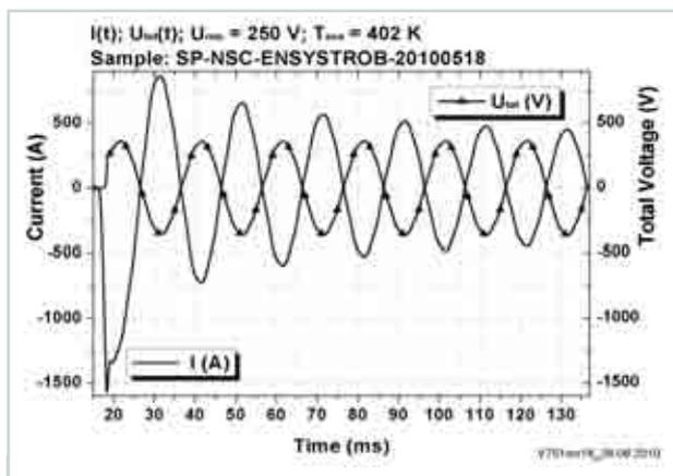
Fig.8: Short-circuit test of a current limiter model component.
