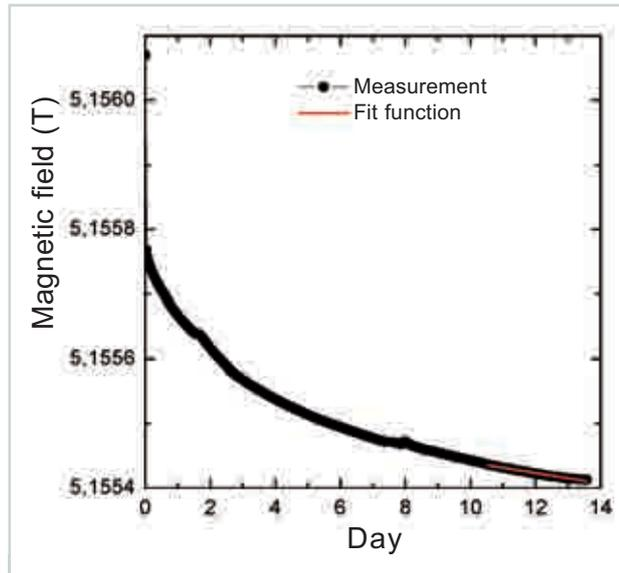
*Fig. 12: Measurement of magnetic field stability in module 5 in the period between October 26 and November 29, 2010. The red line is explained in the text.*
