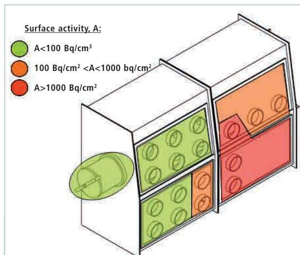
**Fig. 5:** Map of surface contamination of the inside of the PETRA glove box in TLK.
