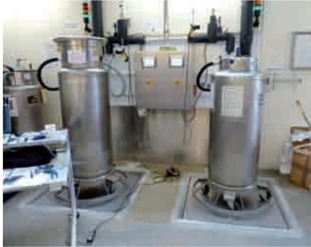
*Fig. 6: LN<sub>2</sub> filling station.*
