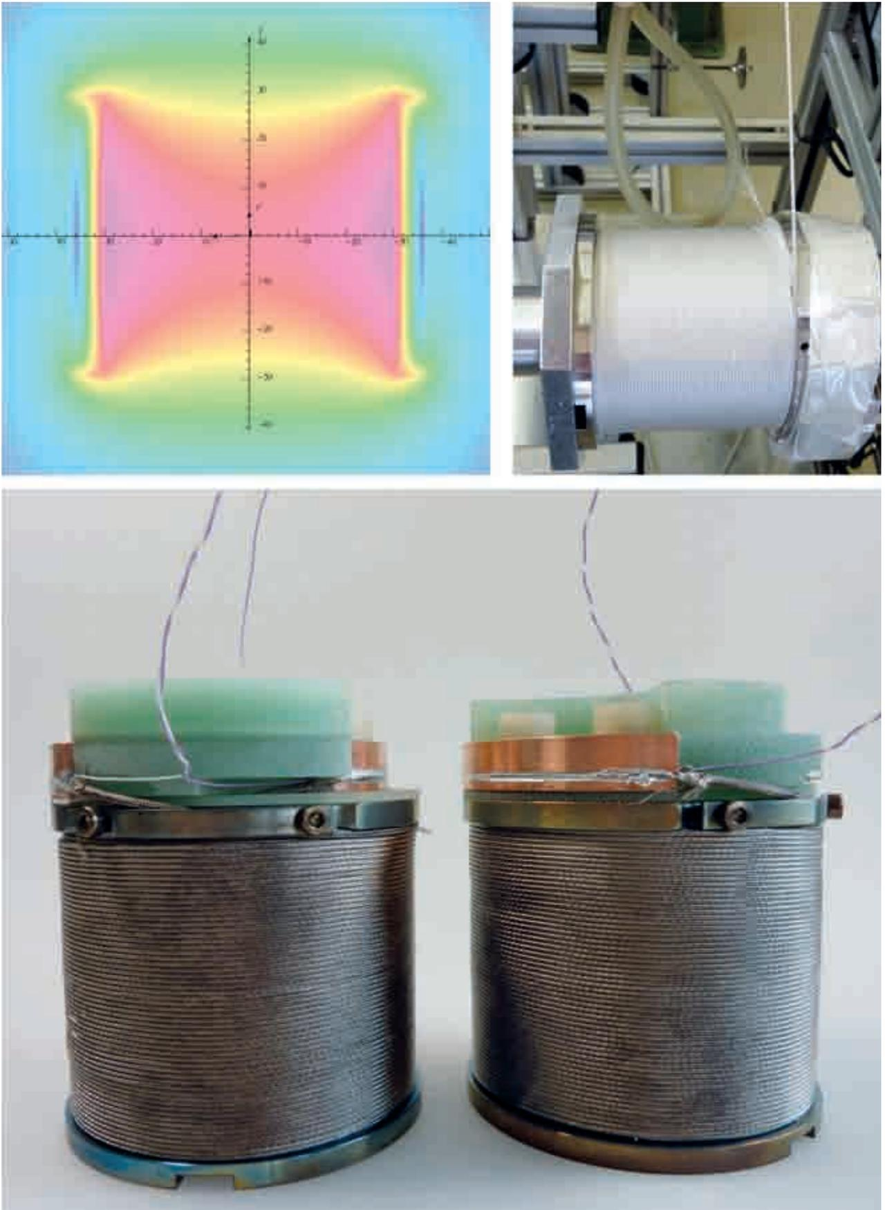
*Field computation for an MgB<sub>2</sub>-coil (top left), coil production (top right), and annealed coils prior to sealing with wax (bottom).*
