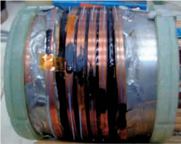
*Fig. 5: NbTi test coil with FBG sensors.*
