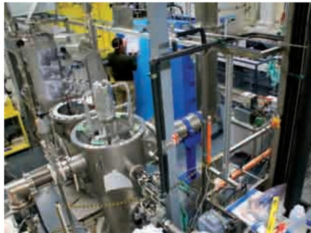
*Fig. 4: View of the TRENTA facility: In the front left, the opened cryocolumn can be seen. The black column on the right hand side of the picture is part of WDS. The blue unit in the background is the Linde cryofacility for ISS.*
