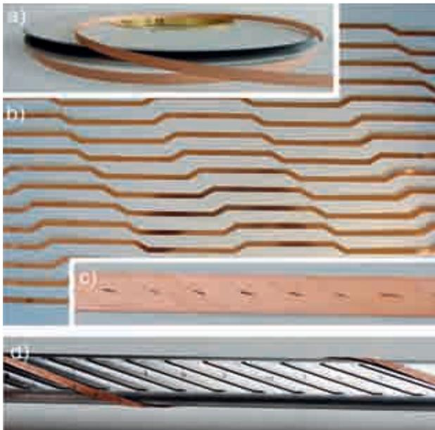
Fig.2: Commercial REBCO-CC strip (a), punched strips (b), Roebel cable (c), Rutherford cable mold with a Roebel strand (d).
