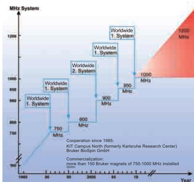
**Fig. 5: Chronological development of the superconducting magnet systems for high resolution NMR spectroscopy for frequencies from 750 MHz.**
