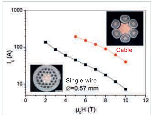
Fig.4: Comparison of the current carrying capacities of a single  $MgB_2$  wire and a cable made up of six single wires.
