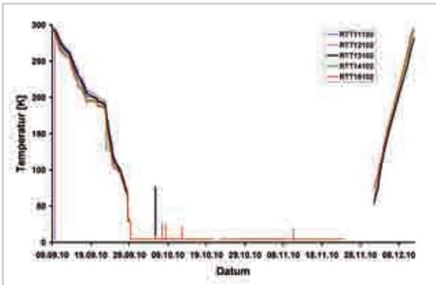
*Fig. 11: Temperature curve of the five magnet modules of DPS during the first commissioning phase. The five peaks in October and November are the temperature increases caused by magnet quenches and a fast discharge of the field via the safety diodes, respectively.*
