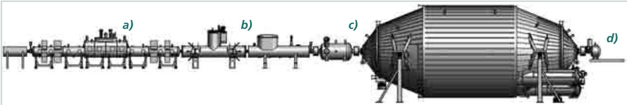
**Fig. 1:** Schematic diagram showing the KATRIN international large experiment. The electrons produced in  $\beta$ -decays in a high-intensity windowless molecular tritium source (WGTS, a) are passed through a tritium pumping section with the active and passive elements of DPS2-F and CPS (b) to a system (c) consisting of two electrostatic spectrometers (roughing and main spectrometers). The analyzed electrons are detected in a solid-state detector (d).
