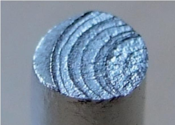
*Fig. 9: Fracture surface of 4 mm dia. of a fatigue specimen made of PF jacket material after some 25,000 cycles at a loading amplitude of 100 MPa to 1100 MPa at 4.2 K.*
