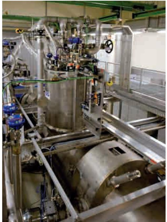
*Fig. 9: View of DPS after assembly of all connecting lines (such as those leading to the cryotransfer line).*
