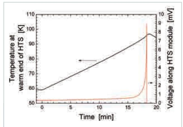
Fig. 7: Temperature and voltage during simulation of a loss of coolant.
