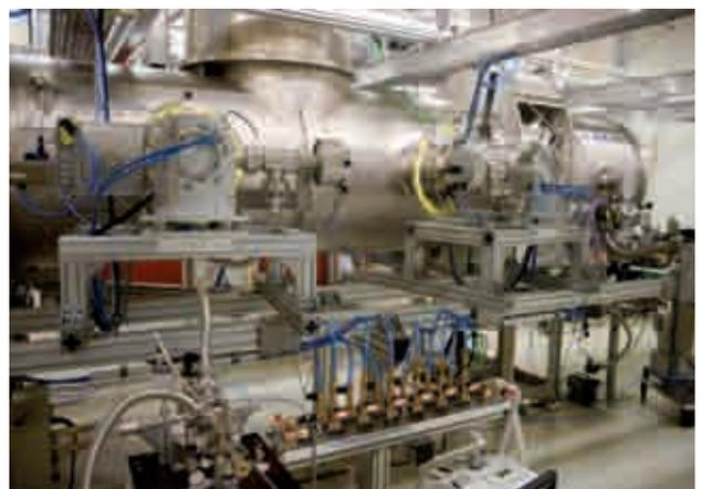
*Fig. 10: View of pumping chambers No. 2 and 3 and the attached valves and turbo molecular pumps of the MAG2800 type.*
