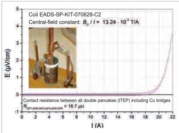
**Fig.13: Determining the critical current of a REBCO-CC split-coil magnet.**
