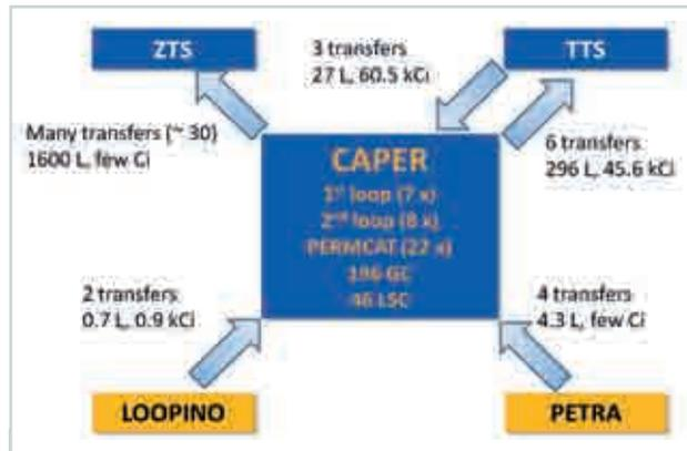
*Fig. 2: Survey of tritium transfers of the CAPER plant. Waste gases came from LOOPINO and PETRA.*
