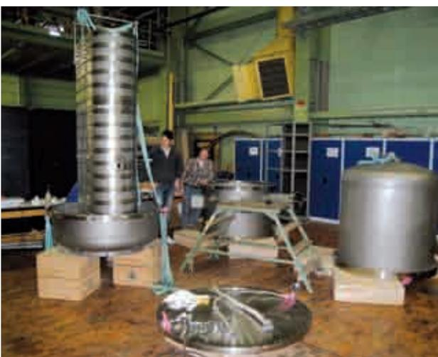
*Fig. 1: Test cryostat with cryoshield.*
