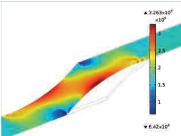
*Fig. 5: FEM computation of the stress distribution in a Roebel tape under axial loading.*
