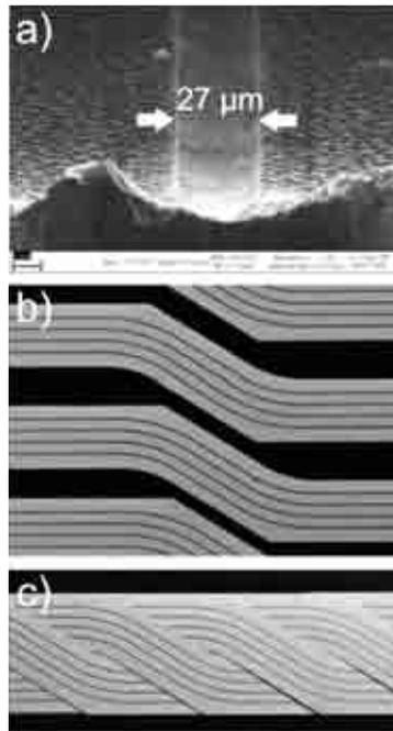
**Fig.1: SEM-image of a slit 27 micrometers wide made by a picosecond laser in the superconducting layer of a REBCO strip conductor (a); slitted Roebel strands (b), and Roebel cable with slitted strands (c).**
