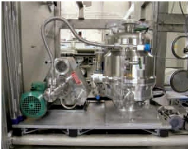
**Fig. 6:** TRITOP experiment under construction. The two pumps involved can be seen; on the left, Nor-metex ("triangle"), on the right, the MAG2800 turbopump.
