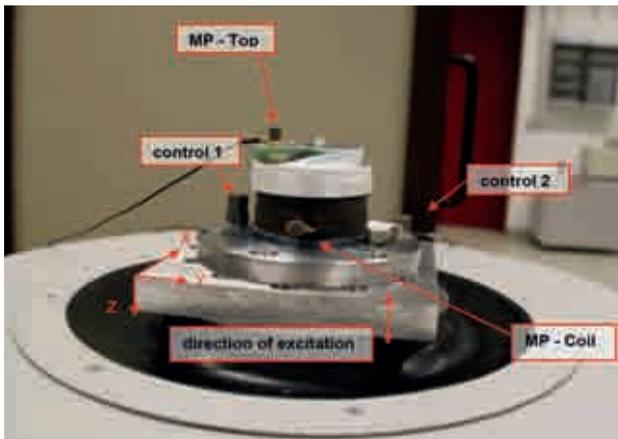
Fig.10:  $MgB_2$  coil mounted on a shaker for excitation in the axial direction (z-direction).
