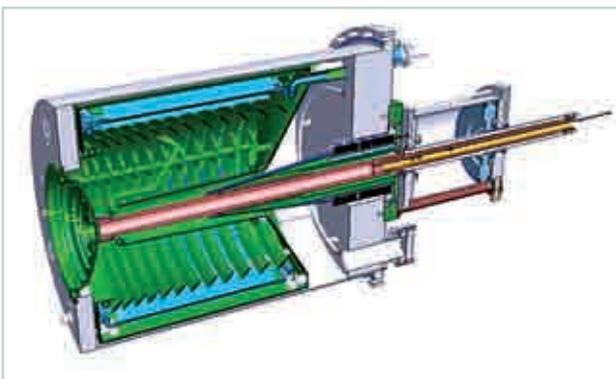
*Fig. 1: 3D CAD-model of the prototype torus cryopump.*
