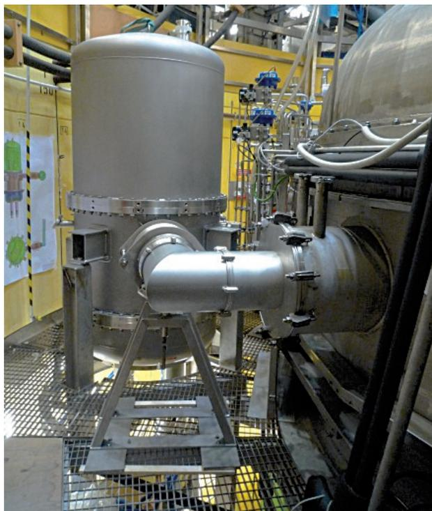
*Fig. 3: Test cryostat with prototype power supply lead in the test phase.*
