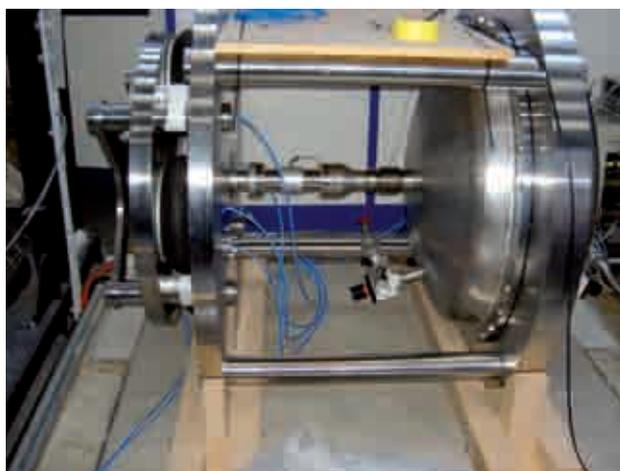
*Fig. 2: Facility for testing static metal seals.*
