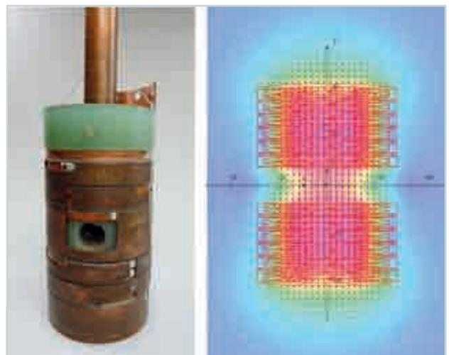
Fig.12: Coated-conductor split-coil magnet consisting of twice three double pancakes (left), and field distribution computed with OPERA-3D (right).
