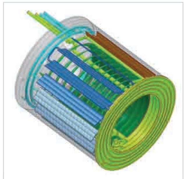
Fig. 8: The cryogenic parts of the pump are replaced by an equivalent volume (cylindrical shell).
