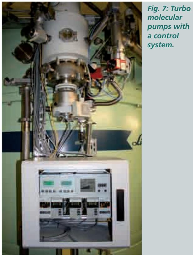
*Fig. 7: Turbo molecular pumps with a control system.*
