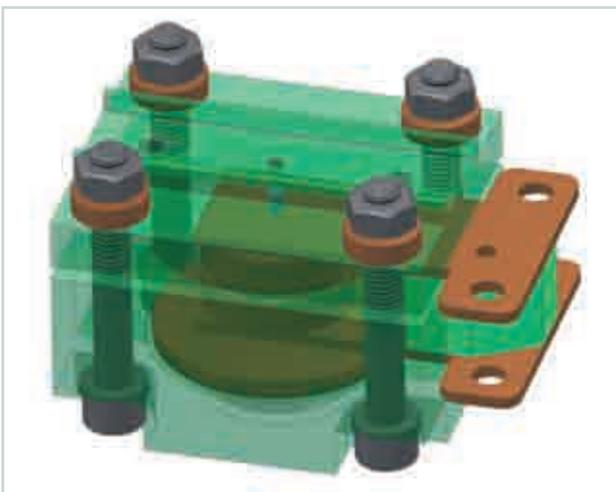
Fig. 4: Diode housing for  $U(I)$  measurement.
