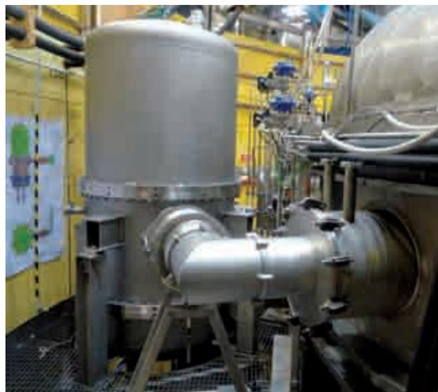
**Fig. 2: Test cryostat for the test of the W7-X prototype power supply leads in TOSKA.**
