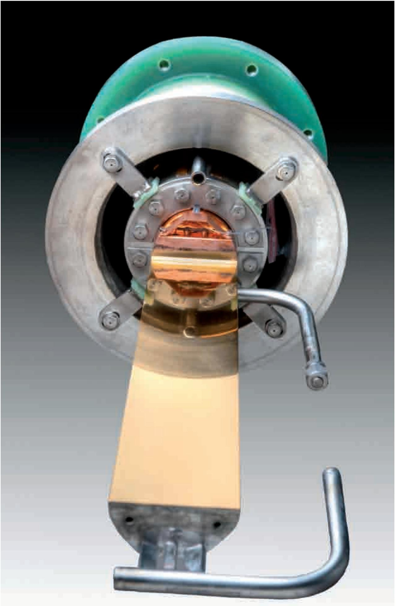
*Cold contact (4,5k) of the 18200 Ampere HTS current lead*
