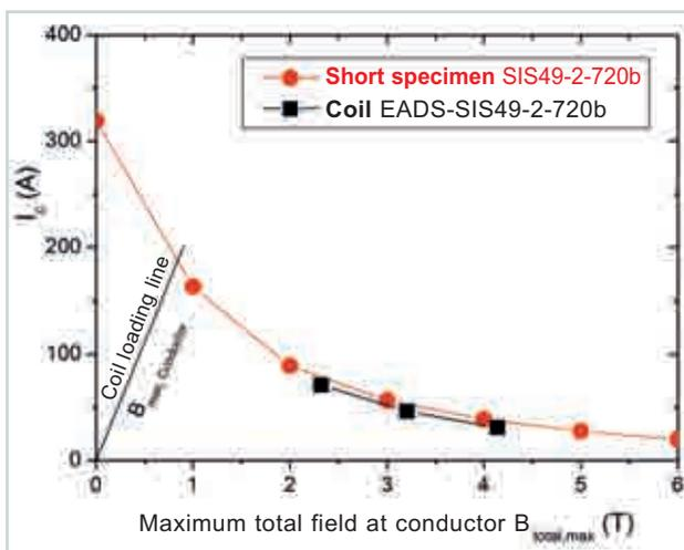
Fig.11: Current carrying capacities of a short  $MgB_2$  specimen produced at KIT, and a coil produced from this wire, as a function of the maximum total field along the conductor. The loading line shows the connection between the coil current and the maximum field in the coil without a background field.
