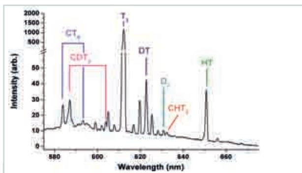
**Fig. 7:** LARA spectrum recorded in the Loopino test loop with a tritium gas mix of extremely high purity (approx. 97%), which was left in the loop for 21 days. The methane species ( $CT_n$ , etc.) generated can be seen clearly.
