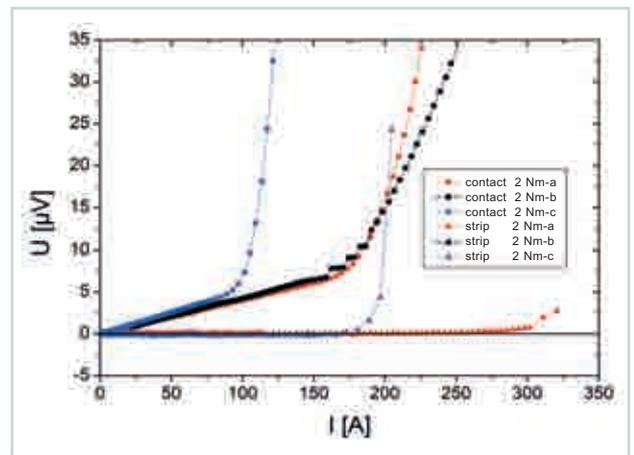
Fig.5: Three Ag diffusion contacts bolted with 2 Nm.
