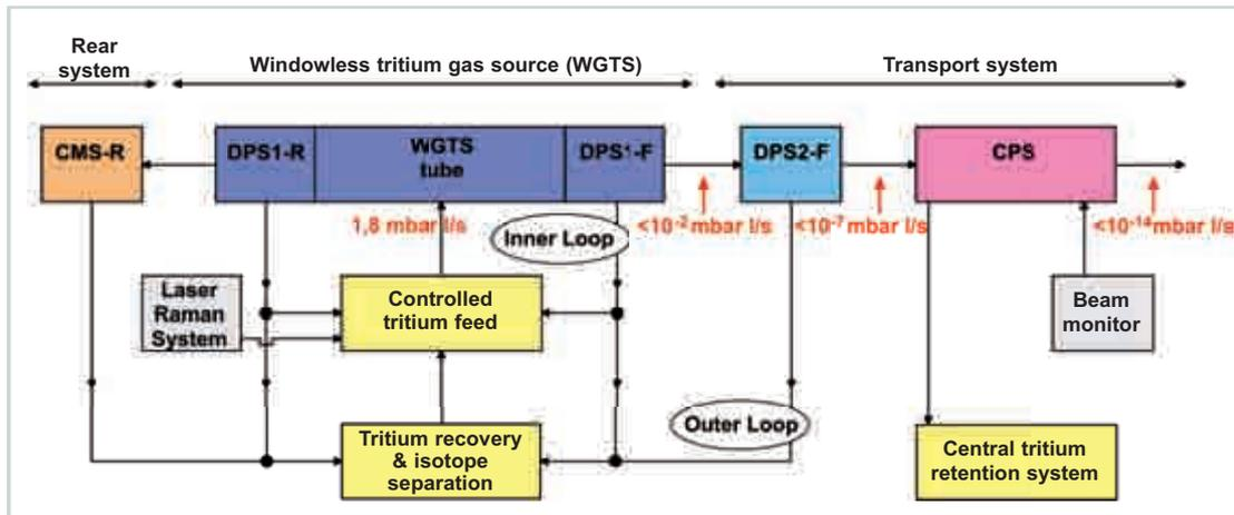
Fig. 3: Block diagram of the KATRIN tritium source and its interfaces with the infrastructure of TLK.
