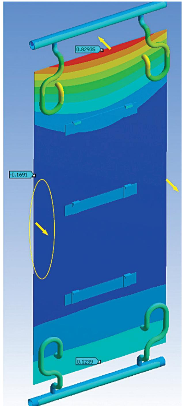
Fig.5: Computing the bending, in mm, forward (negative) and backward (positive) of a thermal shield during cooling from 300 K to 80 K.
