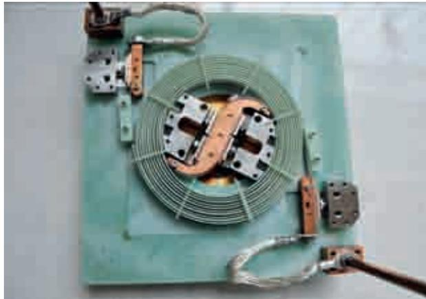
Fig.7: Test component of an HTS current limiter made of a coated conductor.
