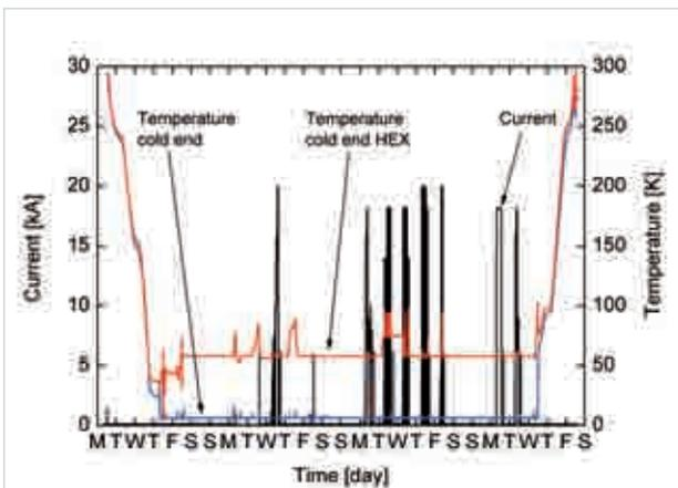
Fig. 6: Time curve of the prototype test from cooling to experimental operation to heating.
