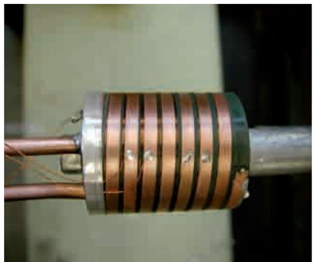
Fig. 3: Test object with YBCO winding.
