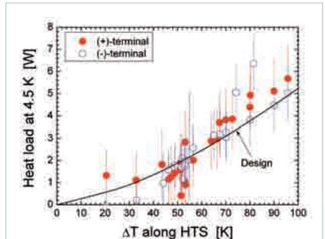
Fig. 8: Thermal load at the 4.5 K level as a function of the temperature gradient across the HTS module.
