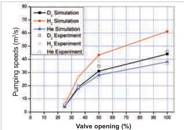
Fig. 10: Simulation results compared with TIMO measurements.
