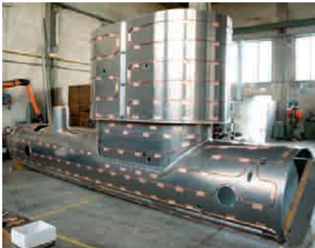
**Fig. 5:** Thermal shield of CPS. In the middle of the system, which is more than 7 m long, the high tower can be seen which later will accommodate the large IHe tank.
