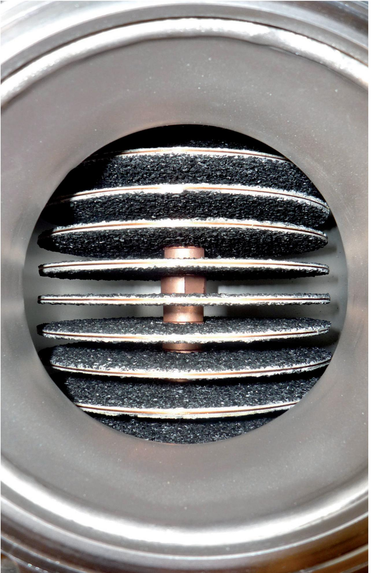
*Prototype cryosorption pump for SIS100/FAIR*
