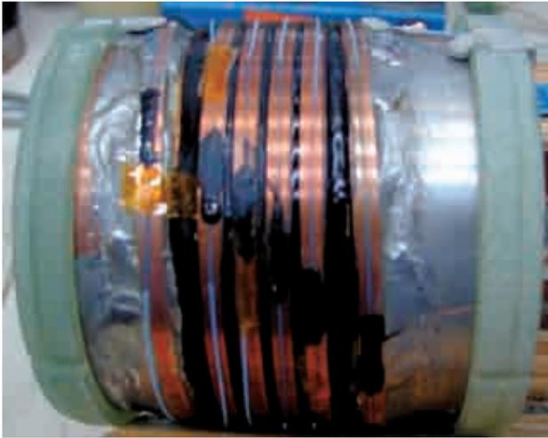
*Fig. 5: NbTi test coil with FBG sensors.*
