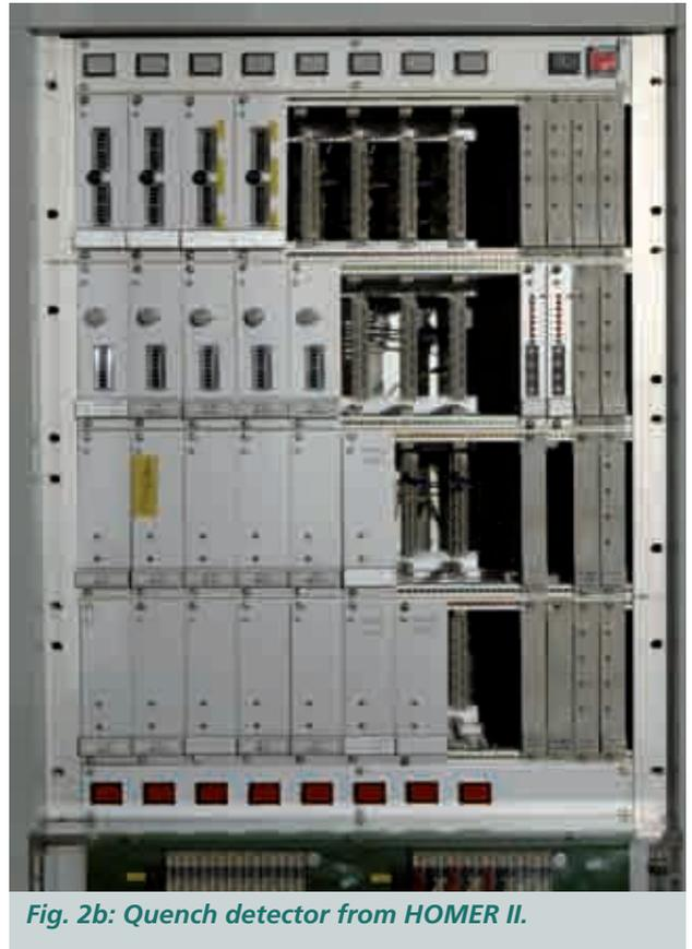
Fig. 2b: Quench detector from HOMER II.
