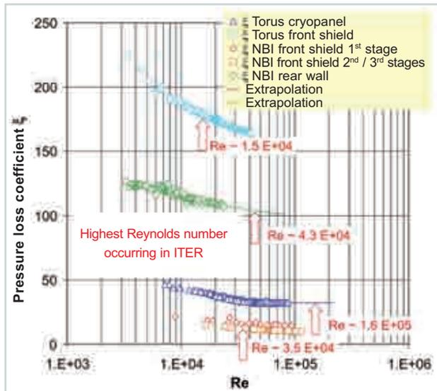
**Fig. 6: Pressure loss coefficients,  $\xi$  as a function of the Reynolds number for various hydroformed components.**
