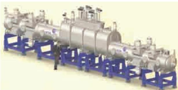
**Fig. 2:** WGTS magnet cryostat. The  $16 \text{ m}$  long cryostat is of an extremely complex technical structure and must meet strict technical requirements. The system has 12 cryogenic loops; six different fluids (He, Ne,  $N_2$ , Ar,  $T_2$ , and Kr) are used.
