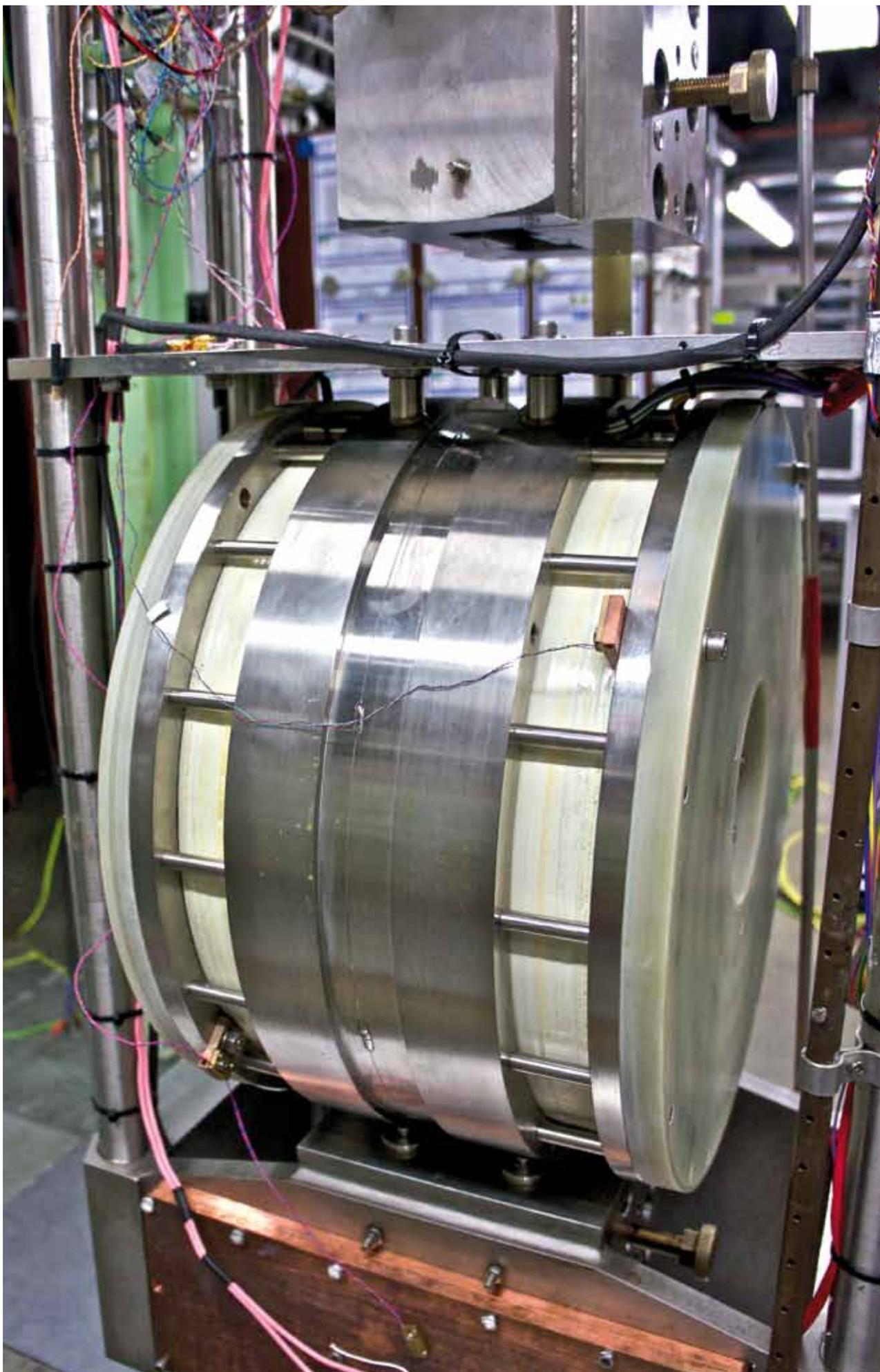
*New twelve-tesla magnet of the FBI facility to measure superconducting cables under realistic operation conditions.*
