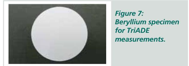
Figure 7: Beryllium specimen for TriADE measurements.
