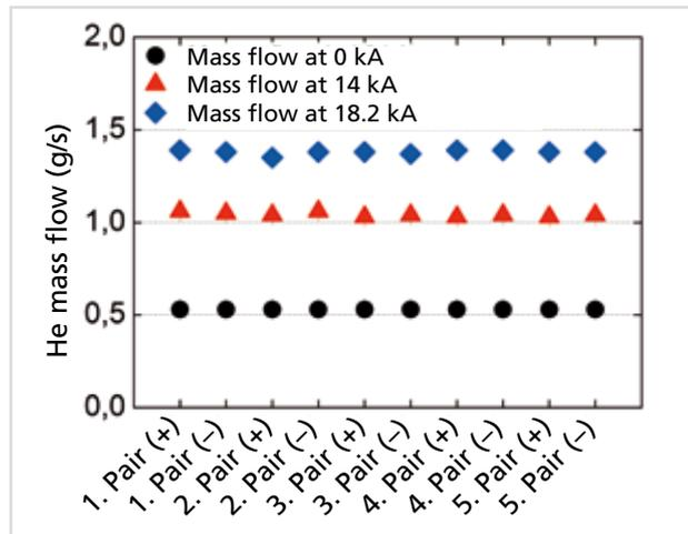
**Figure 14:** 50 K helium mass flows measured at 0.14 and 18.2 kA for five series current leads.
