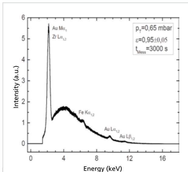
**Figure 9:** BIXS spectrum of a gaseous tritium source recorded by a silicon drift detector. A continuous bremsstrahlung spectrum is superposed by material-specific fluorescence lines.
