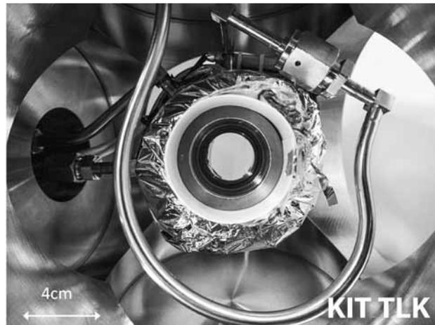
**Figure 7:** Cryogenic test cell of the TApIR experiment in the vacuum tank used for thermal insulation.
