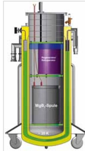
Figure 6: Cryostat with SMES ( $MgB_2$  coil) and regenerator/recuperator unit.
