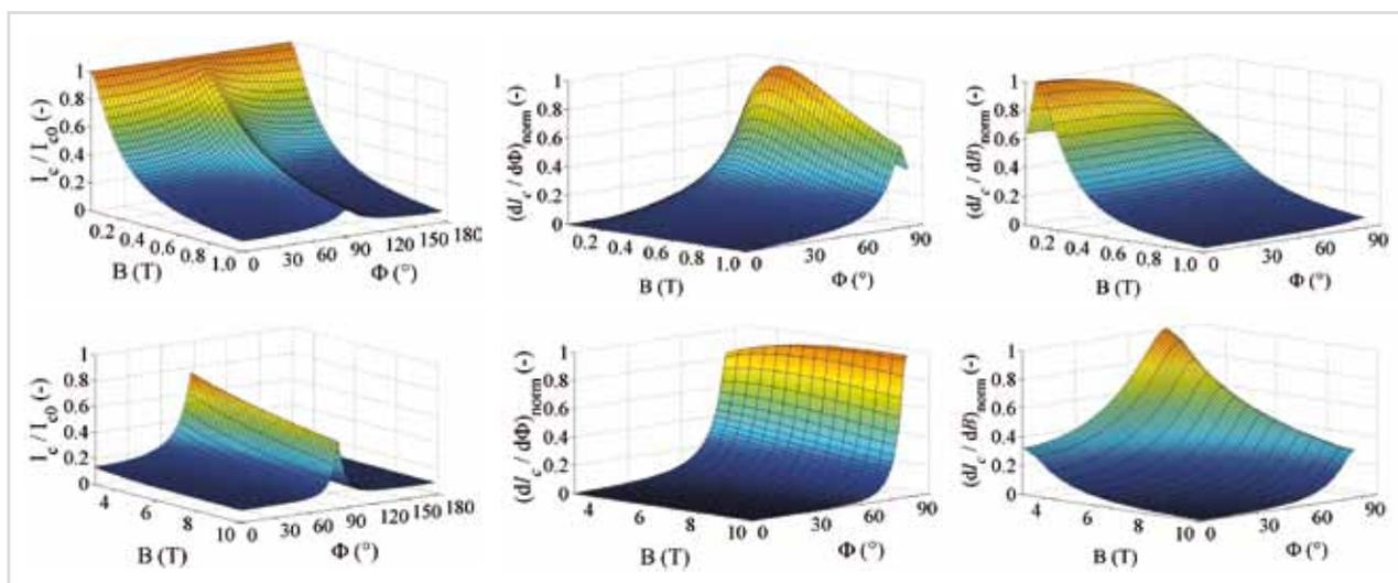
Figure 5: 3D fit (normalised) of the  $I_c(B, T, \Phi)$  data determined and partial derivation of the fit functions to the angle  $\Phi$  and magnetic field  $B$  for  $T = 77$  K (top) and  $T = 4.2$  K (bottom).
