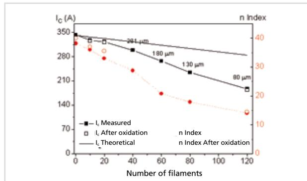
**Figure 1: Transport currents and  $n$  values of conductors with various numbers of filaments. The conductor remains indifferent in case of subsequent annealing in oxygen.**
