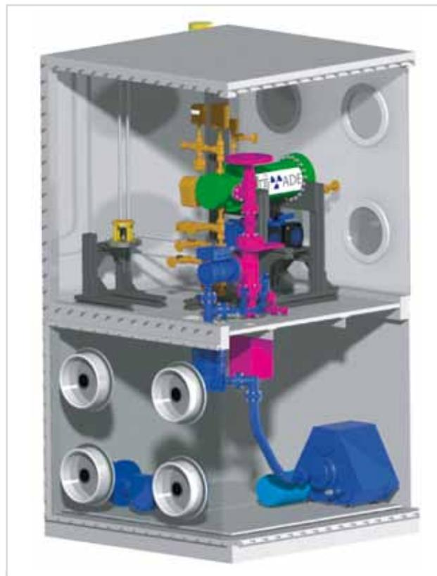
**Figure 10:** CAD of the TriADE experiment with the pumping station (coloured blue), core components (green), instruments and manual valves (brown), mass spectrometer and the corresponding volume (magenta), as well as the specimen holder (yellow).
