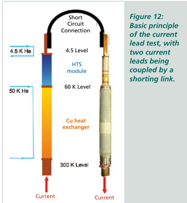
**Figure 12:** Basic principle of the current lead test, with two current leads being coupled by a shorting link.
