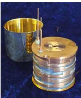
**Figure 7:** Magnet based on HTS tape conductors in five double pancake windings prior to the application of solder contacts with a central field of 5 T.
