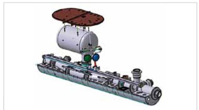
Figure 4: View into the CPS. The individual beam tube sections and the helium reservoir are visible. The protection diodes are planned to be installed below the tank (green, blue).
