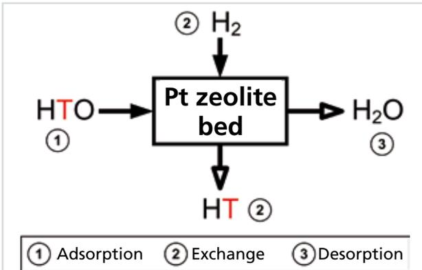
**Figure 3: Schematic representation of the capture & exchange method for processing highly tritiated water (HTO) and tritium recovery.**
