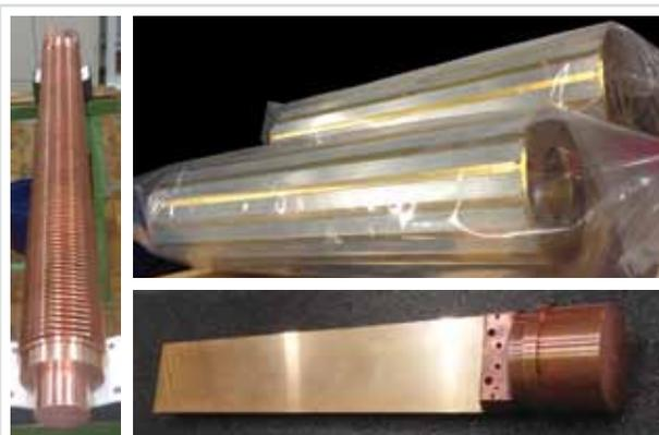
*Figure 1: Components for the 26 kA current lead.*
