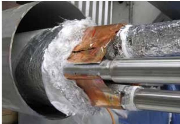
Figure 2: Cryo transfer line between the 2-kW facility and CuLTka.
