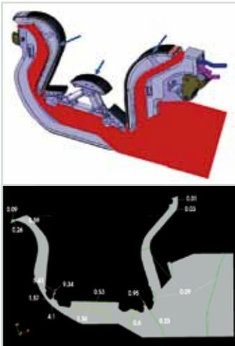
**Figure 5: Calculated pressure distribution (in Pa) below an ITER divertor cassette (top). The integral total pressure is 2.6 Pa in this example.**
