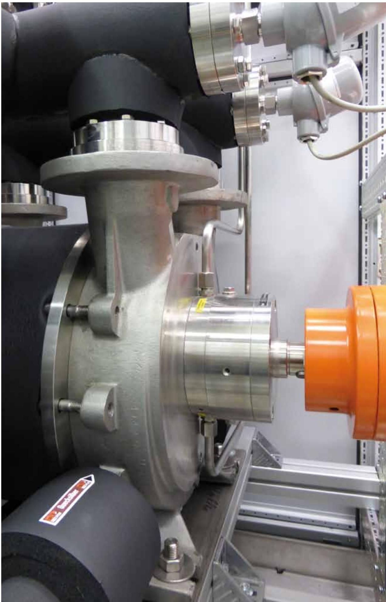
*The first mercury liquid ring vacuum pump operated worldwide.*
