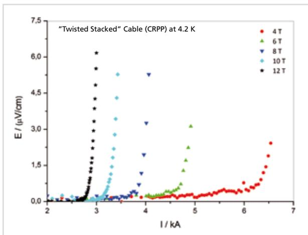
Figure 5: Measurement of critical current at variable magnetic fields and 4.2 K. The cable was supplied by CRPP (Switzerland).
