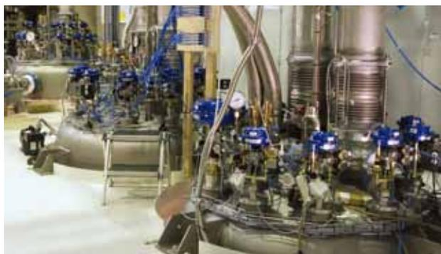
*Figure 3: Valve box (right), control cryostat (centre), and second valve box (rear left) in the CuLTka test facility.*
