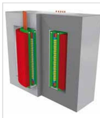
**Figure 8:** Sectional view of a superconducting transformer. The current-limiting superconducting winding is coloured yellow.
