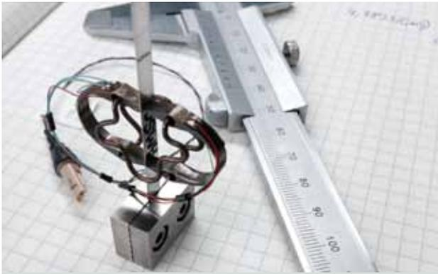
**Figure 8:** HTS wire prepared for a tensile test at room temperature and extensometer.
