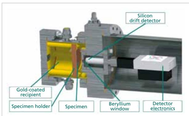
Figure 6: CAD drawing of the main components of TriADE.
