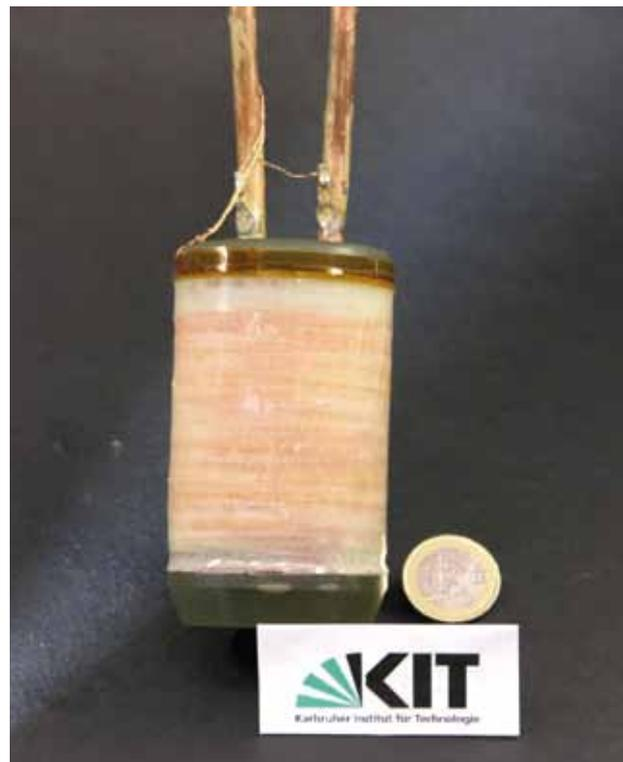
**Figure 8:** 1 T REBCO mini solenoid for the HOMER I-20 T configuration.
