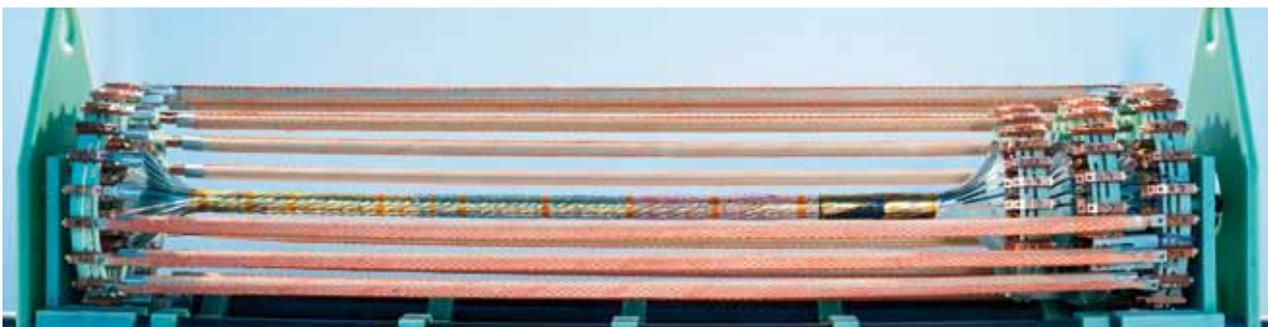
Figure 15: Two cable designs with current-carrying capacities of the individual phases of 50 % (left) and 90 % (right) and a current-carrying capacity adjusted to phase 1 (left) or phase 2 (right) of the real cable.
