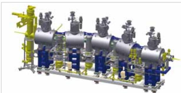
Figure 3: New concept of the differential pumping section of KATRIN. The five superconducting magnets and the five pumping chambers can be seen.
