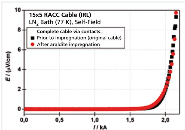
Figure 4: Critical current of an HTS tape prior to and after impregnation with araldite / quartz sand (1:1).
