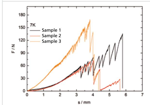
**Figure 10:** Mechanical behaviour under tensile loading at room temperature and 7 K (samples 1 and 2: Para-aramide thread and sample 3: Para-aramide twaron thread).
