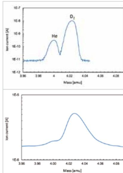
**Figure 6: Resolution of He and D<sub>2</sub> in a gas mixture with 3.7% He and 95.4% D<sub>2</sub>. The top diagram shows the reference measured with a high-end quadrupole, the bottom diagram represents the best result obtained with the new ART-MS.**
