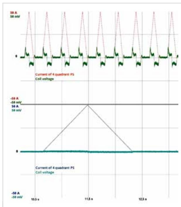
**Figure 2: Behaviour of the MgB<sub>2</sub> test coil during a triangular charge and discharge cycle at frequencies of 0.3 Hz (top) and 3 Hz (bottom), respectively.**
