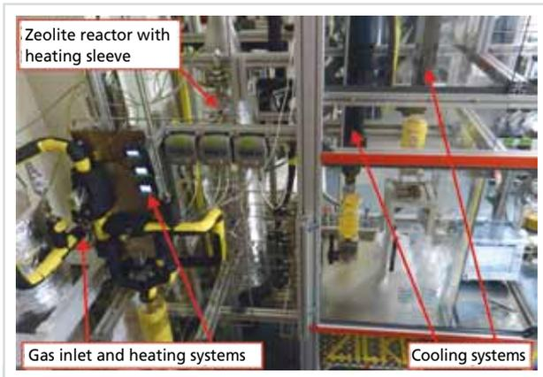
**Figure 4: The Zicke experiment – test set-up for studying the C&E method under ITER-relevant technical conditions.**
