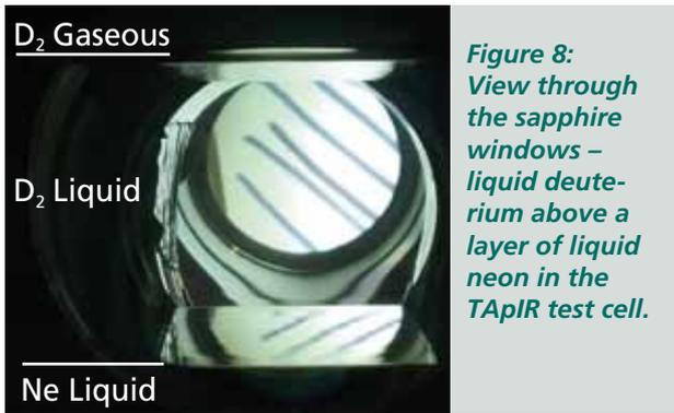
**Figure 8:** View through the sapphire windows – liquid deuterium above a layer of liquid neon in the TApIR test cell.
