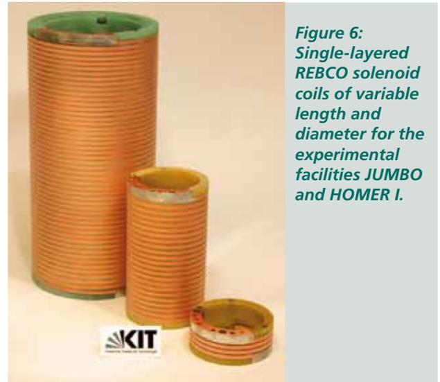
Figure 6: Single-layered REBCO solenoid coils of variable length and diameter for the experimental facilities JUMBO and HOMER I.
