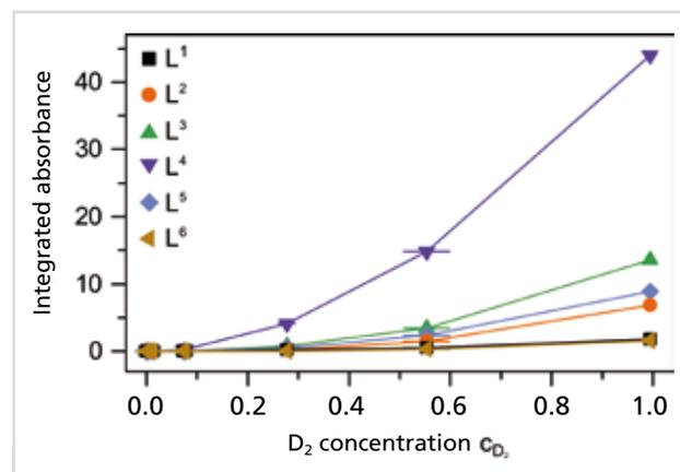
**Figure 10:** Integrated absorbance of the lines L<sub>1</sub> to L<sub>6</sub> in the second D<sub>2</sub> vibration band as a function of D<sub>2</sub> concentration.
