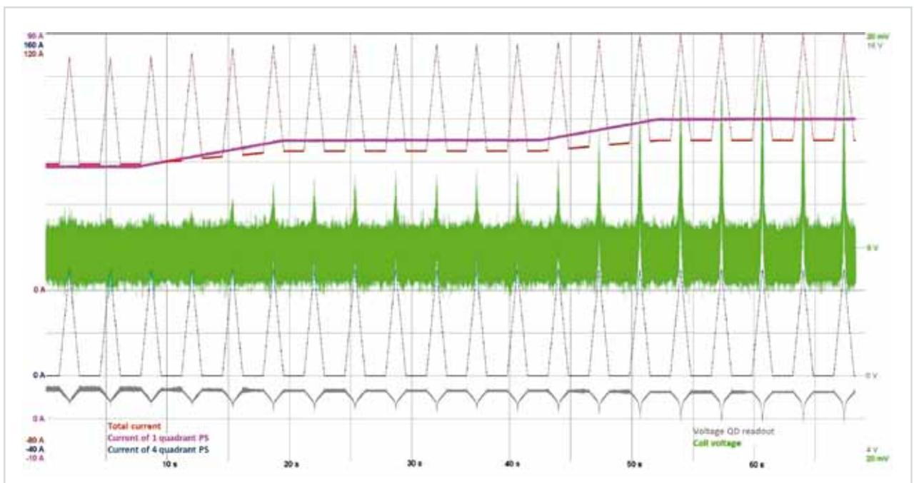
Figure 7: Behaviour of the REBCO solenoid coil at 77 K under triangular current loading in the range from 110 A to 120 A.
