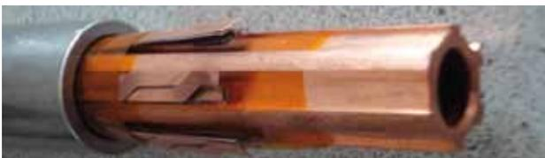
**Figure 3: Rutherford cable concept with six Roebel strands in hexagonal geometry and a cladding tube for mechanical stabilisation.**
