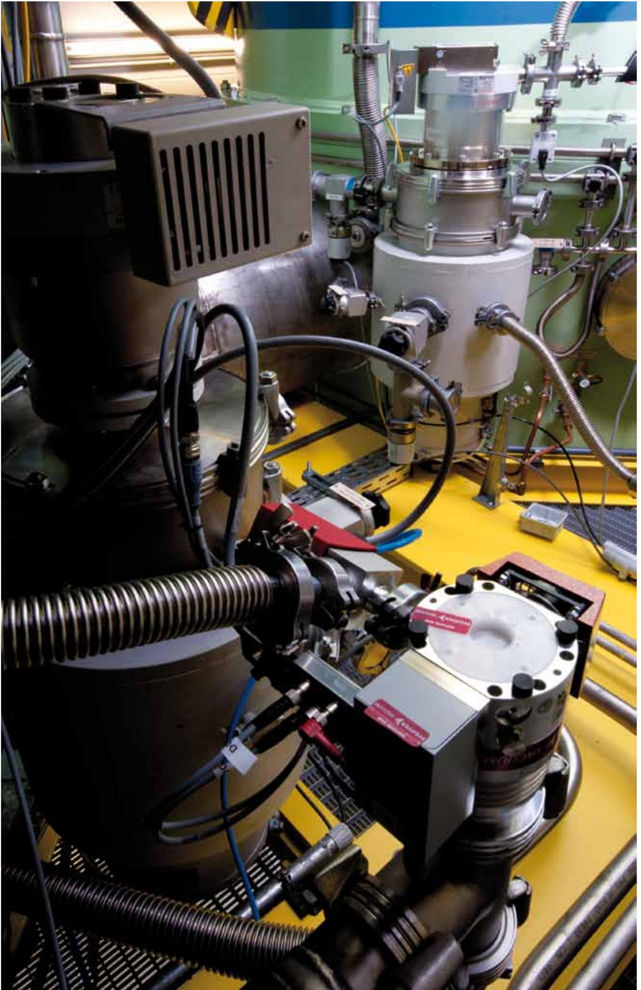
*Turbomolecular pump of the 2-kW helium refrigerator.*
