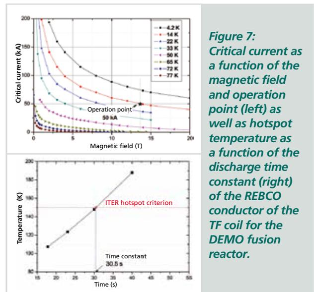
Figure 7: Critical current as a function of the magnetic field and operation point (left) as well as hotspot temperature as a function of the discharge time constant (right) of the REBCO conductor of the TF coil for the DEMO fusion reactor.
