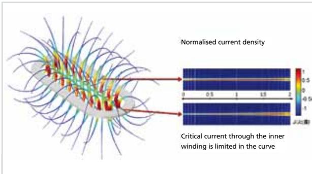
**Figure 6:** Calculated field distribution in a racetrack coil.
