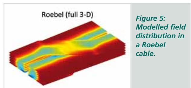
**Figure 5: Modelled field distribution in a Roebel cable.**
