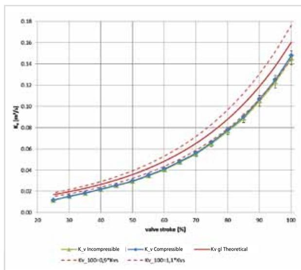
Figure 4: Operation characteristics of cryovalves.
