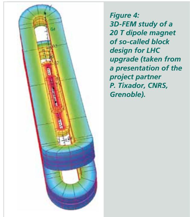
Figure 4: 3D-FEM study of a 20 T dipole magnet of so-called block design for LHC upgrade (taken from a presentation of the project partner P. Tixador, CNRS, Grenoble).
