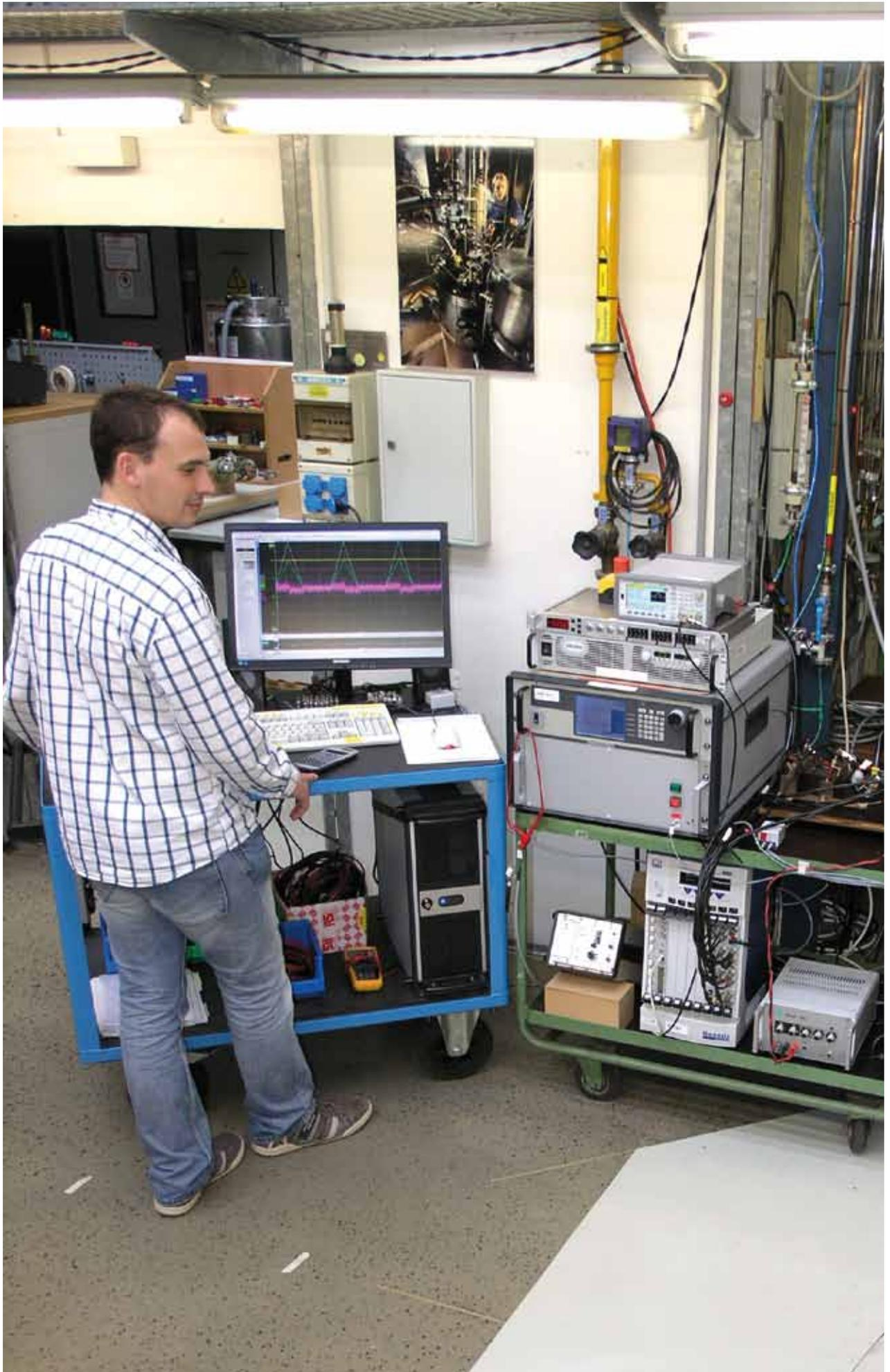
*Set-up and commissioning of the magnetic current supply unit with integrated quench protection for a superconducting energy storage system under the EWI-LIQHYSMES project.*
