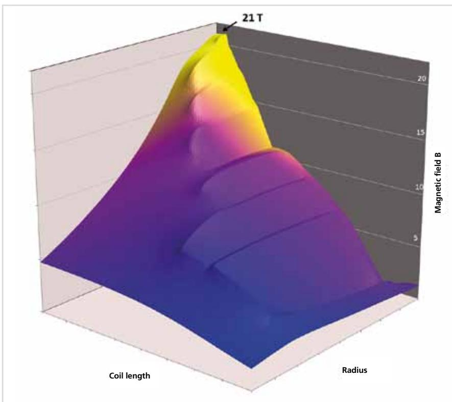
**Figure 9:** Magnetic field distribution of the complete magnet system with  $B_{0, \max} = 21$  T, consisting of 3 NbTi and 3  $(\text{NbX})_3\text{Sn}$  coils of the HOMER I facility ( $B_0 = 20$  T) plus one REBCO mini solenoid coil ( $B_0 = 1$  T).
