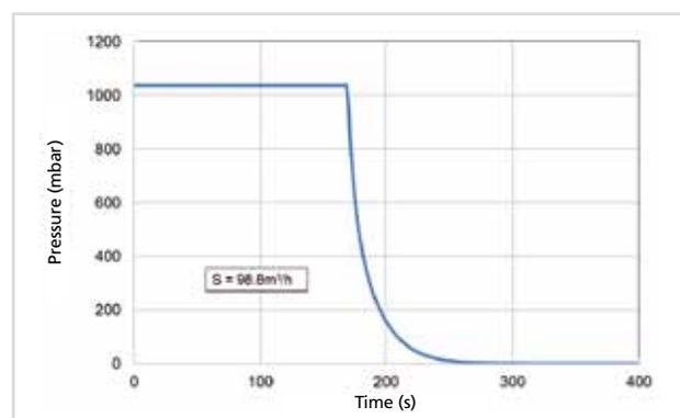
**Figure 8:** First pumping curve of a mercury ring pump: The 450 l dosage dome of the THESEUS facility was evacuated to an end pressure of a few mbar within 90 seconds at a pumping speed of nearly 100 m<sup>3</sup>/h.
