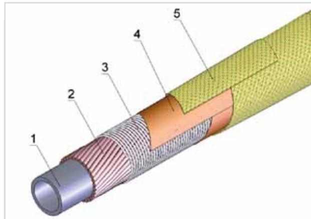
**Figure 9:** Nuclotron cable: 1 CuNi pipe, 2 SC wire, 3 NiCr wire (possibly carbon / Kevlar thread), 4 Kapton, 5 glass fibres.
