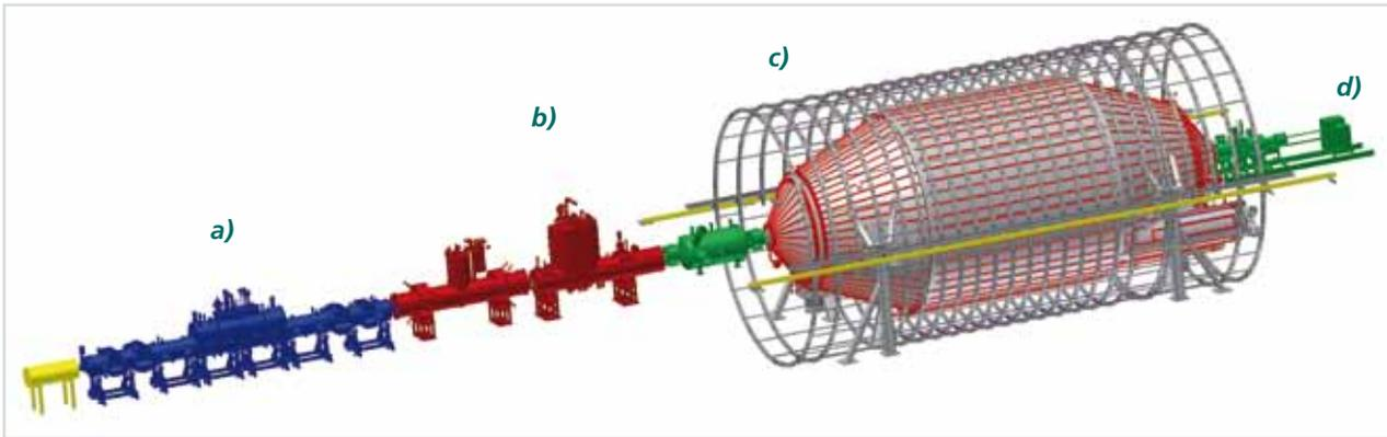
**Figure 1:** Schematic representation of the KATRIN international large-scale experiment. The electrons produced by  $\beta$ -decays in a high-intensity windowless molecular tritium source (WGTS, [a]) are passed through a tritium pumping station with the active and passive elements DPS2 and CPS (b) to a system (c) consisting of two electrostatic spectrometers (pre spectrometer and main spectrometer). The analysed electrons are counted by a semiconductor detector (d).
