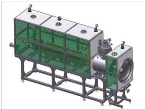
Figure 5: Design of the rear section of KATRIN.
