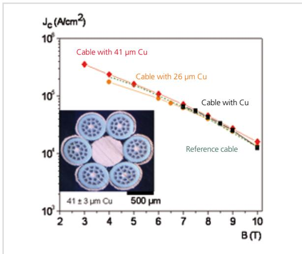
**Figure 2: Stranded magnesium diboride AC cable cross-section with central Cu stabilisation and Cu plating for improved coupling and behaviour of the transport currents.**
