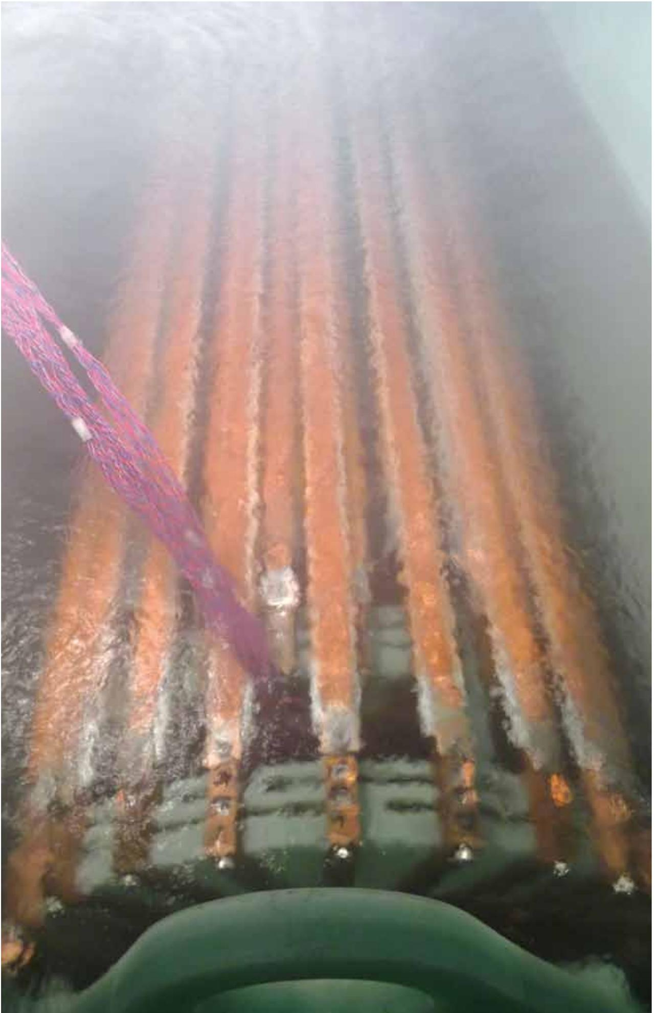
*Model of the power cable in the liquid nitrogen bath.*
