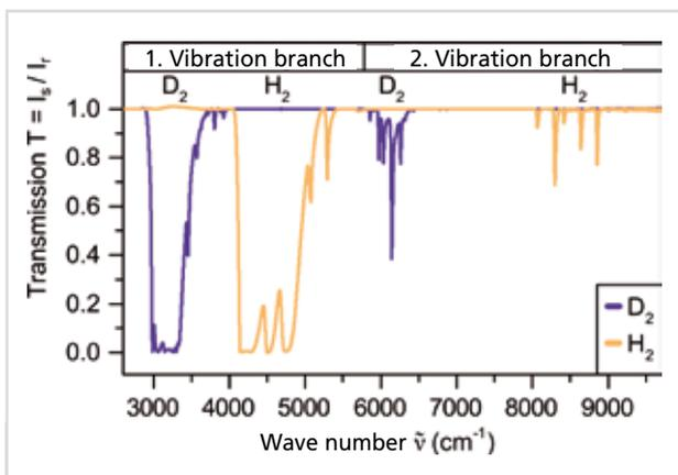
**Figure 9:** Transmission spectrum of liquid hydrogen (H<sub>2</sub>, purity 6.0; yellow) and deuterium (D<sub>2</sub>, purity 2.4 + remainder HD; magenta) measured in TApIR.
