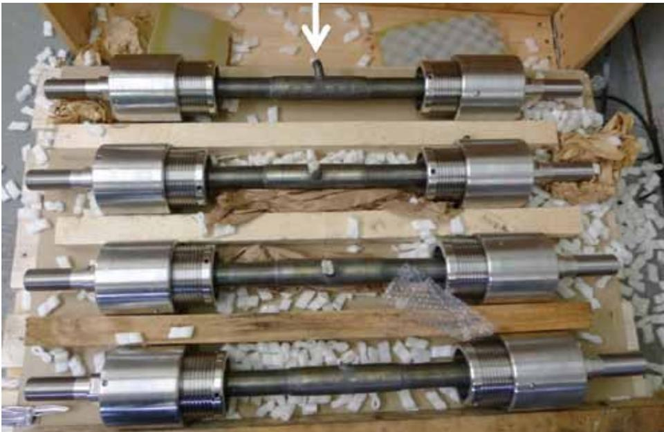
**Figure 11:** Four European prototypes of helium inlets for the ITER TF coils with a length of about 1.2 m each. On both sides, the clamps to mount the components in the test facility are visible. In the centre (see arrow), the welded pipe section for the helium inlet is located.
