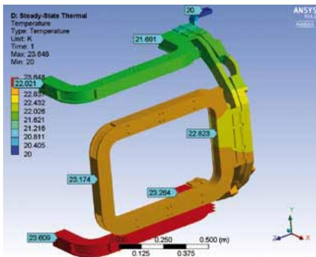
Figure 5: Temperature distribution of the superconducting coils on a copper ring for the demonstrator with four coils.
