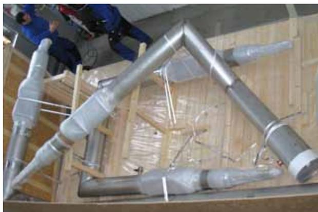
Figure 3: Cryo transfer line sections for CuLTka.
