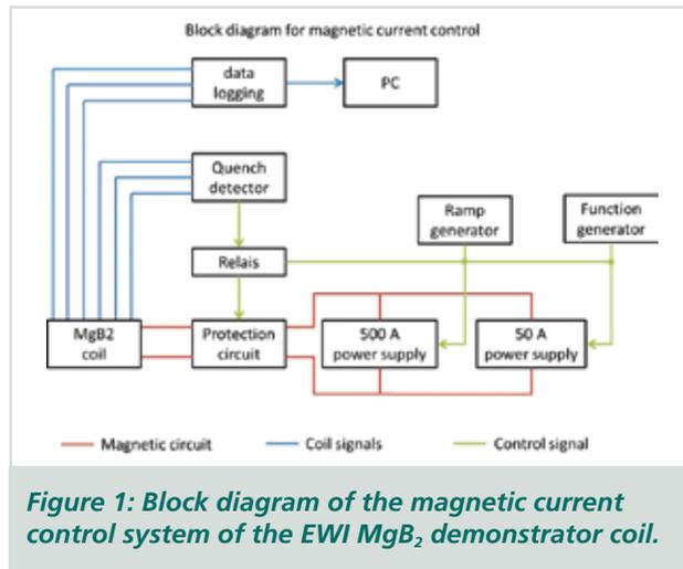
**Figure 1: Block diagram of the magnetic current control system of the EWI MgB<sub>2</sub> demonstrator coil.**
