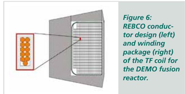
Figure 6: REBCO conductor design (left) and winding package (right) of the TF coil for the DEMO fusion reactor.
